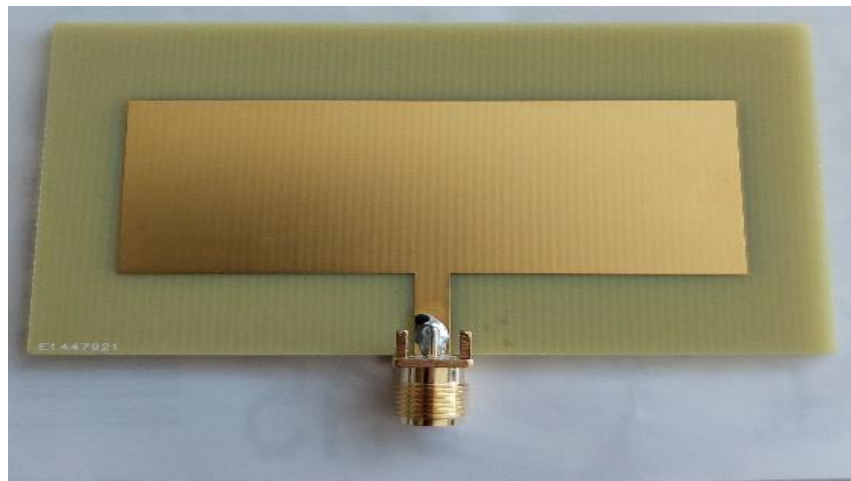
Figure 4.1.1 Fabricated antenna with SMA connector
