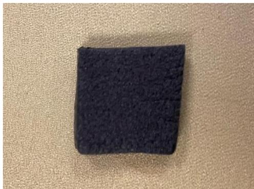
Figura 55: Campione Stokvis GY 14,53x14,33x3,67 mm
