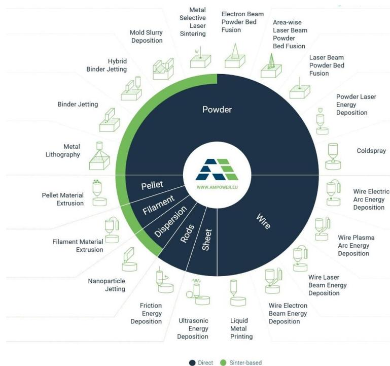
Figure 1: Classification of Metal AM Technologies [10]
