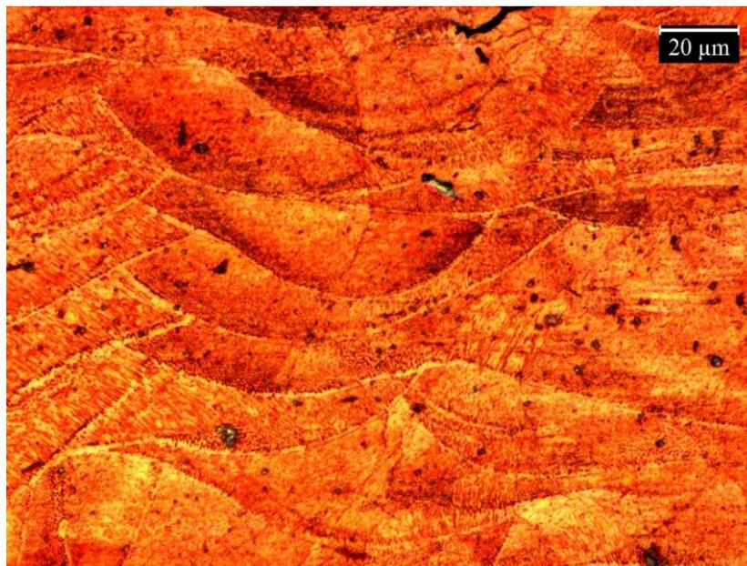
Figure 49: Melt-pool visualization (Magnification: 500X)
