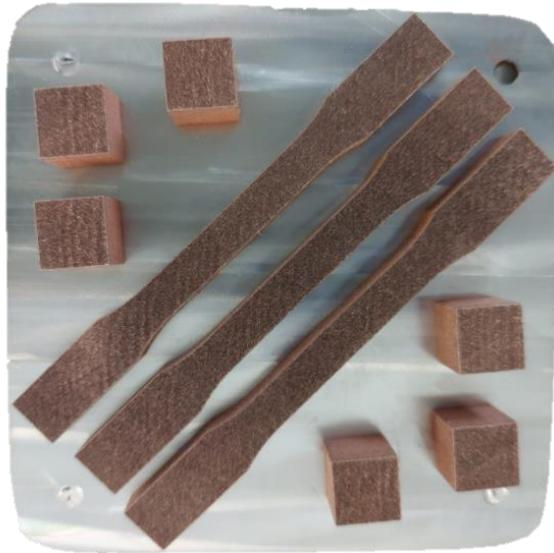
Figure 15: Job 3 printed samples with dog-bone tensile samples
