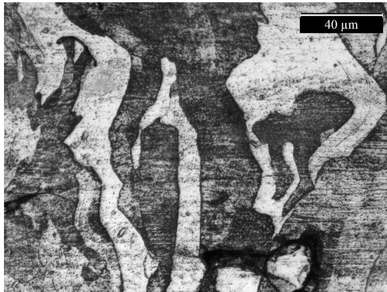
Figure 51: Columnar grain structure (Magnification: 500X)
