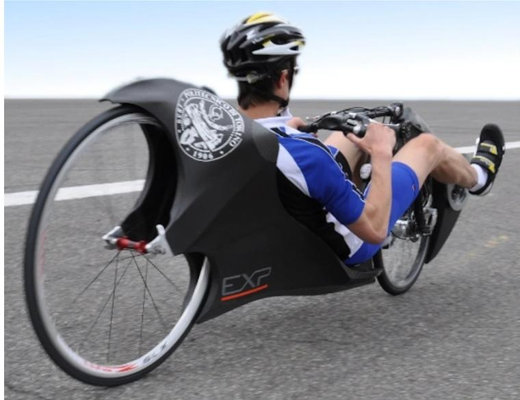
Figure I.2.1: Team Policumbent's first prototype, C.O.R.A. (Cycling Optimized Recumbent Aeroshape)
