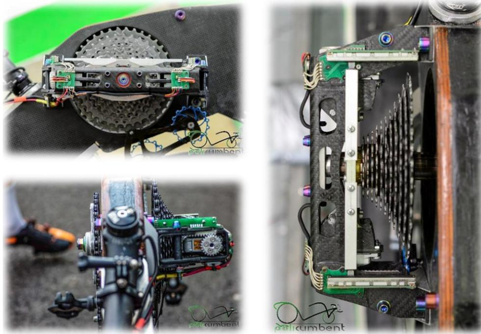
Figure I.2.10: Prototype Taurus's patented gear shifting system
