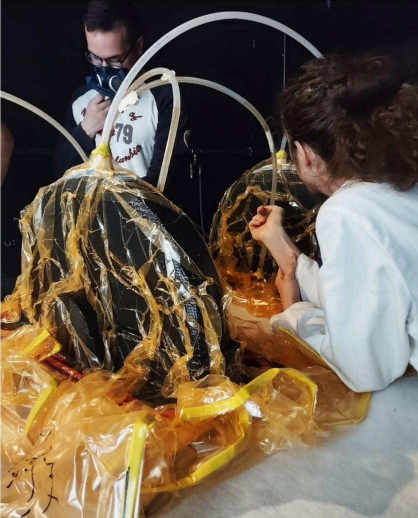
Figure III.2.6: Wheel covers during the infusion procedure
