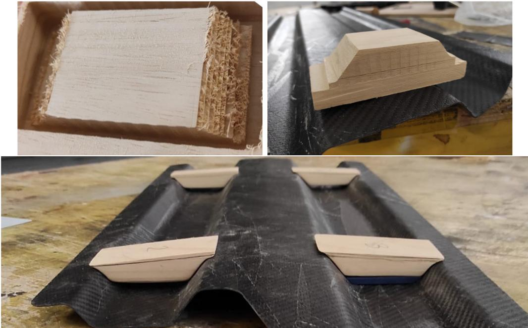
Figure III.2.12: Wood machined parts: after raw machining on top left, after sanding on top right and set in place for fit check on bottom
