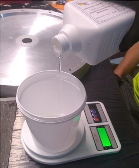
Figure III.2.5: Hand lamination: preparing the matrix by combining the resin with its catalyst
