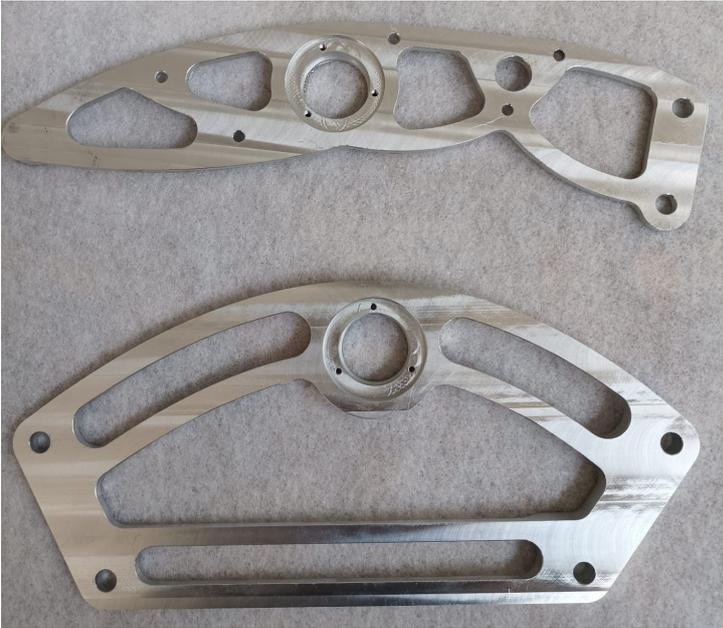
Figure II.3.3: Aluminum plates used to support the grooved shaft of the moving cassette system
