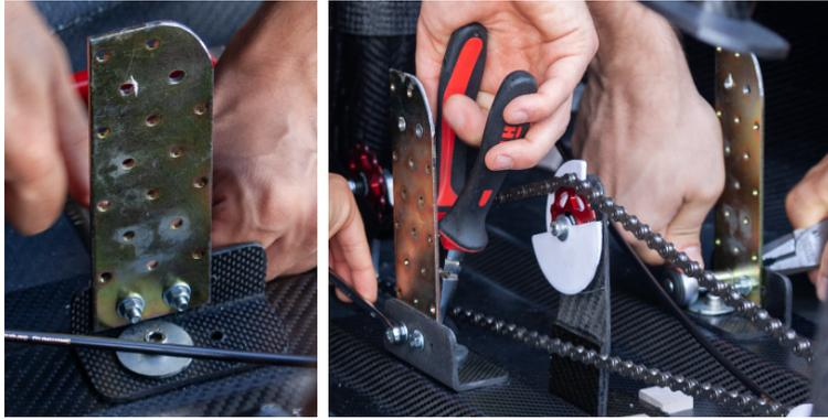
Figure II.9.3: Adjustable seat: plates set in place on the bottom longerons reinforced rear section
