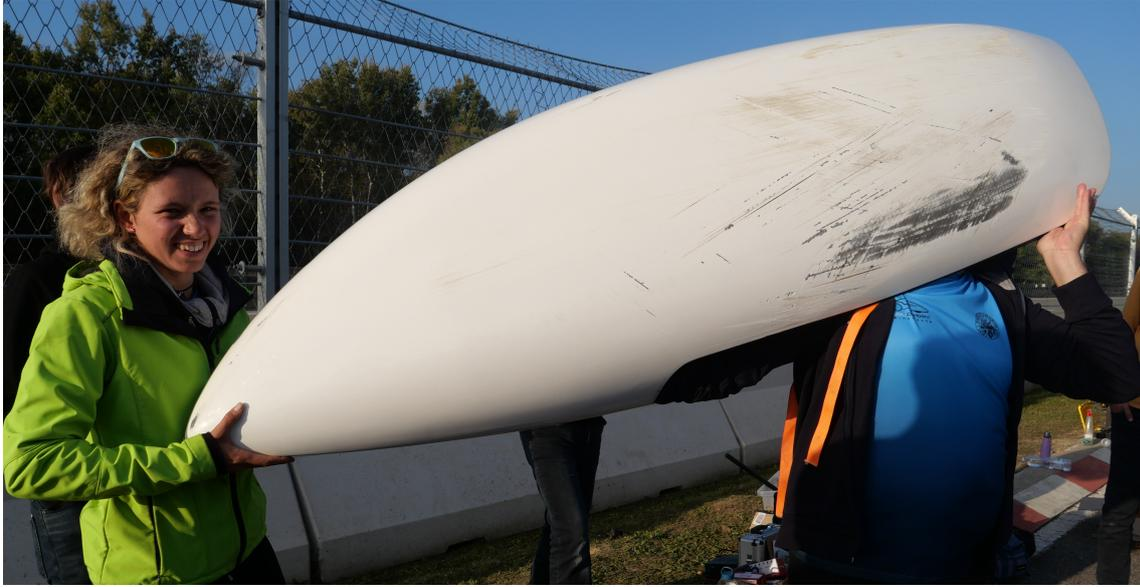
Figure I.2.11: Vittoria Spada, rider of Taurus X, standing unharmed with the prototype's fairing in her hand after a crash at 70 km/h
