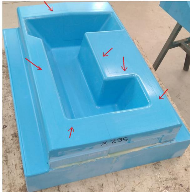
Figure III.2.2: Piece's outlines on the basin's mold
