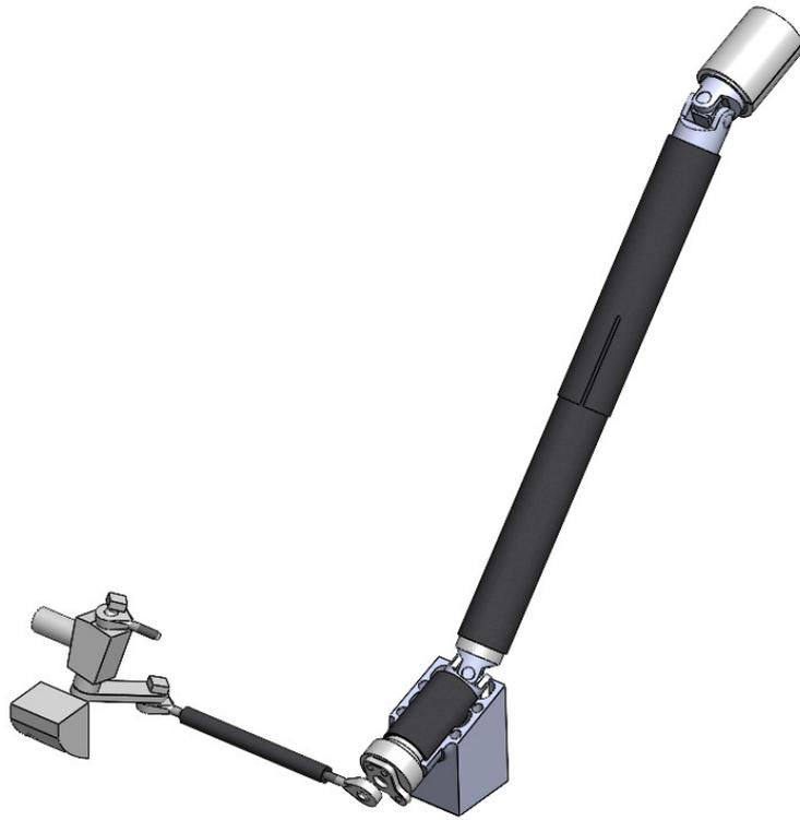
Figure II.3.8: Carbon tubes were used for the steering mechanism too, both for the main column and for the tie-rods
