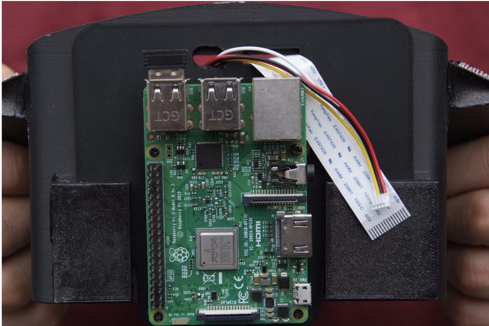
Figure II.4.12: Rear view of the cameras' assembly: the lid is set in place thanks to the 2 lateral lamellas, similarly to a frame for photographs
