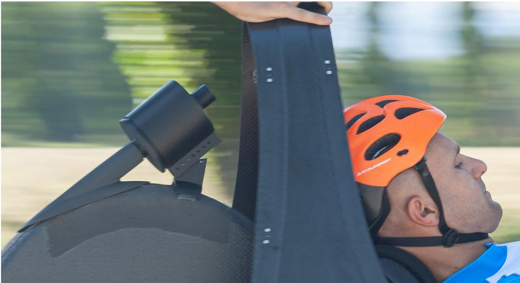
Figure II.9.8: Air filter connection on the wheel cover
