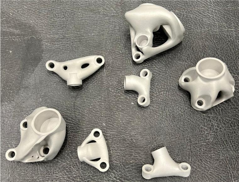
Figure II.3.2: Optimized 3D printed parts used for the transmission’s supports structure
