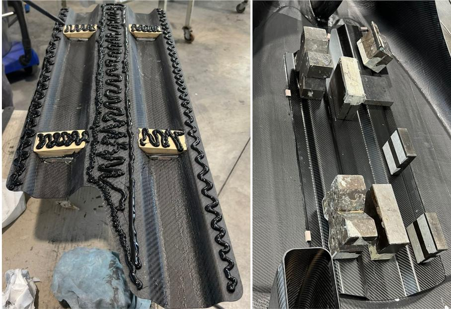
Figure III.2.10: Glue spilling and weight application on the bottom longerons
