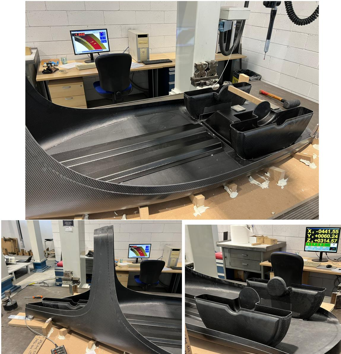
Figure III.2.9: Tolerance checks on the fairing
