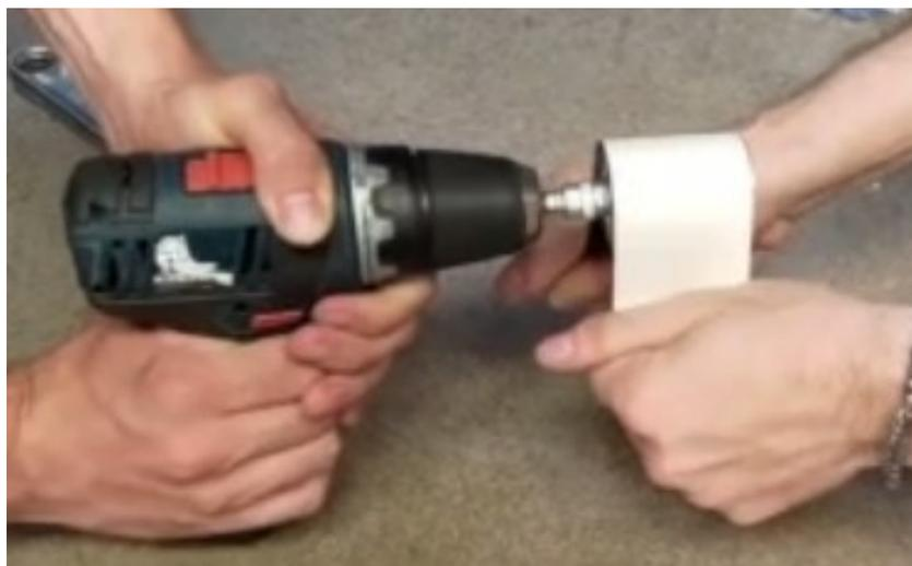
Figure III.2.14: Sanding a piece fit onto the screw
