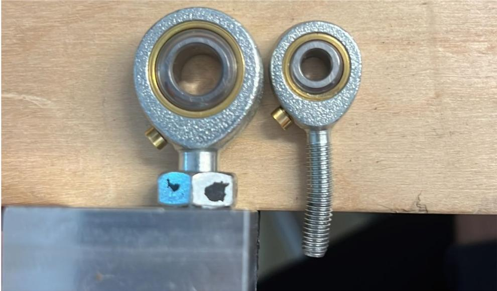
Figure II.7.4: On the right: one of the M5 bent rod-end bearings. On the left: one of the replacement M8 parts used in their stead after a basic dimensioning
