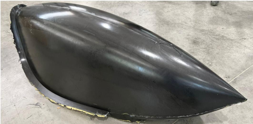
Figure III.2.7: Raw front fairing just extracted from the mold. Window and flange cuts needed
