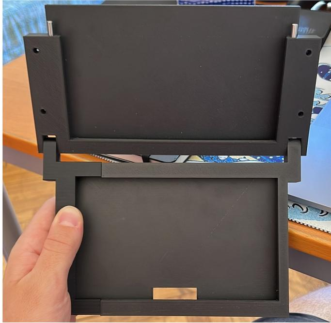
Figure II.4.15: Partially mounted frames for the screens
