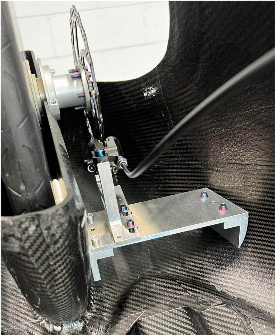
Figure II.8.5: Braking system in place on Cerberus
