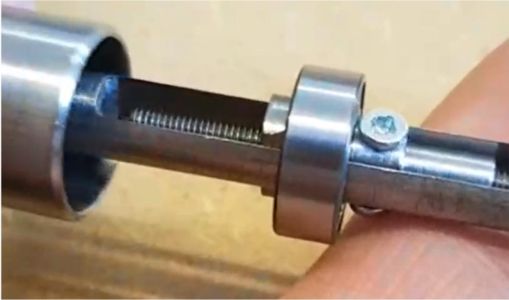
Figure II.5.7: Inner ring of bearing  $\varnothing 7\text{-}\varnothing 14 \times 5$  locked in place
