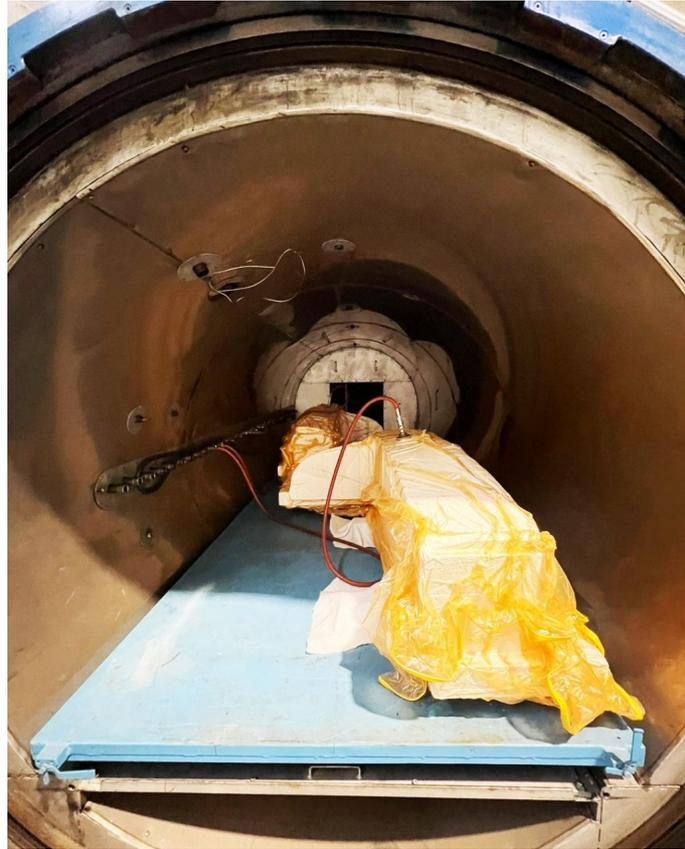
Figure III.2.4: Structural fairing mold (carbon prepreg) in the autoclave
