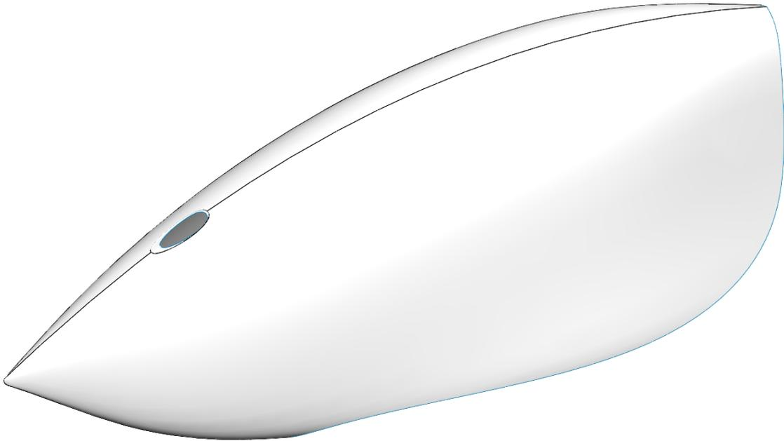
Figure II.2.3: CAD image of the surface used for the front fairing's molds generation
