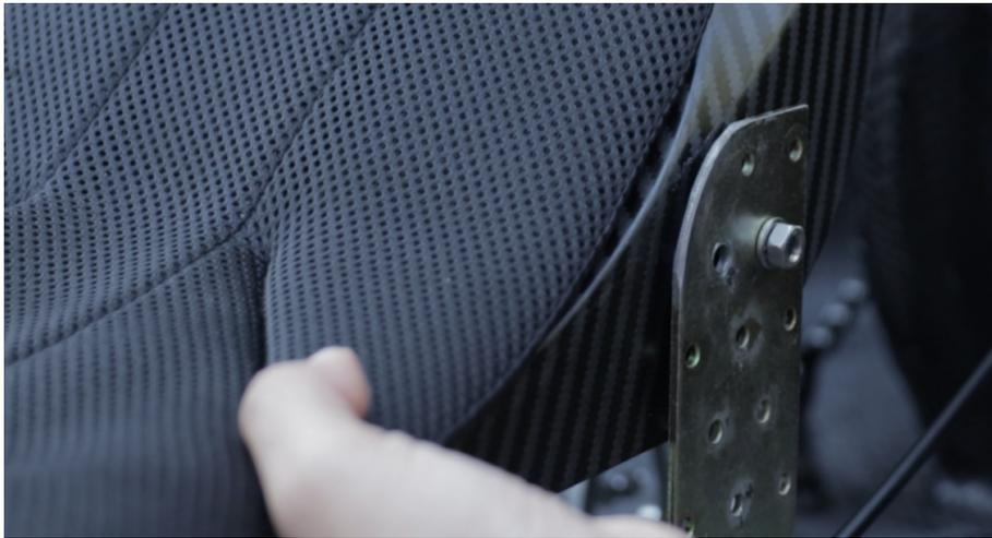
Figure II.9.4: Adjustable seat, rear locking system, upper part: depending on the hole used, the seat moves up and down and is reclined
