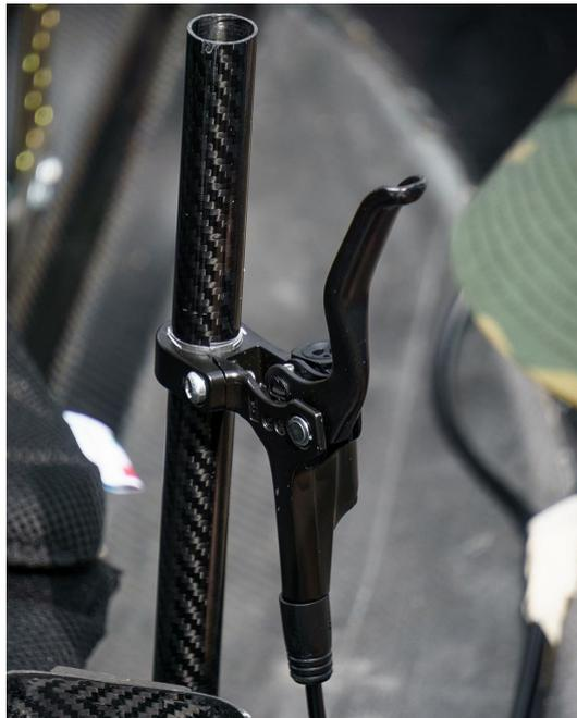
Figure II.3.5: Carbon tube used as a support for the brake lever
