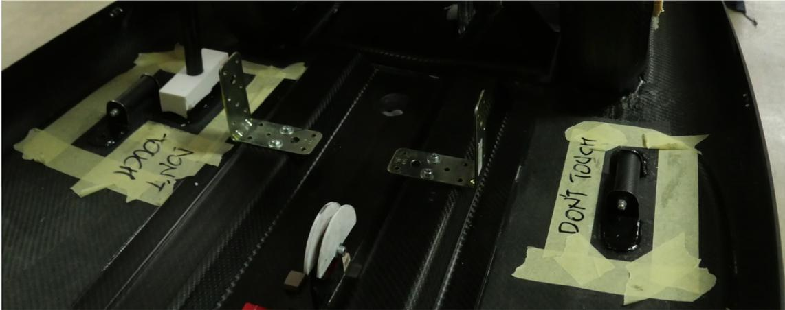
Figure II.9.6: Anchoring points for the seatbelt being glued onto the fairing
