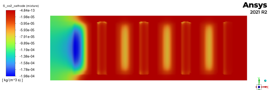
Figure 6.9: Carbon Dioxide CO 2 Sink Term, active at the Cathode
