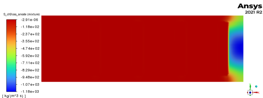
Figure 6.7: Acetate \text{CH}_3\text{COO}^- Sink Term, active at the Anode
