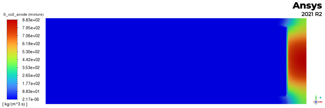
Figure 6.8: Carbon Dioxide CO 2 Sink Term, active at the Anode
