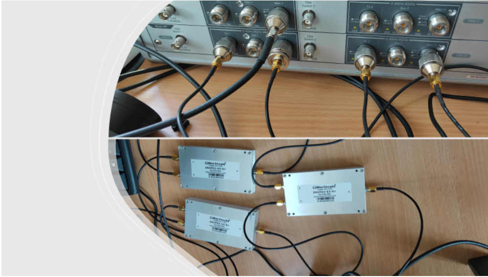
Figure 3.21: MT8000A connection with the device in 4x4 MIMO mode (real picture of the platform)
