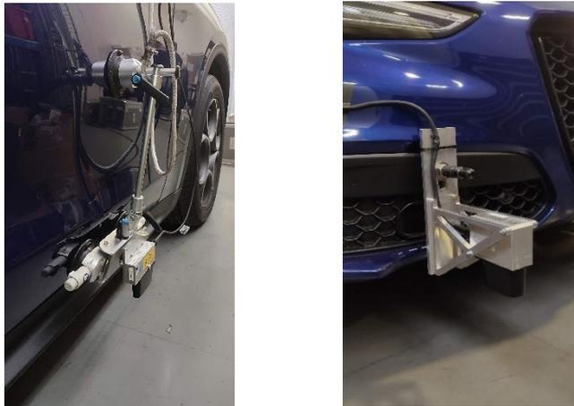
*Figure 36: Optical sensors for vehicle height (left) and side slip angle (right)*
