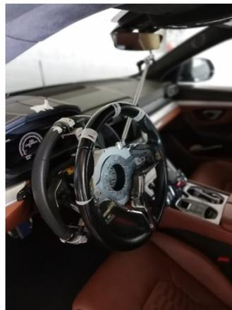
*Figure 37: Steering torque sensor*
