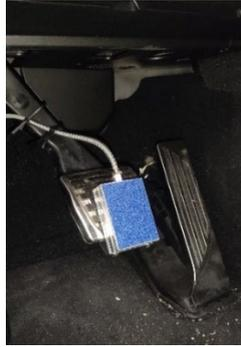
*Figure 38: Load cell on brake pedal*
