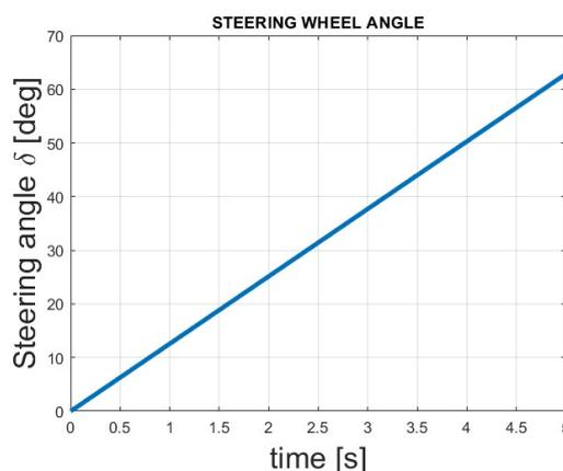
Figure 19: Steering angle during Ramp steer manoeuvre
