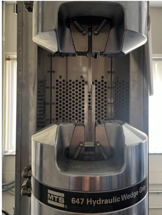
Figure 2.9: Double Lap Joint placed in the MTS Testing System
