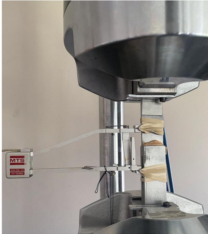
Figure 5.36: DLJ placed on the MTS machine with an extensometer
