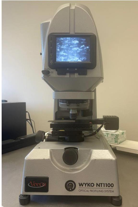
Figure 2.4: WYKO NT1100 surface profiler
