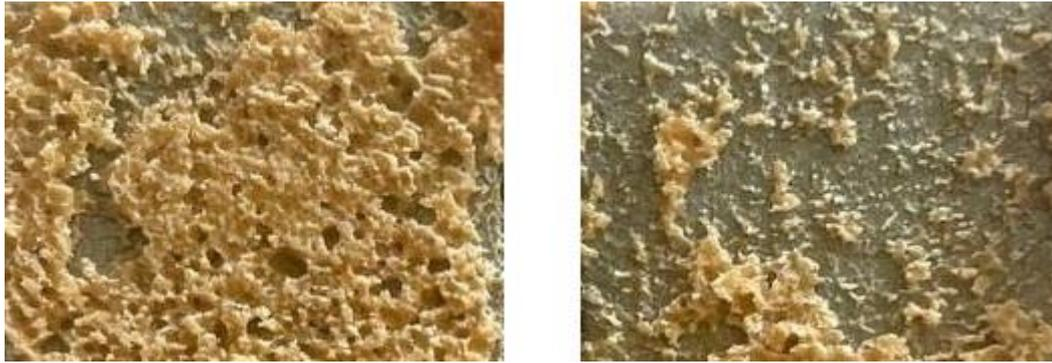
Figure 5.29: Fracture surface of DLJs cured in autoclave
