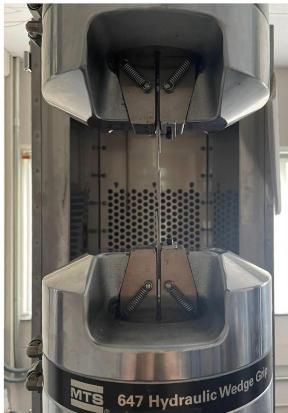
Figure 2.6: MTS Fatigue Testing System for SLJs
