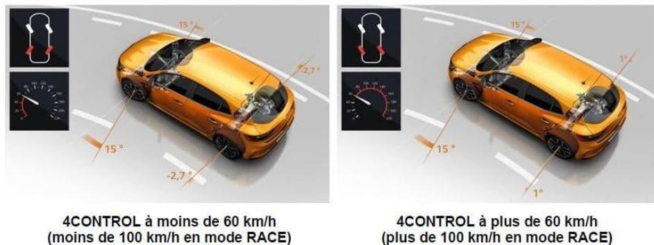
**Figure 2.7** Scheme of Renault 4Control [19].
