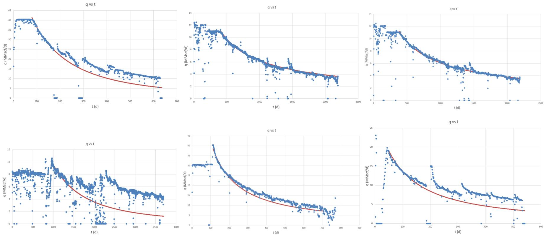
Figure A-4. Decline curve fit for the wells #29 (upper left), #30 (upper middle), #31 (upper right), #32 (bottom left), #33 (bottom middle), #34 (bottom right).
