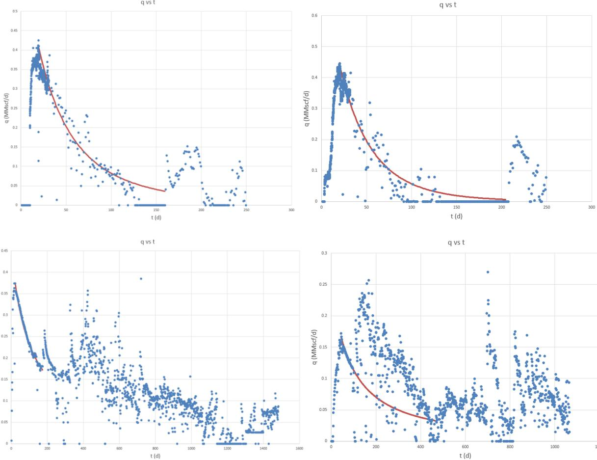
Figure A-1. Decline curve fit for the wells #2 (upper left), #3 (upper right), #4 (bottom left), #5 (bottom right).
