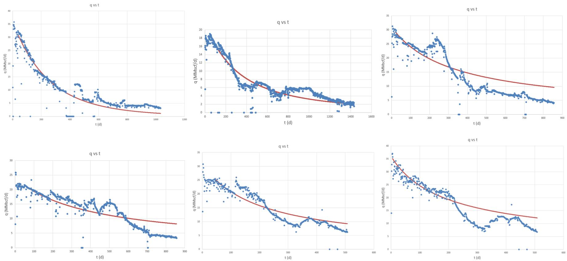
Figure A-9. Decline curve fit for the wells #71 (upper left), #72 (upper middle), #73 (upper right), #74 (bottom left), #75 (bottom middle), #76 (bottom right).
