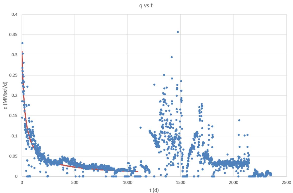
Figure 24. Well #1 production rate versus time plot with decline curve fit.
