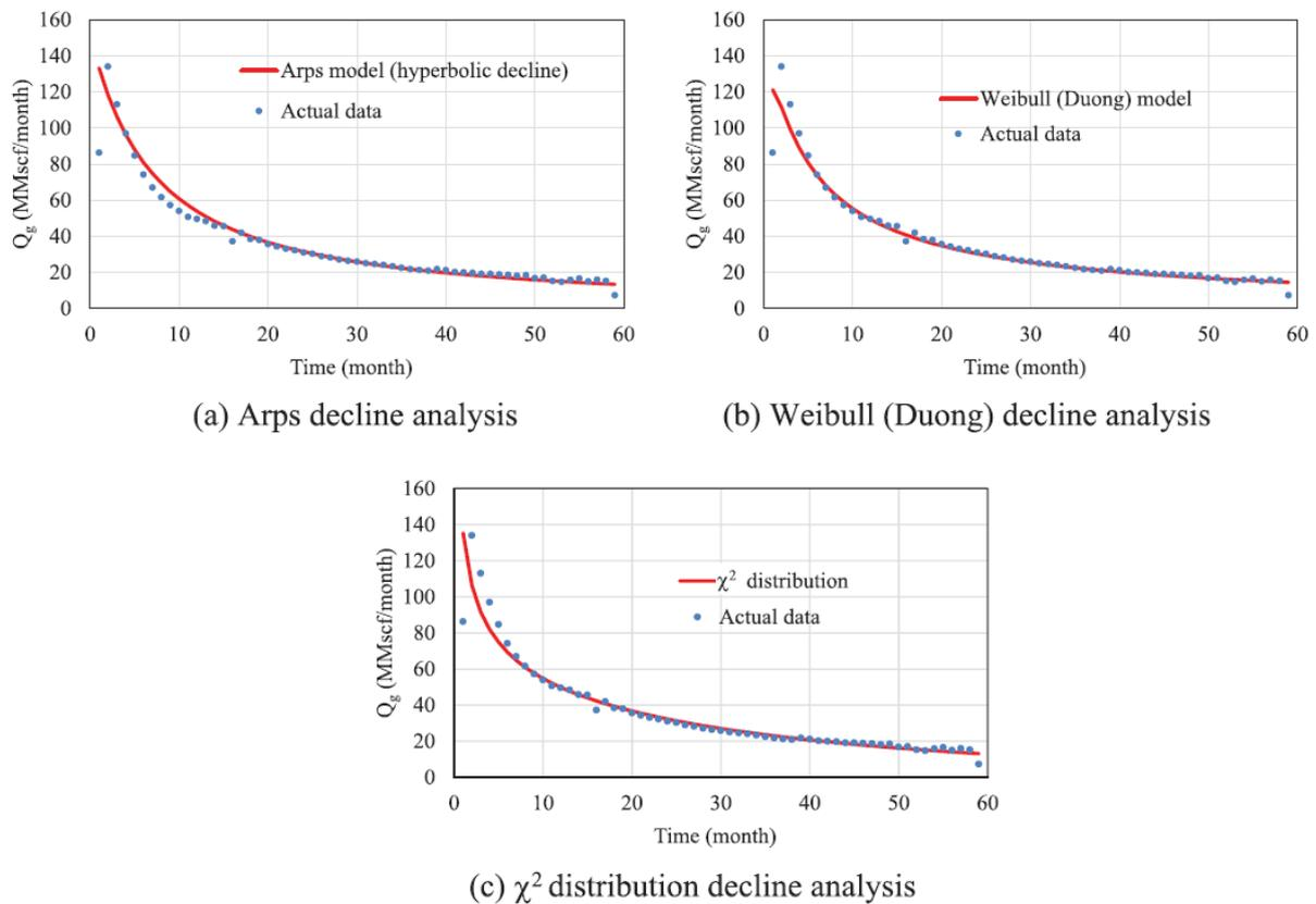
Figure 10. DCA using different types of decline curve models. (Y. Yuan et al., 2020)
