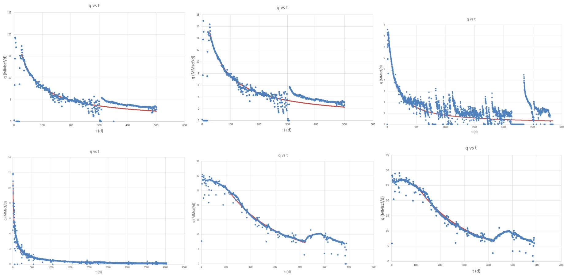
Figure A-7. Decline curve fit for the wells #47 (upper left), #48 (upper middle), #49 (upper right), #62 (bottom left), #63 (bottom middle), #64 (bottom right).
