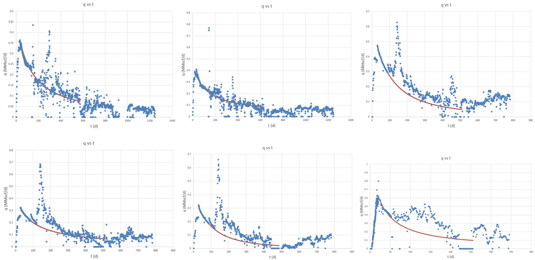
Figure A-2. Decline curve fit for the wells #6 (upper left), #7 (upper middle), #8 (upper right), #9 (bottom left), #10 (bottom middle), #11 (bottom right).
