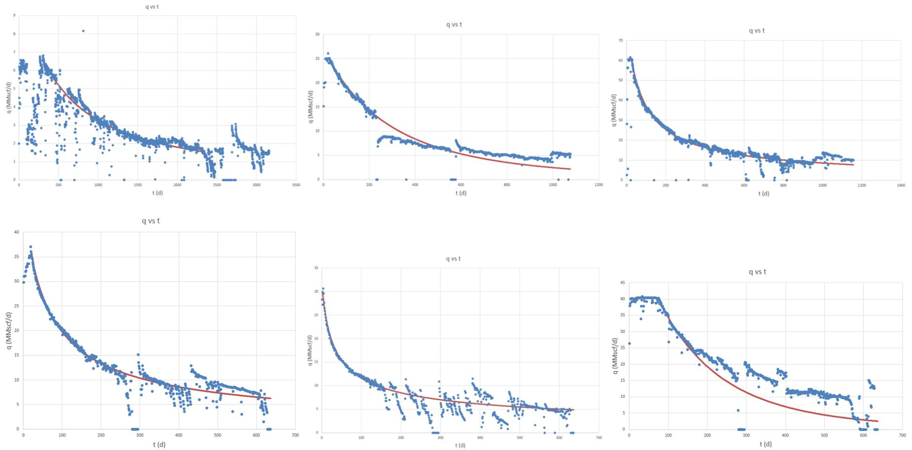
Figure A-3. Decline curve fit for the wells #23 (upper left), #24 (upper middle), #25 (upper right), #26 (bottom left), #27 (bottom middle), #28 (bottom right).
