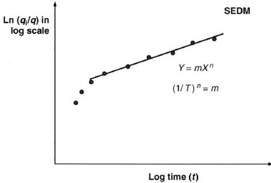
Figure 11. Plot of SEDM/SEPD model. (A. Satter & G. M. Iqbal, 2015)
