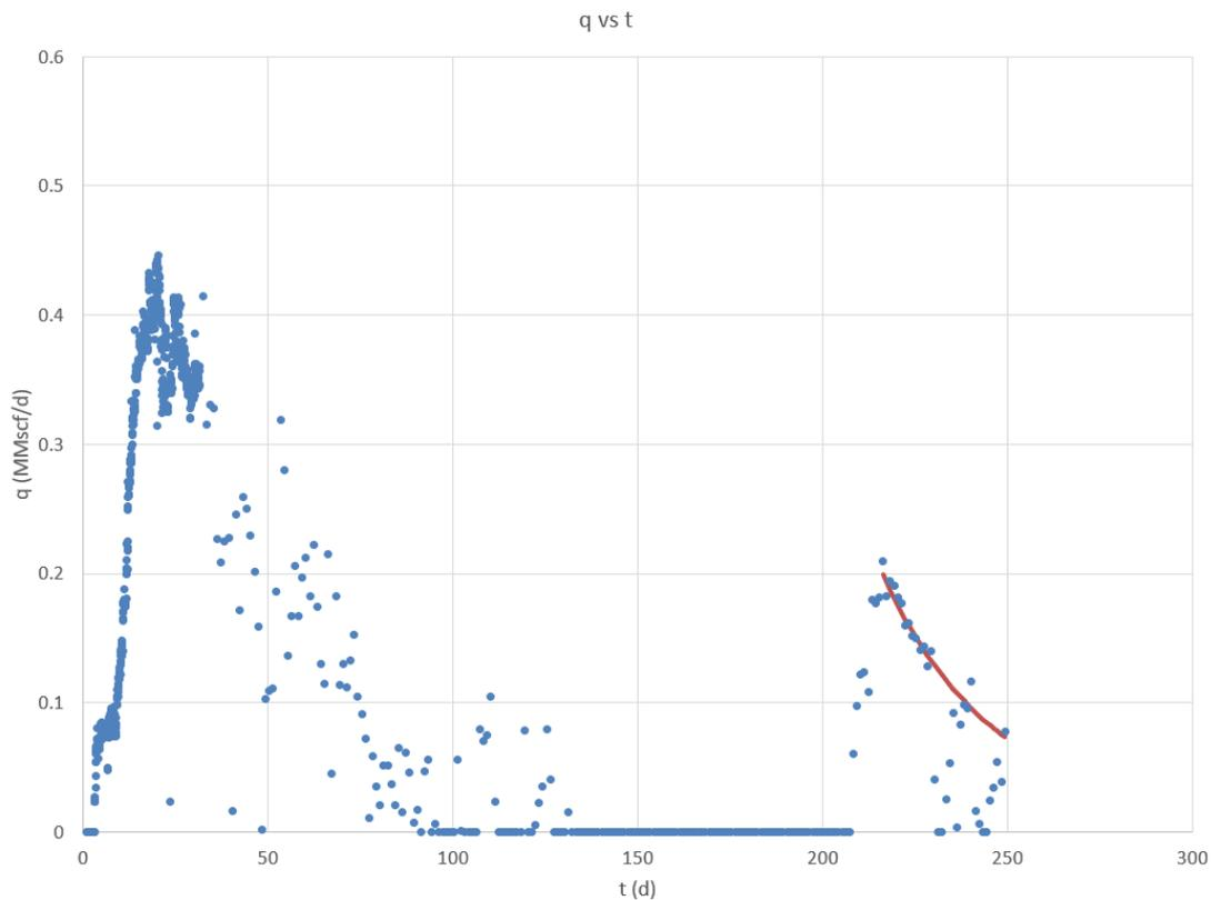
Figure 40. Well #3 production rate versus time plot with second decline curve fit.
