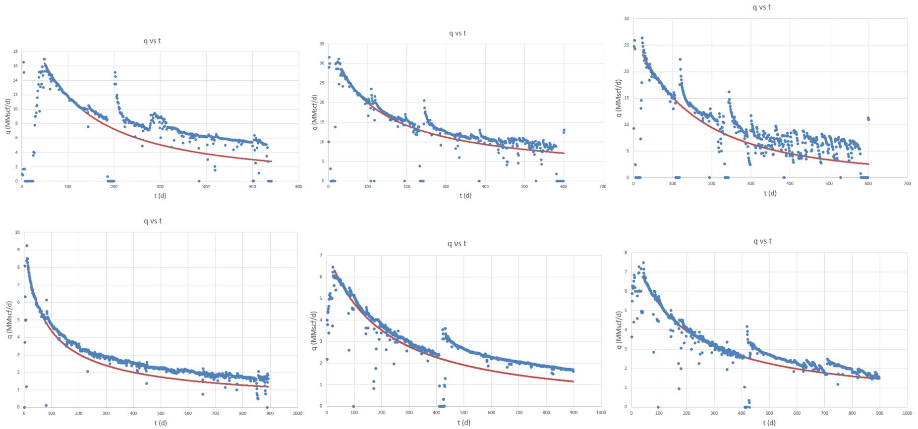
Figure A-5. Decline curve fit for the wells #35 (upper left), #36 (upper middle), #37 (upper right), #38 (bottom left), #39 (bottom middle), #40 (bottom right).
