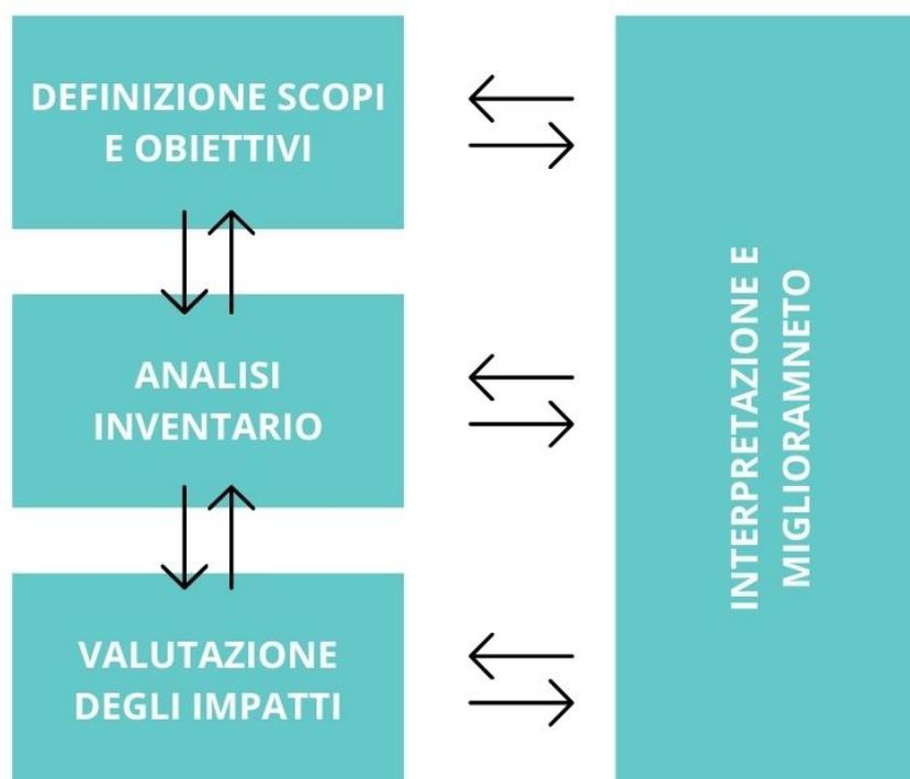
Figura 15 - Fasi LCA
