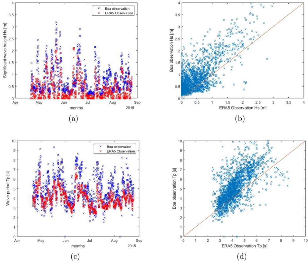
Figure 5.2: Comparison between buoy and ERA5 data
