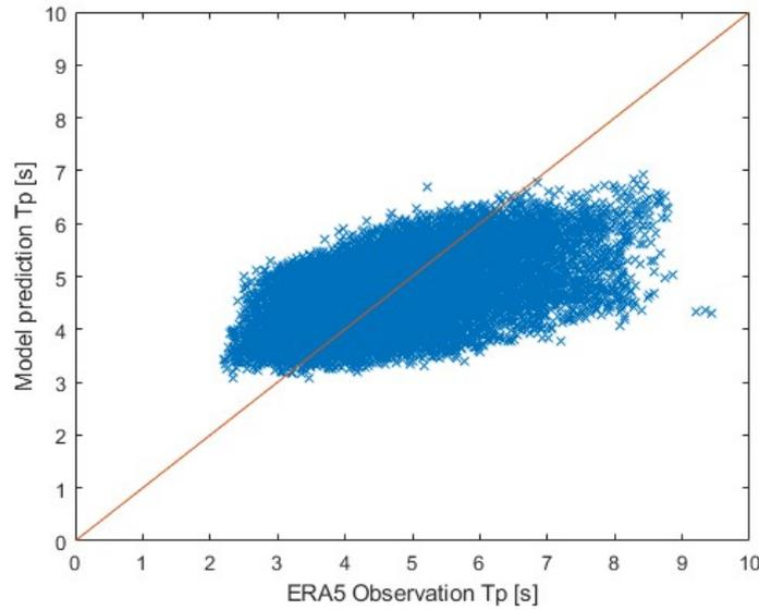
Figure 4.12: Comparison of linear multiple regression  $T_p$  prediction and ERA5 observation.
