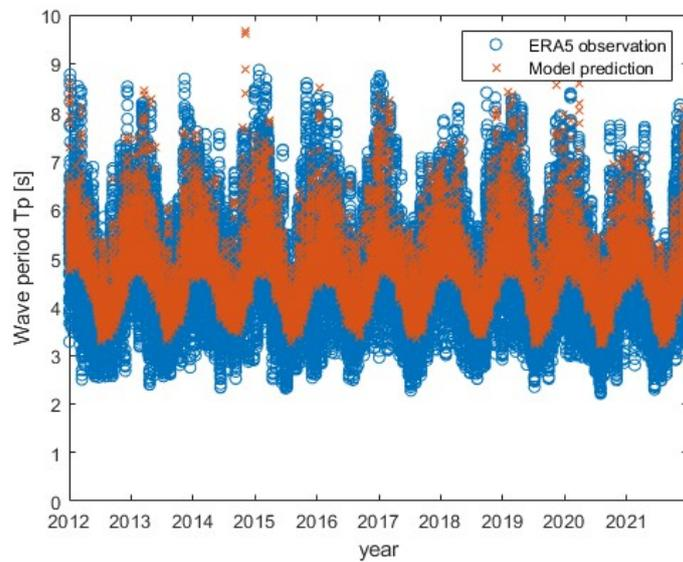
Figure 4.11: Linear multiple regression model results, mean wave period prediction.
