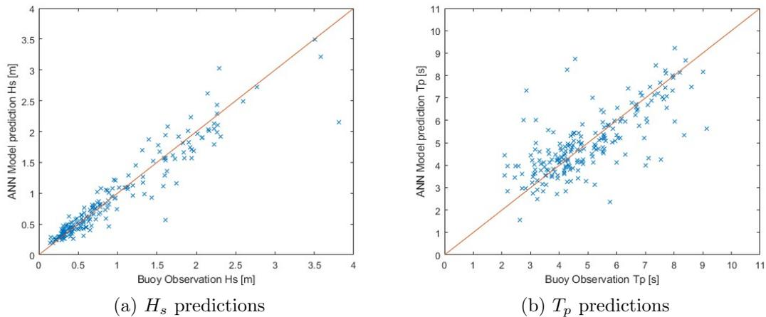
Figure 5.5: Quadratic multiple regression model performances with buoy data implementation.
