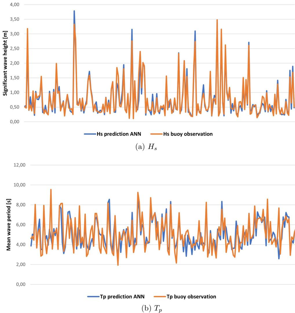
Figure 5.8: ANN model predictions with respect to buoy observations.
