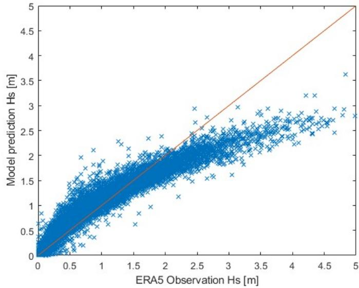
Figure 4.10: Comparison of linear multiple regression  $H_s$  prediction and ERA5 observation.
