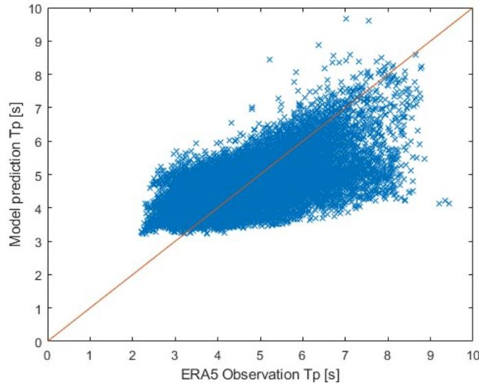
Figure 4.14: Comparison of quadratic multiple regression  $T_p$  prediction and ERA5 observation.
