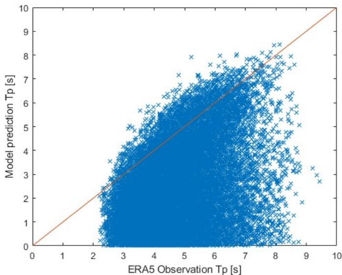
Figure 4.7: Comparison of SMB  $T_p$  prediction and ERA5 observation.
