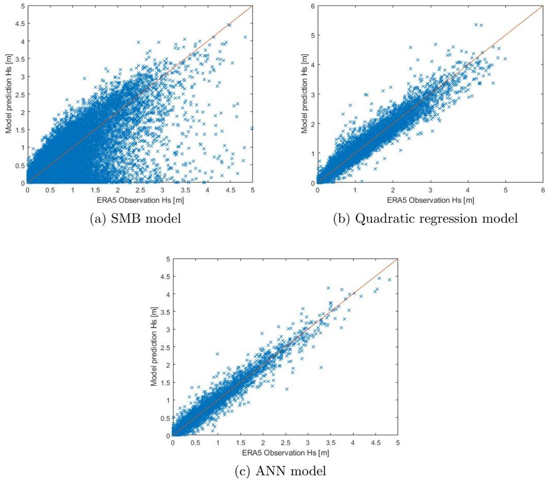
Figure 4.19:  $H_s$  prediction of different models.
