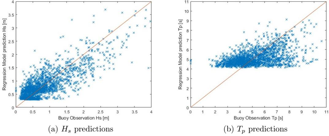
Figure 5.4: Quadratic multiple regression model performances with buoy data implementation.
