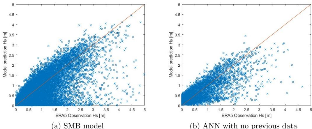
Figure 4.20:  $H_s$  prediction of SMB and ANN model with no previous data considered.
