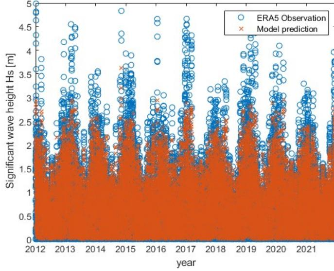
Figure 4.9: Linear multiple regression model results, significant wave height prediction.
