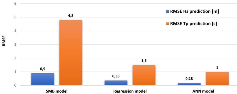
Figure 5.6: Model performances with buoy data implementation.
