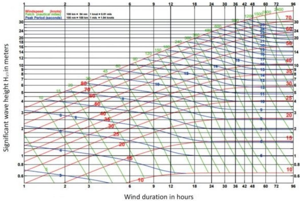
Figure 2.1: Manual wave-growth nomogram.
