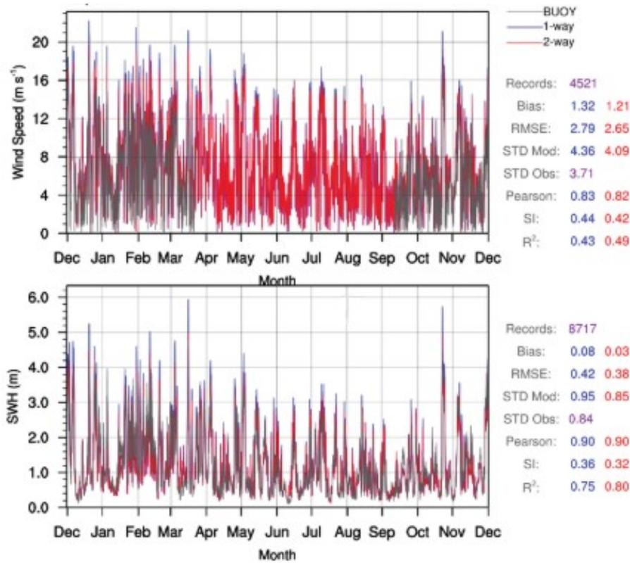
Figure 2.3: Results coupled atmosphere-ocean wave modelling system, namely CHAOS [27].
