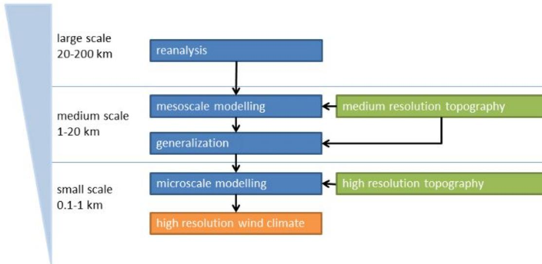
Figure 3.3: Schematic showing the methodology of the GWA is downscaling [44].
