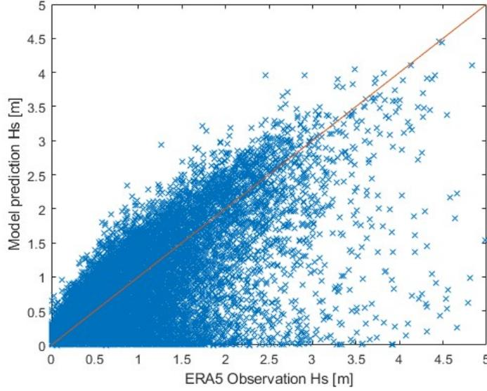
Figure 4.5: Comparison of SMB  $H_s$  prediction and ERA5 observation.
