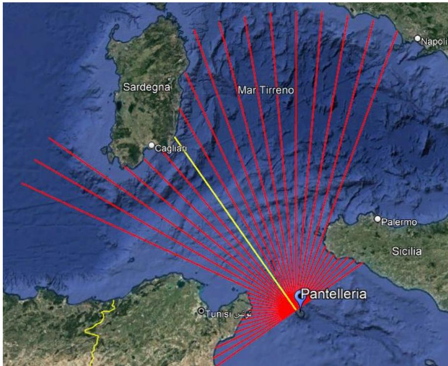
Figure 3.6: Fetch length from the the Island of Pantelleria.
