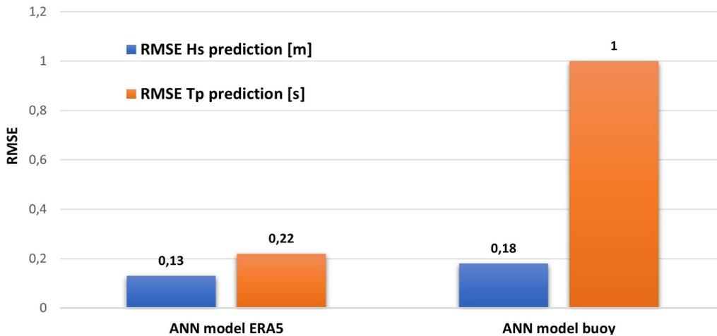
Figure 5.7: Comparison ANN model results between with ERA5 and buoy data implementation.
