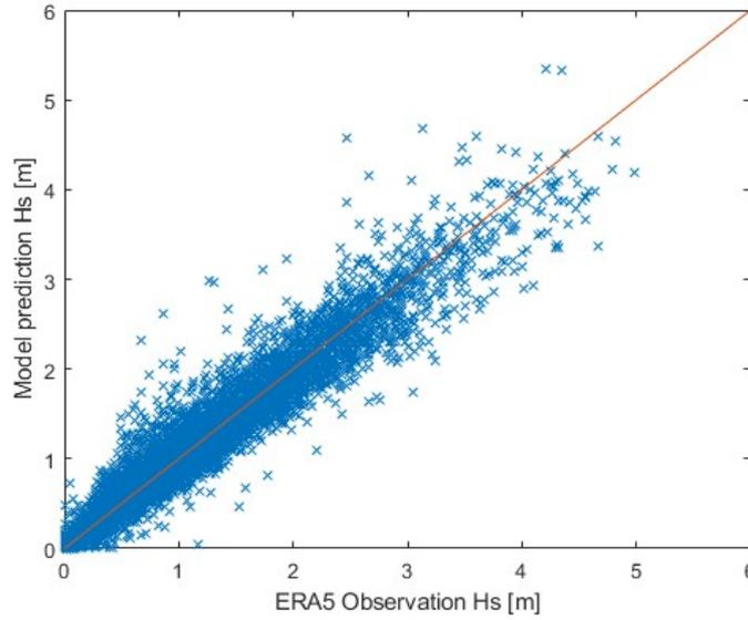
Figure 4.13: Comparison of quadratic multiple regression  $H_s$  prediction and ERA5 observation.
