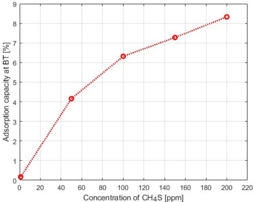
Figure 8.2: Adsorption capacity of CH<sub>4</sub>S at different concentrations
