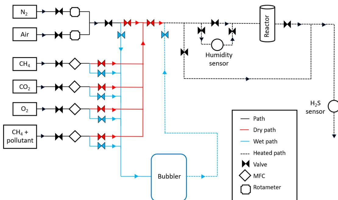
Figure 5.6: Gas station prototype schematic (personal elaboration)
