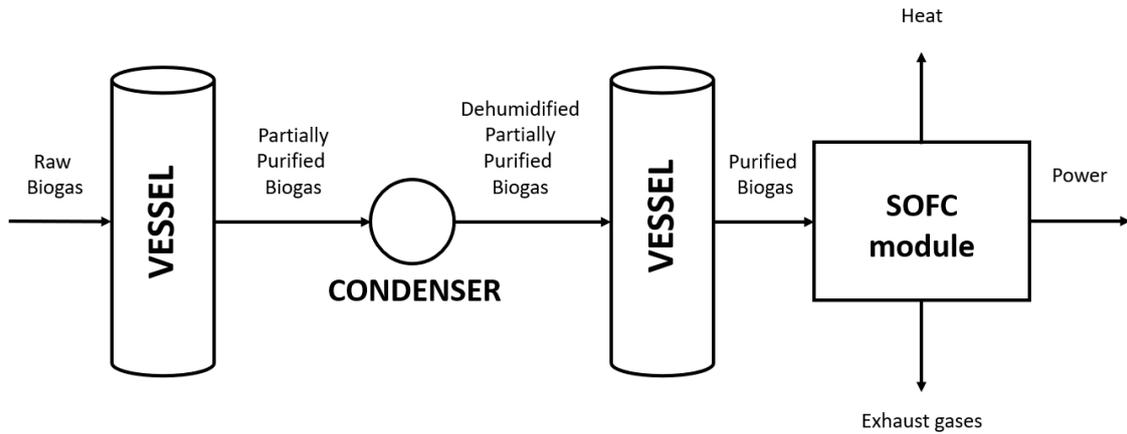
Figure 7.2: Purification process with 2 vessels and a condenser (personal elaboration)
