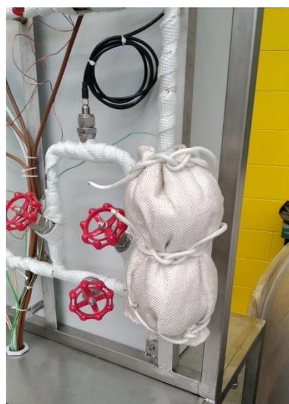
Figure 5.2: The coated reactor
