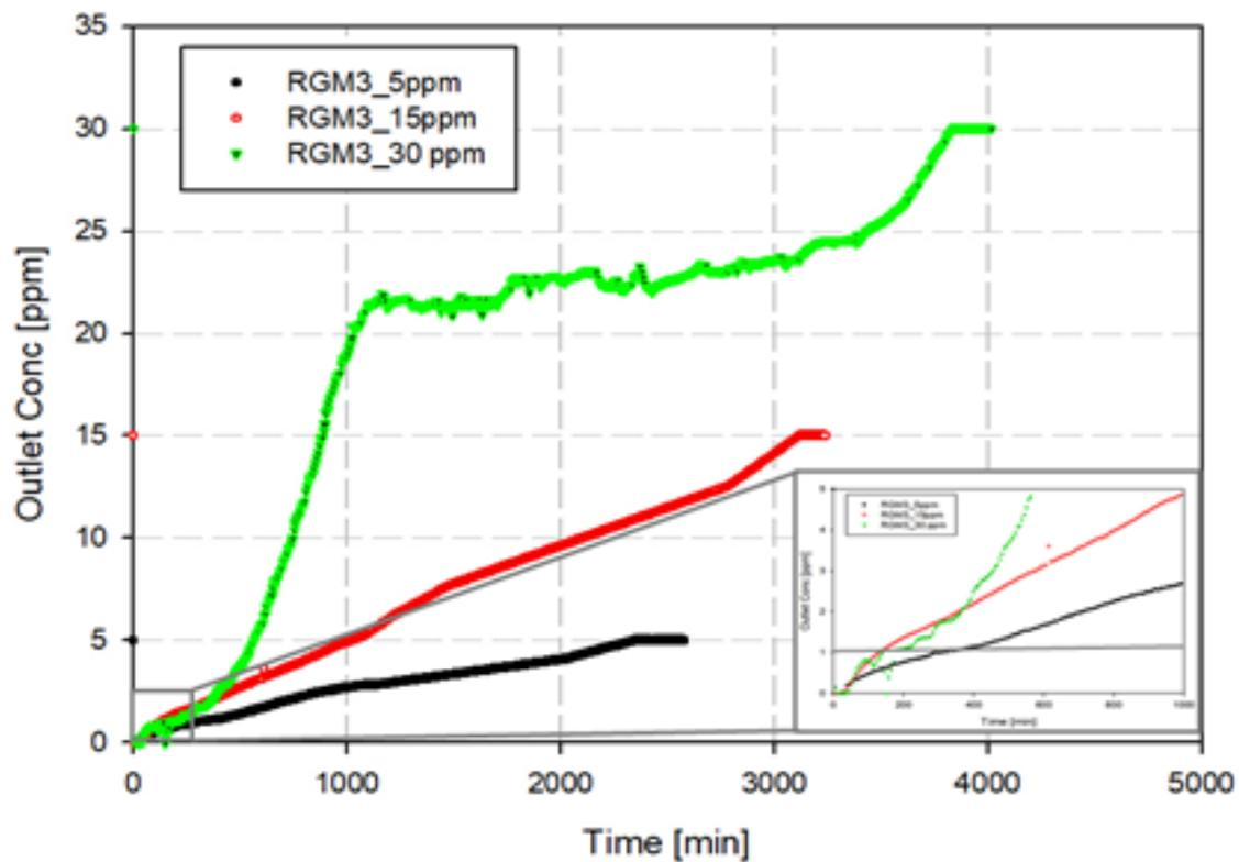
Figure 6.6: ENEA tests on COS at different inlet conditions [62]
