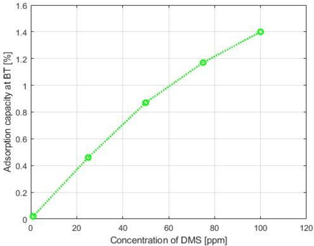
Figure 8.3: Adsorption capacity of DMS at different concentrations
