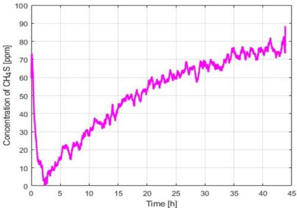
Figure 6.5: Test on Bioclean Gas Granular (100 ppm of  $\text{CH}_4\text{S}$ )
