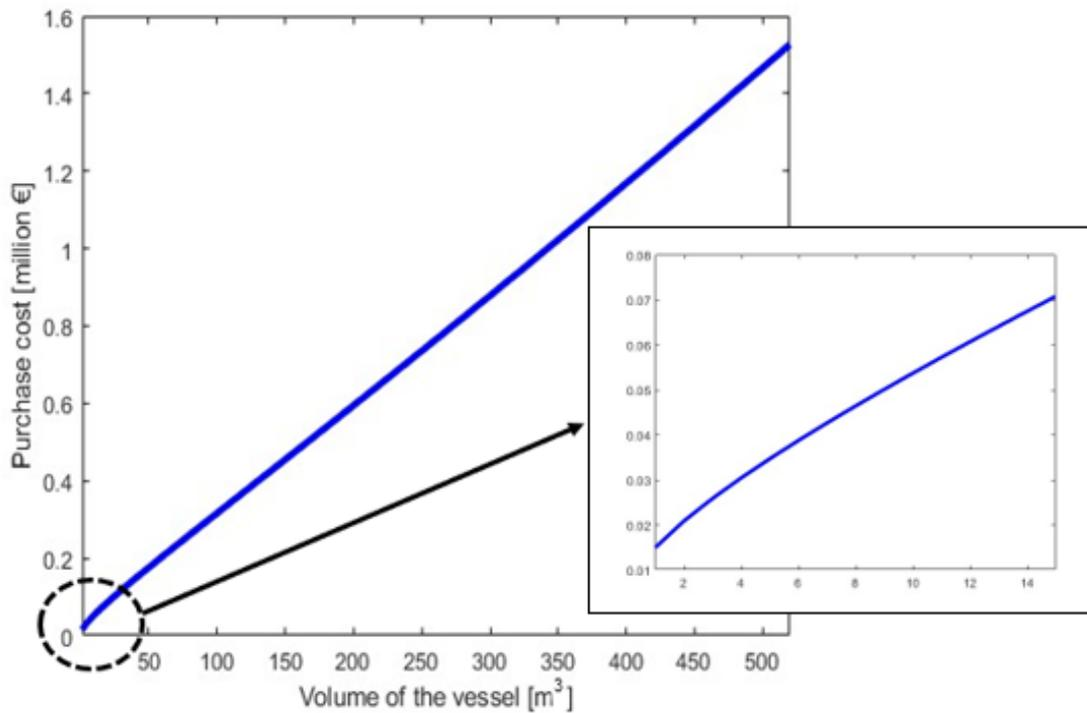
Figure 8.4: Purchase price of a vertical process vessel applying Turton cost functions
