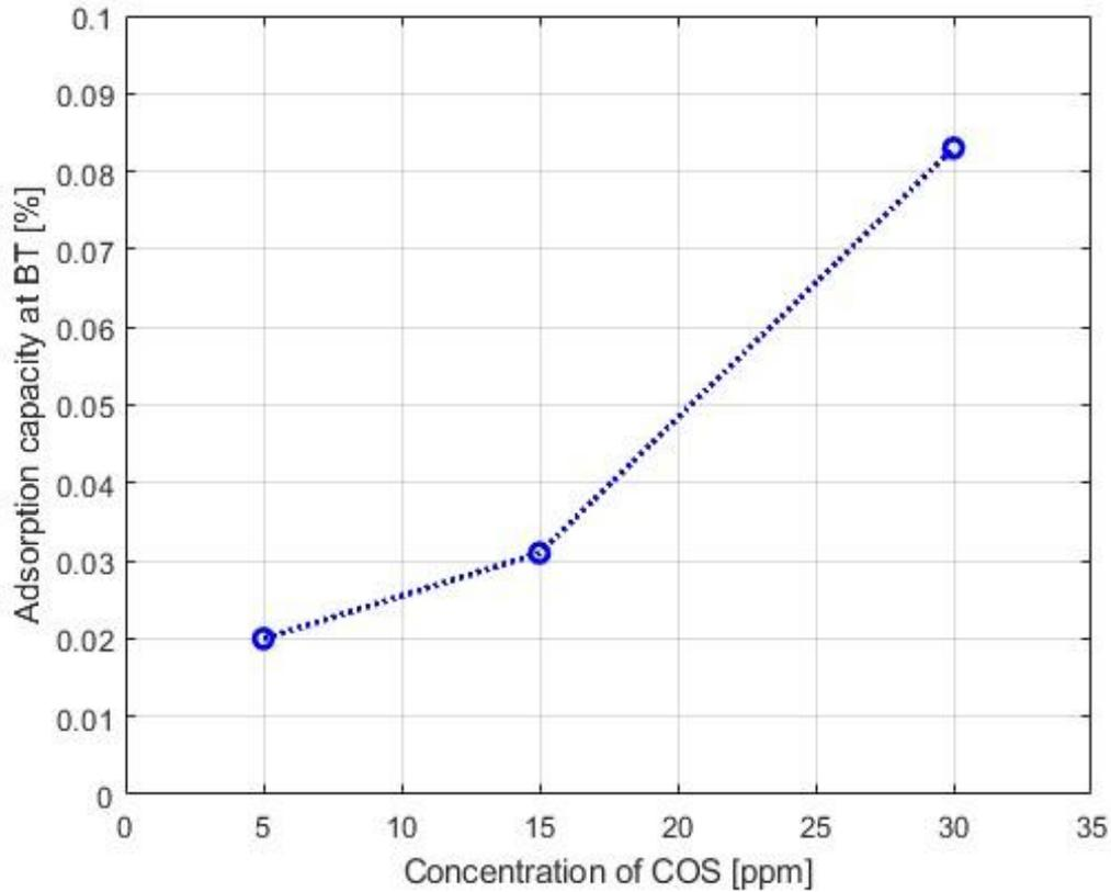
Figure 8.1: Tested adsorption capacity of Norit RGM-3 on COS removal at different concentrations
