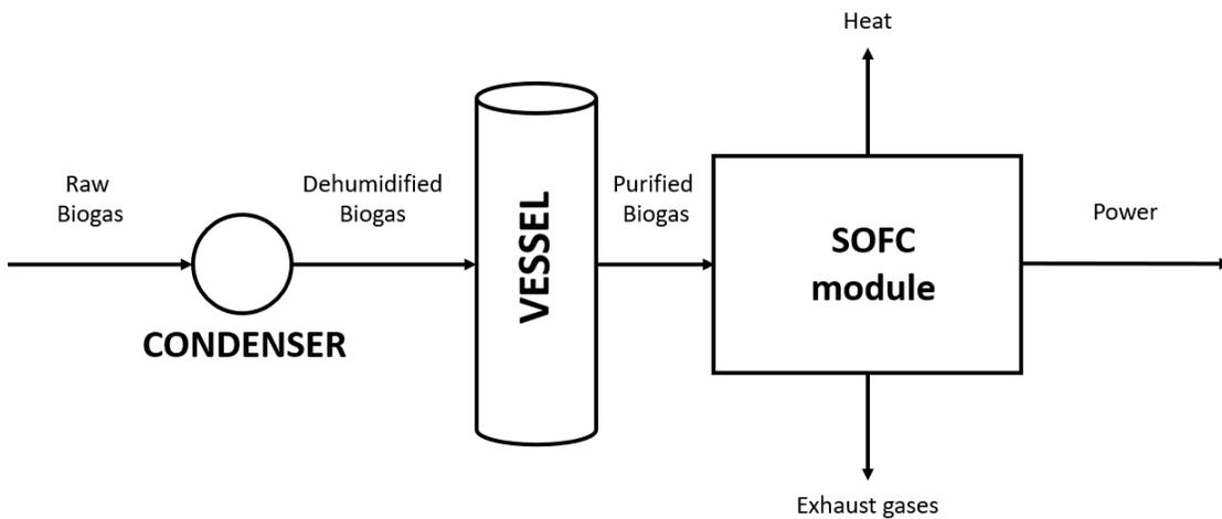
Figure 7.3: Purification process with a condenser and 1 vessel (personal elaboration)
