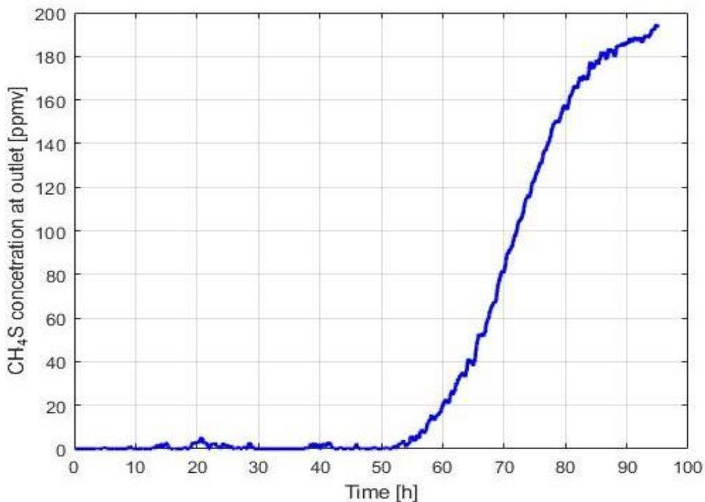
Figure 6.4: Test on Norit RGM-3 (200 ppm of CH<sub>4</sub>S)
