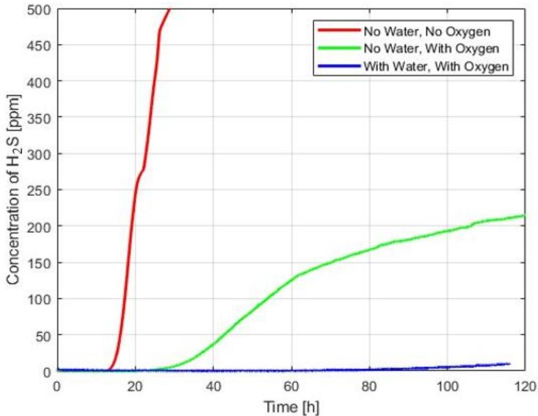
Figure 6.1: Tests on Norit RGM-3 in different conditions (500 ppm of H<sub>2</sub>S)
