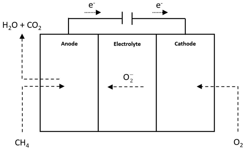
Figure 1.4: Schematic representation of a SOFC powered by methane (personal elaboration)
