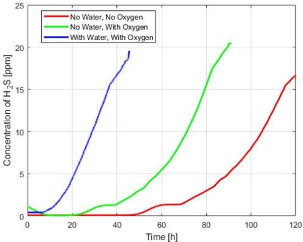
Figure 6.2: Tests on SulfaTrap R7H in different conditions (500 ppm of H<sub>2</sub>S)
