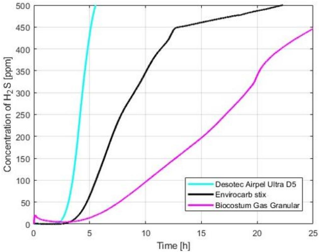
Figure 6.3: Tests on Desotec Airpel Ultra D5, Envirocarb stix and Biocostum Gas Granular (500 ppm of H<sub>2</sub>S, no water, no oxygen)
