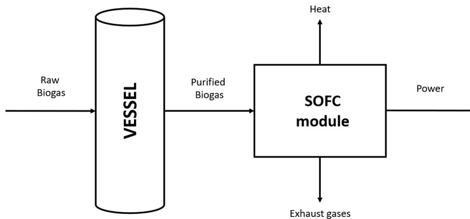
Figure 7.1: Purification with only one vessel (personal elaboration)
