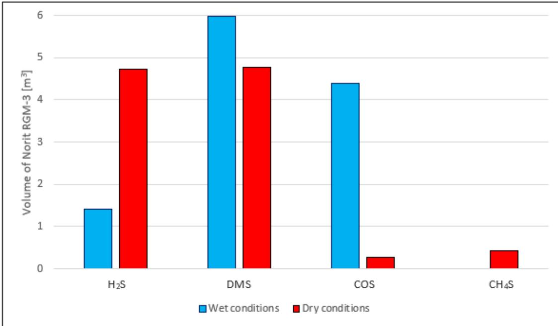
Figure 9.1: Comparison of the volume of Norit RGM-3 needed in different conditions for each component
