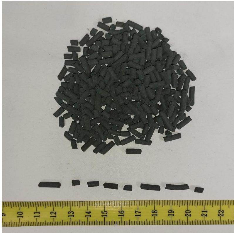
*Figure 5.8: SulfaTrap R7H*
