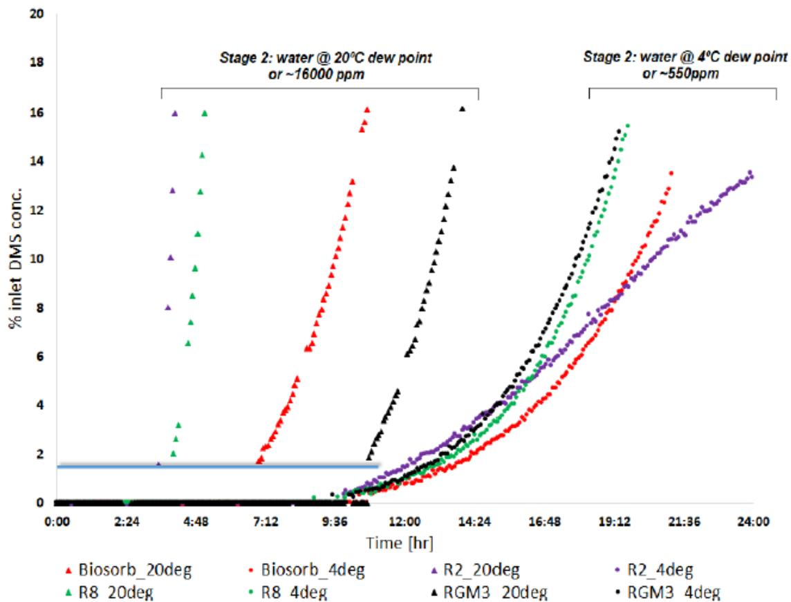
Figure 6.8: Breakthrough curves obtained for different materials (semi-wet and wet conditions, 100 ppm DMS) [62]
