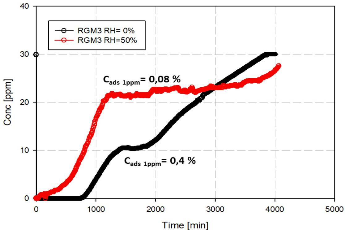
Figure 6.7: ENEA tests on COS in dry and wet conditions (30 ppm of COS) [62]
