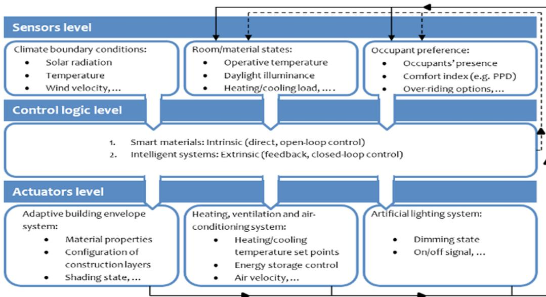
Figure 3: Scheme of the three levels of the control for RBEs [9].
