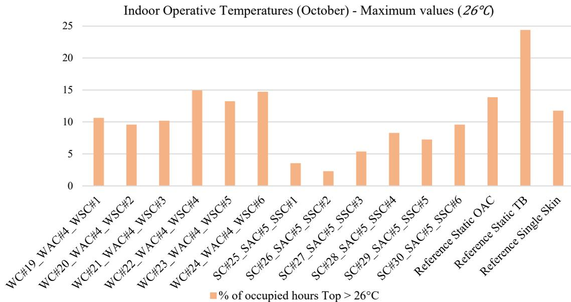
Figure 124: Percentages of occupied hours above  $26^{\circ}\text{C}$  for the different façade systems (October)
