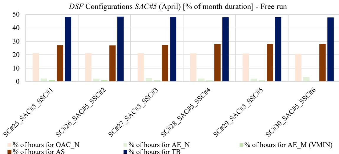
Figure 103: Percentages of hours in the month (April) in which the different DSF configurations have been adopted (active systems turned off) with SAC#5 as airflow control
