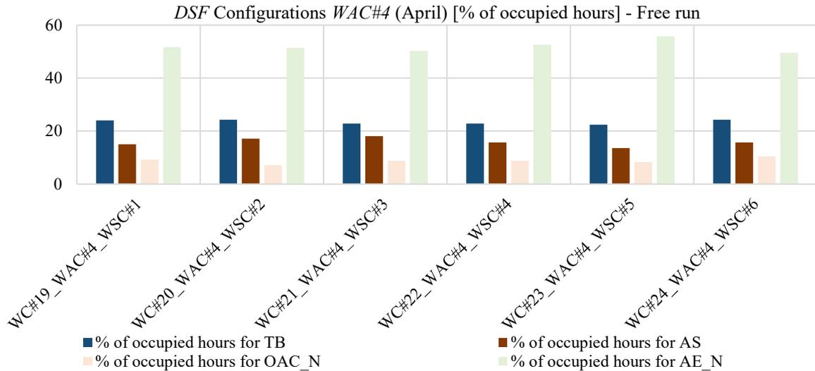
Figure 106: Percentages of occupied hours in the month (April) in which the different DSF configurations have been adopted (active systems turned off) with WAC#4 as airflow control
