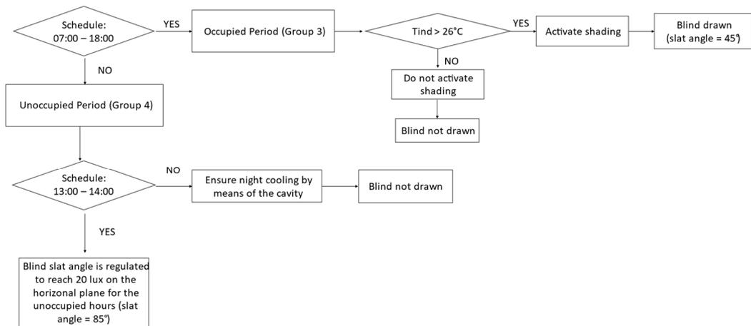
Figure 18: SSC#4 decision tree (Indoor air temperature activation + fixed slat angle)
