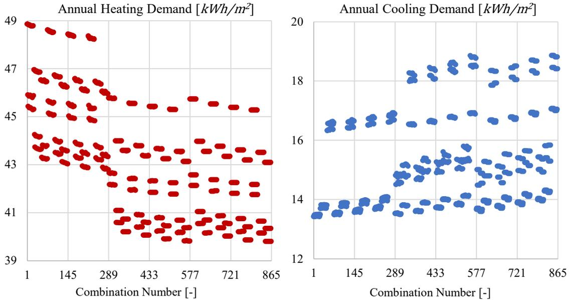
Figure 135: Heating (left) and cooling (right) energy need variation for the 864 different combinations
