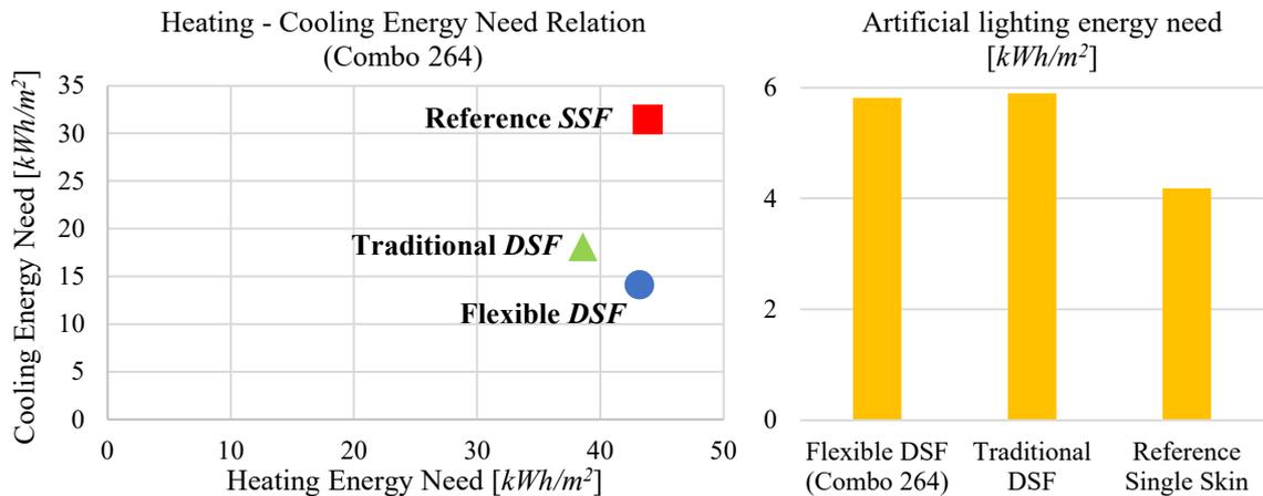
Figure 149: Relation between the heating and the cooling energy needs (left) for Combo 264 and related energy needs for artificial lighting (right)
