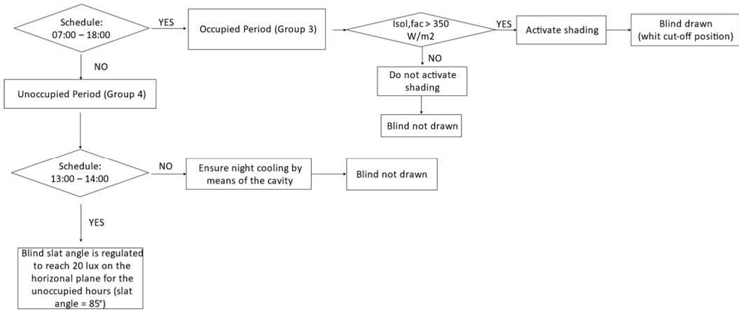
Figure 16: SSC#2 decision tree (Solar radiation activation + cut-off position)
