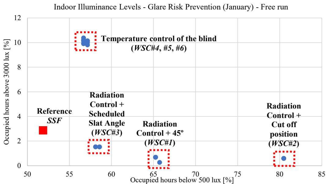
*Figure 93: Relation between the percentages of occupied hours in which the horizontal illuminance levels are above and below the limits of 3000 lux and 500 lux (January).*
