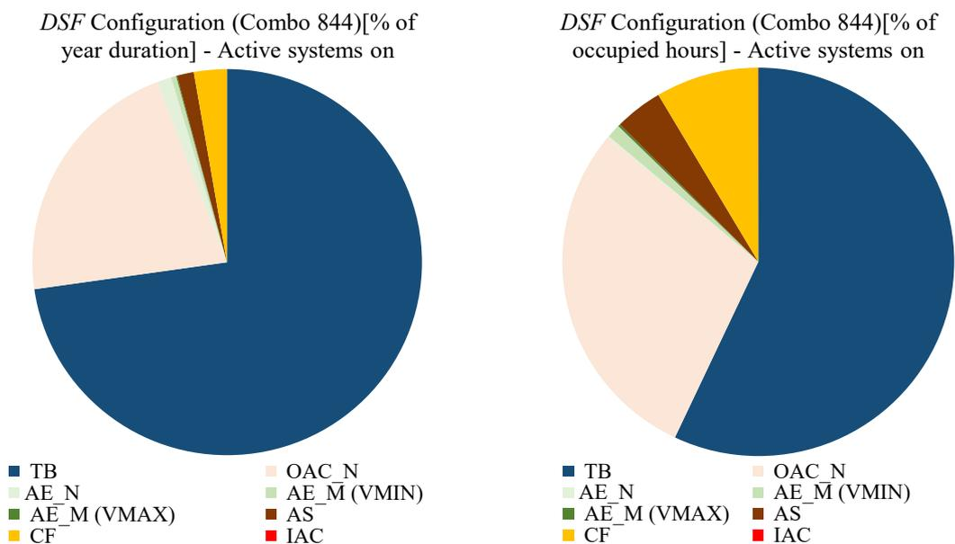
Figure 147: Flexible *DSF* configuration through the year for combo 844: overall month duration (left) and occupied hours (right)
