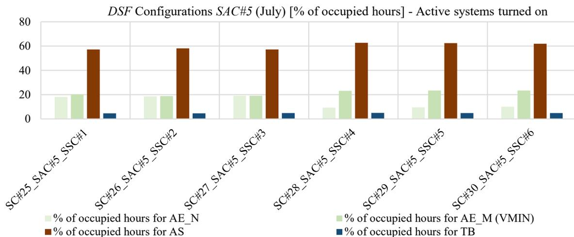
Figure 48: Percentages of occupied hours in the month (July) in which the different DSF configurations have been adopted (active systems turned on) with SAC#5 as airflow control
