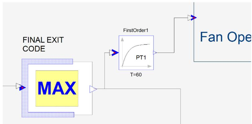
Figure 213: The First Order Operator module adopted to retard the response of the façade actuators. In this case the selected period is 60 seconds.
