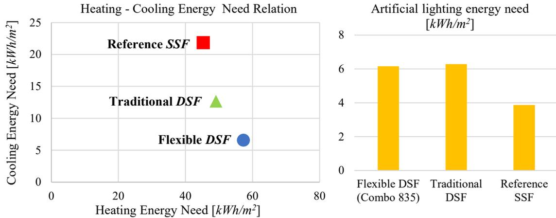
Figure 185: Relation between the heating and the cooling energy needs (left) for Combo 835 and related energy needs for artificial lighting in Oslo (right).
