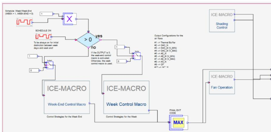
Figure 203: Control implementation for the cavity air flows (on the left) and the shading system (on the right) in the central Control Macro of the DSF
