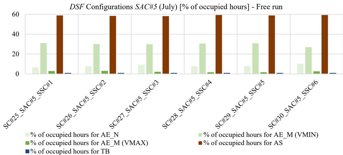
Figure 66: Percentages of occupied hours in the month (July) in which the different DSF configurations have been adopted (active systems turned off) with SAC#5 as airflow control
