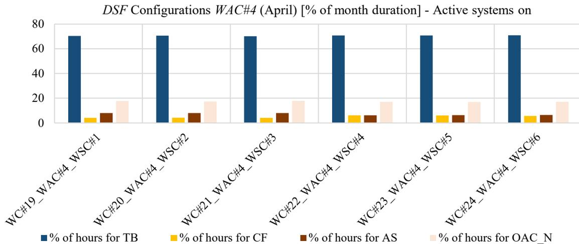
*Figure 98: Percentages of hours in the month (April) in which the different DSF configurations have been adopted (active systems turned on) with WAC#4 as airflow control*
