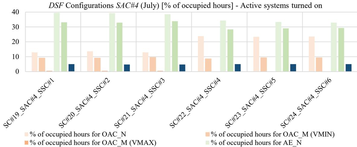
Figure 47: Percentages of occupied hours in the month (July) in which the different DSF configurations have been adopted (active systems turned on) with SAC#4 as airflow control
