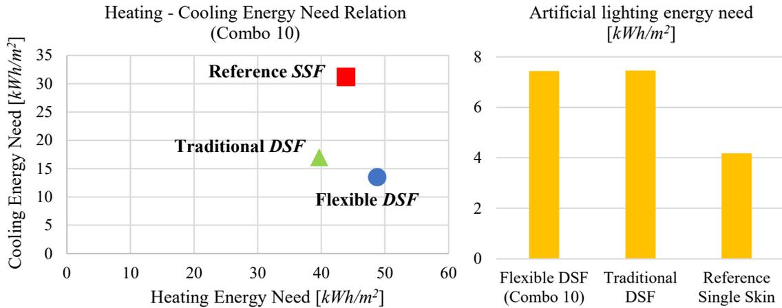
Figure 139: Relation between the heating and the cooling energy needs for Combo 10 (left) and related artificial lighting energy needs (right)
