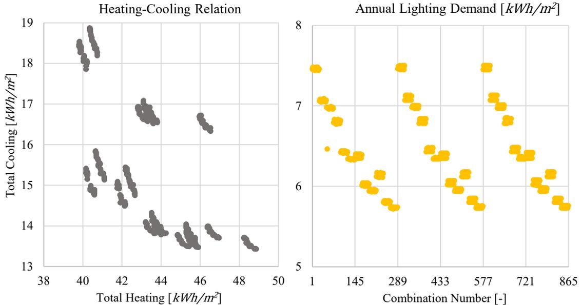
Figure 136: Heating/Cooling energy need relation (left) and artificial lighting energy need variation (right) for the 864 different combinations
