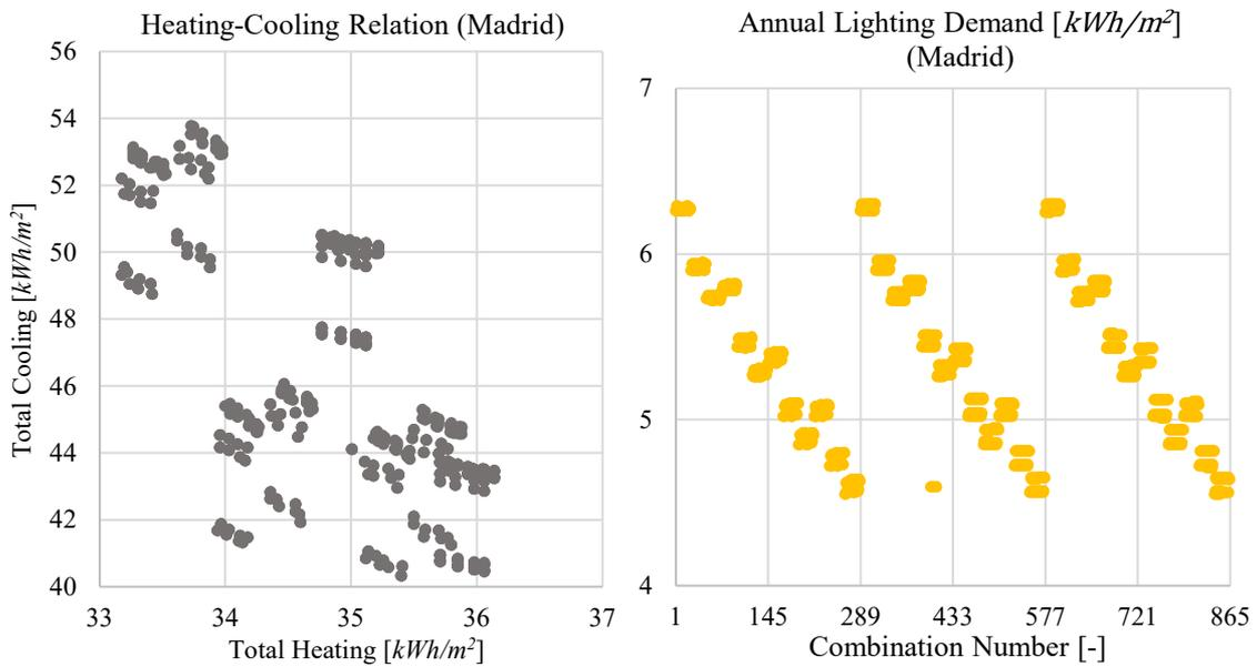
Figure 166: Heating/Cooling energy need relation (left) and artificial lighting energy need variation (right) for the 864 different combinations in Madrid
