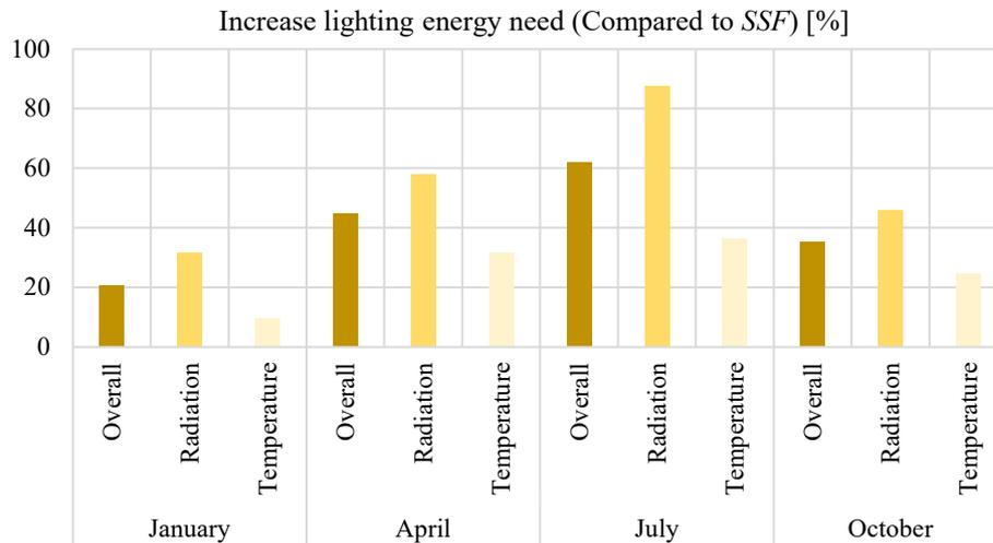
*Figure 131: Average lighting energy need increase in four considered months, considering the one produced by the radiation control, the temperature control and both together*
