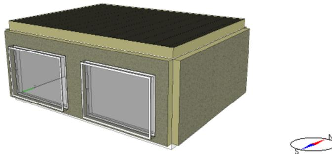
Figure 32: The BESTEST cell used for the thermal zone modelling, with the two identical DSFs applied on the South wall.
