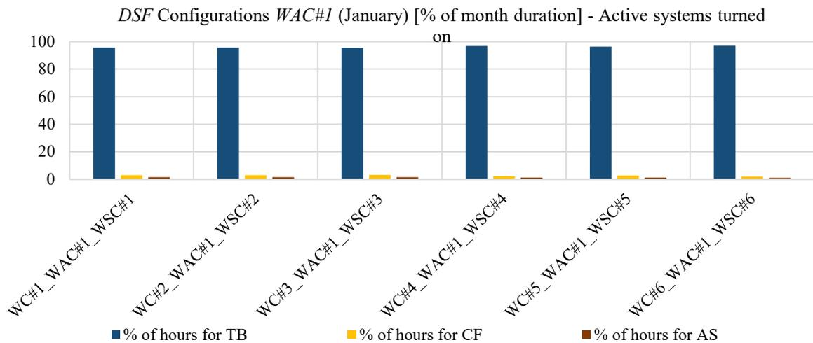
Figure 49: Percentages of hours in the month (January) in which the different DSF configurations have been adopted (active systems turned on) with *WAC#1* as airflow control
