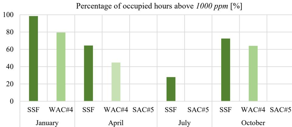
Figure 132: Percentage of occupied hours above the limit of 1000 ppm in the four considered months
