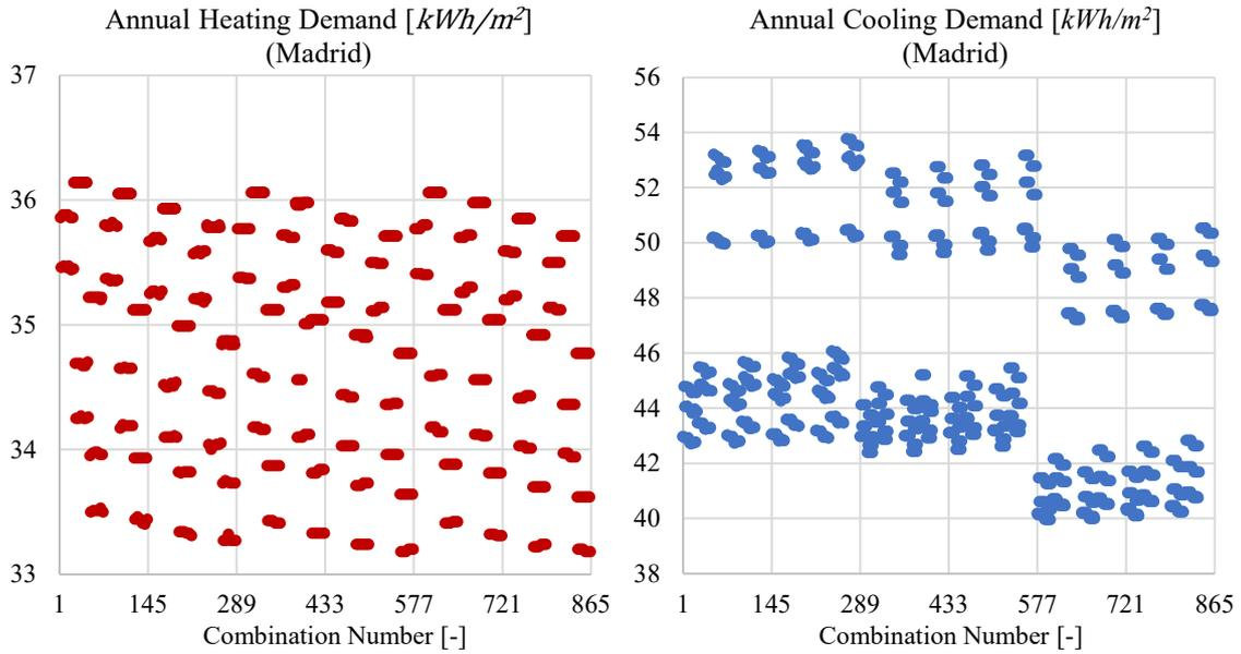
Figure 165: Heating (left) and cooling (right) energy need variation for the 864 different combinations in Madrid
