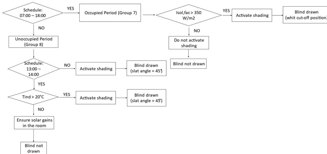
Figure 26: WSC#2 decision tree (Solar radiation activation + cut-off position)
