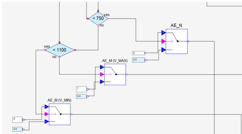
Figure 204: Example of switch modules at the end of a decision tree implemented in IDA ICE for the selection of the confirmation number (in this case 5, 6 and 7).
