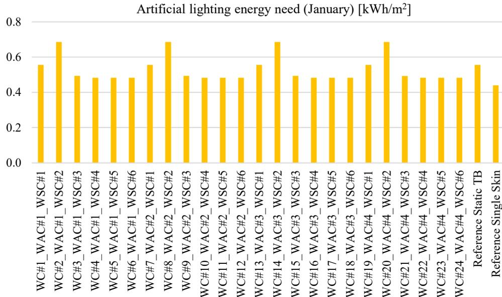
Figure 79: Artificial lighting energy requirements for the different façade systems (January)
