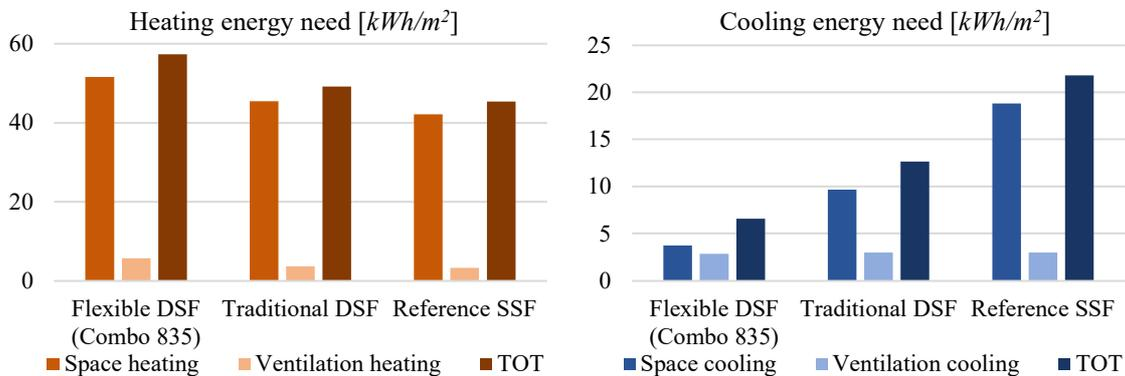
Figure 184: Heating (left) and cooling (right) energy need variation (Combo 835) in Oslo
