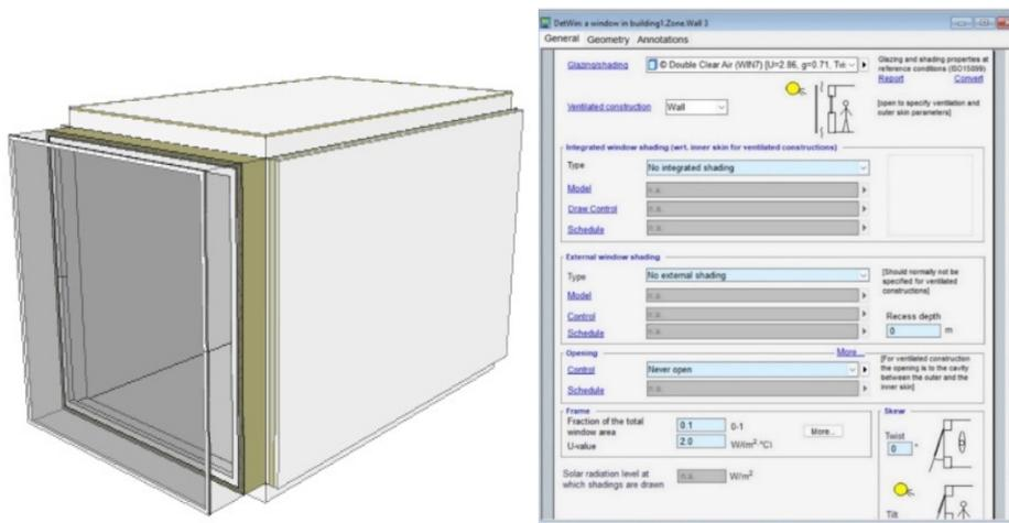
Figure 197: 3D view of the *DSF* in-built model from the IDA ICE graphic interface (left) and Detailed window form in IDA ICE. The glazing properties are referred to the inner skin of the *DSF*. In the “Ventilated construction” field the selection “Wall” enables the creation of the *DSF* model (right).
