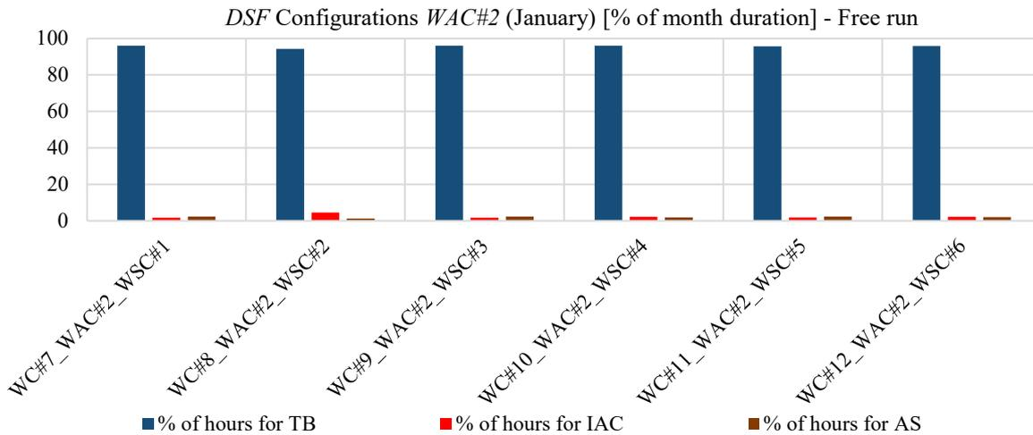
Figure 68: Percentages of hours in the month (January) in which the different DSF configurations have been adopted (active systems turned off) with *WAC#2* as airflow control
