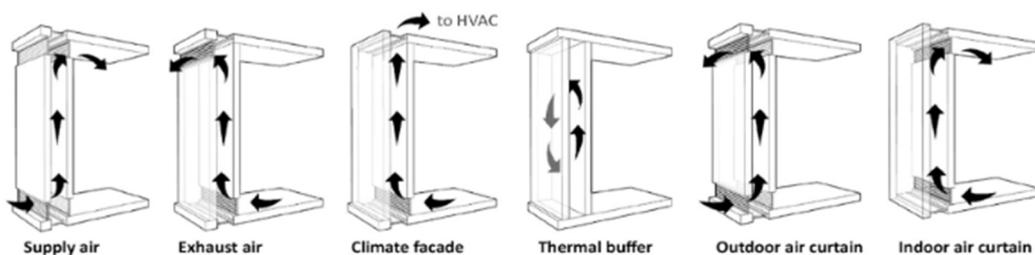
*Figure 196: DSF ventilation modes classification [20].*
