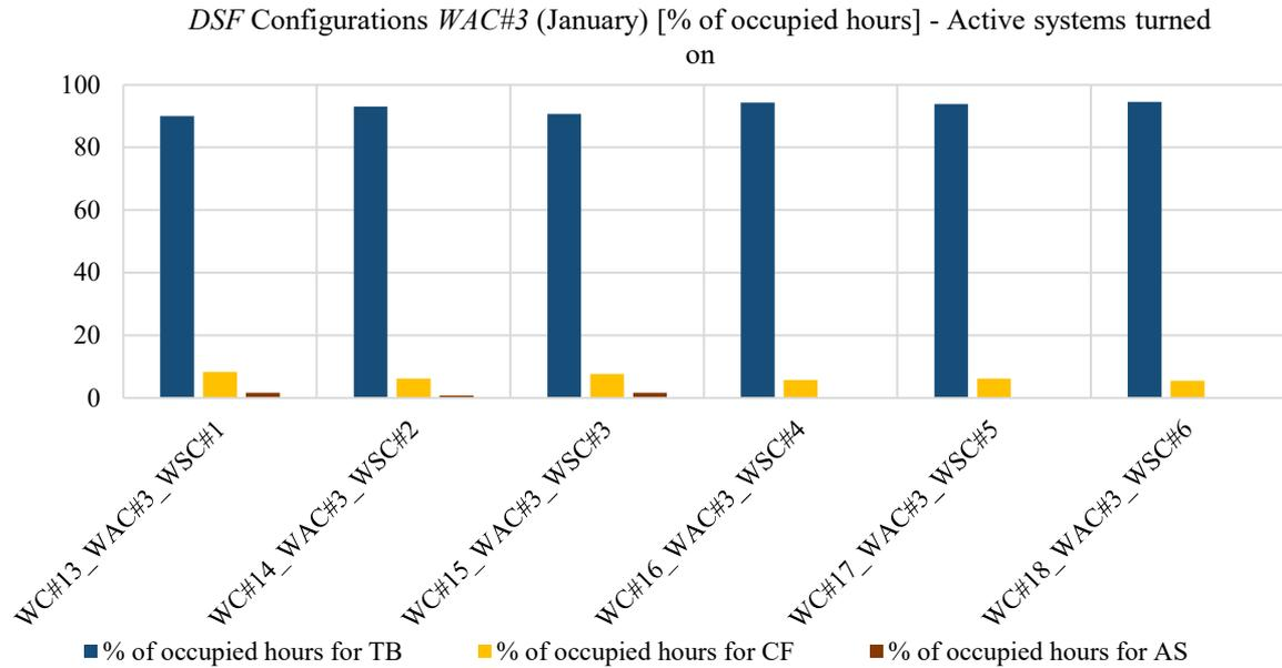
Figure 55: Percentages of occupied hours in the month (January) in which the different DSF configurations have been adopted (active systems turned on) with WAC#3 as airflow control
