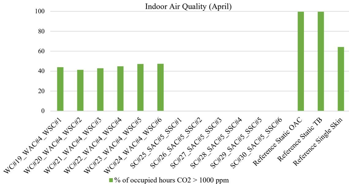
Figure 110: Percentages of occupied hours above 1000 ppm for the different façade systems (April)
