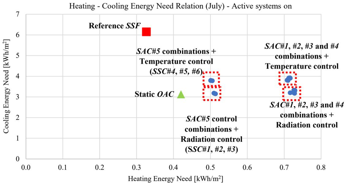
*Figure 91: Relation between the heating and cooling energy needs of the room with the adoption of the different façade system (July).*
