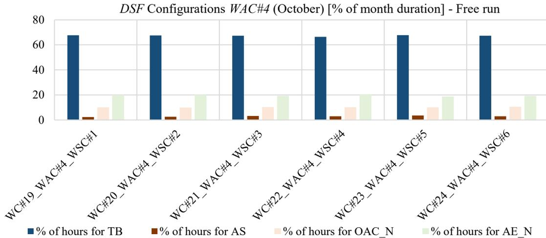
Figure 122: Percentages of hours in the month (October) in which the different DSF configurations have been adopted (active systems turned off) with WAC#4 as airflow control
