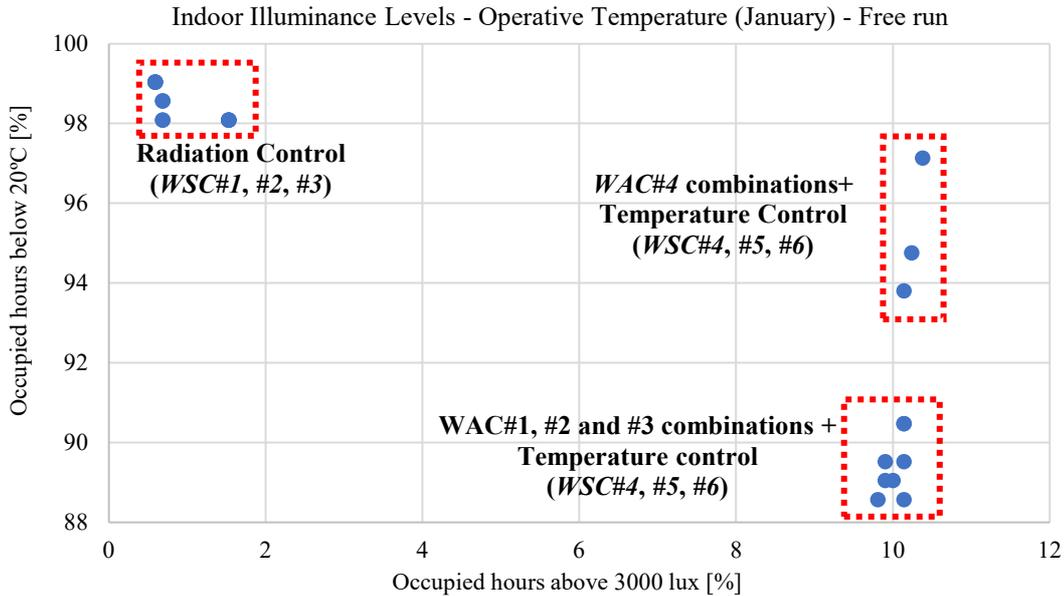
Figure 94: Relation between the percentages of occupied hours in which the horizontal illuminance levels are above 3000 lux and the percentages of occupied hours in which the indoor operative temperature is below 20°C.
