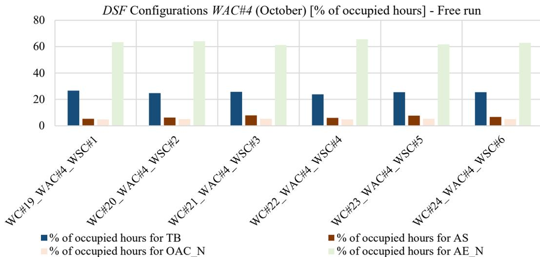
Figure 123: Percentages of occupied hours in the month (October) in which the different DSF configurations have been adopted (active systems turned off) with WAC#4 as airflow control
