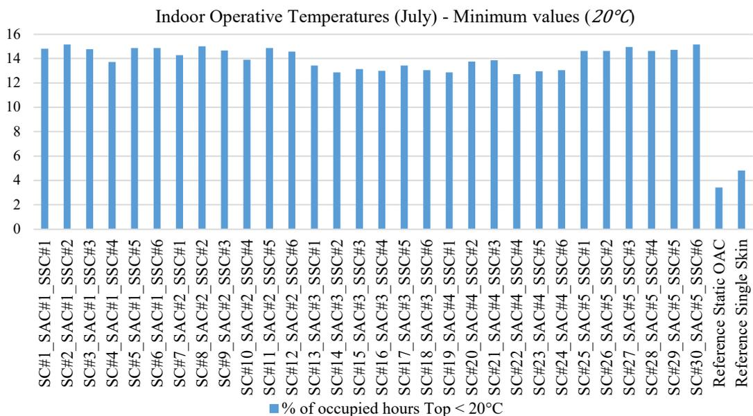
Figure 82: Percentages of occupied hours below 20°C for the different façade systems (July)
