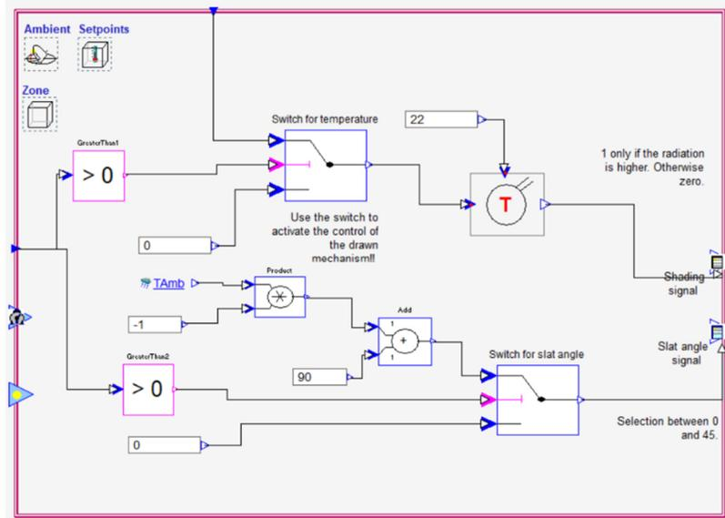
Figure 208: Use of the IDA ICE Control Macro for the application of the shading control
