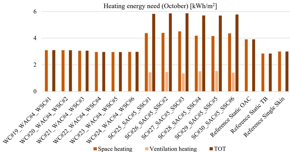
Figure 117: Heating energy requirements for the different façade systems (October)
