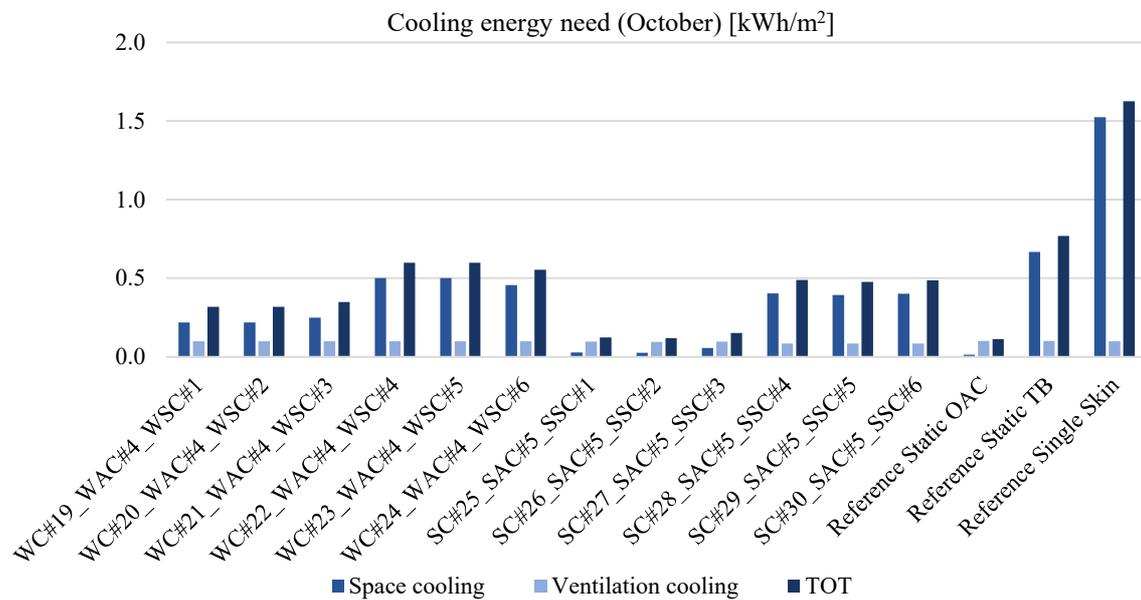
Figure 118: Cooling energy requirements for the different façade systems (October)
