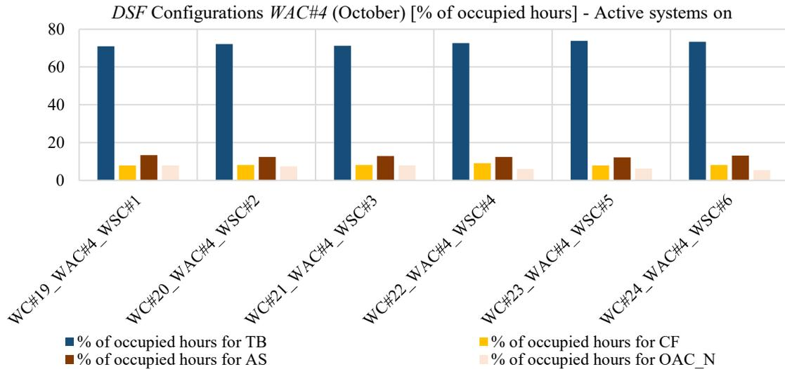
Figure 116: Percentages of occupied hours in the month (October) in which the different DSF configurations have been adopted (active systems turned on) with WAC#4 as airflow control
