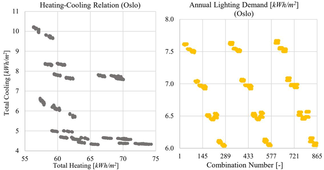
Figure 182: Heating/Cooling energy need relation (left) and artificial lighting energy need variation (right) for the 864 different combinations in Oslo
