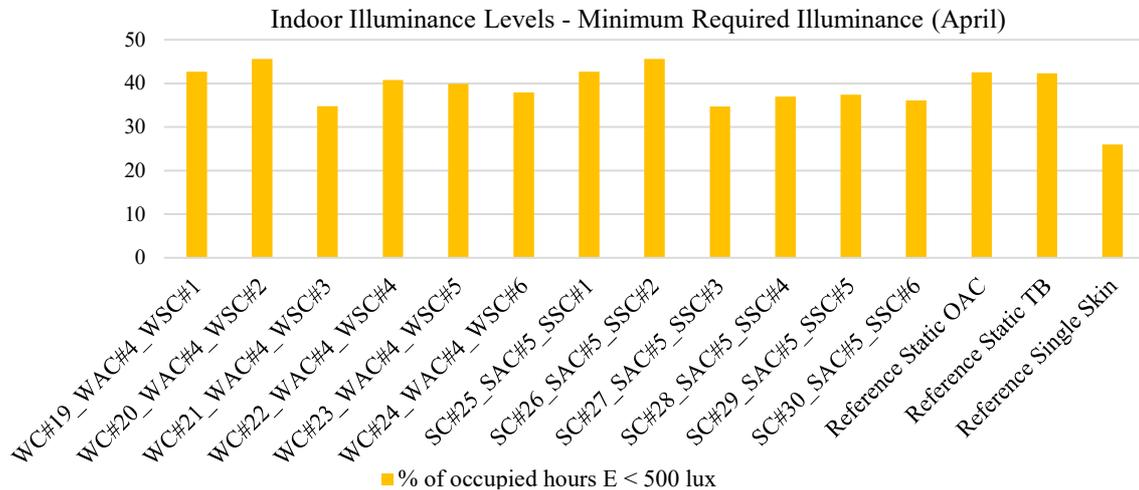
Figure 112: Percentage of occupied hours below the limit of *500 lux* (April)
