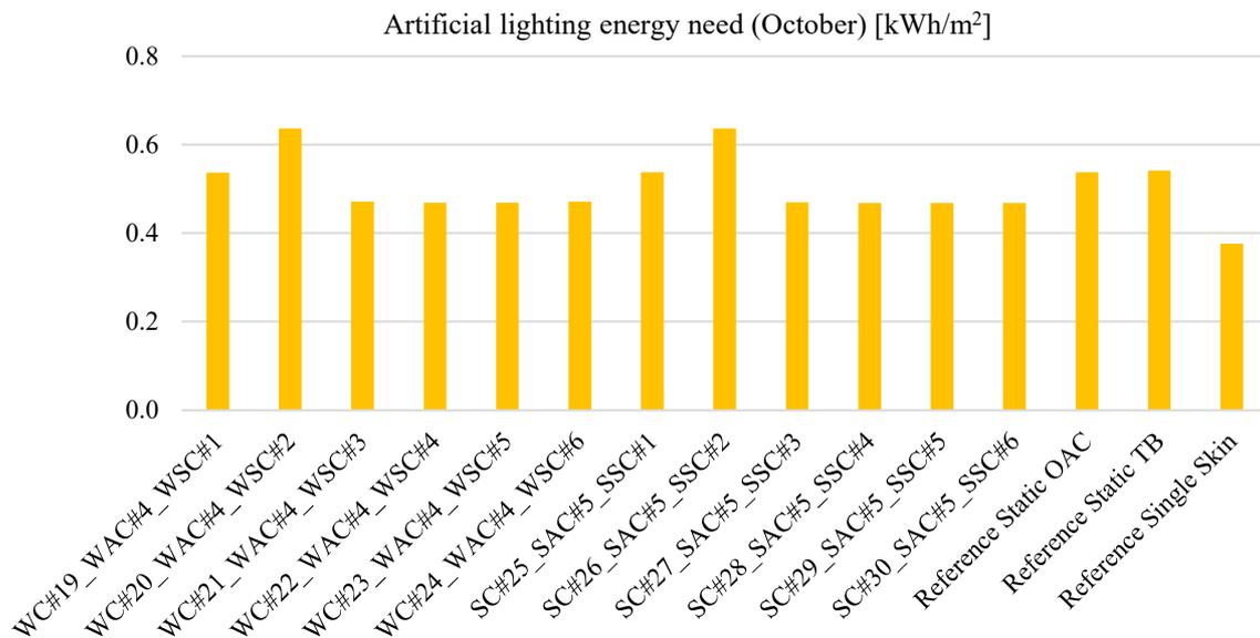
Figure 119: Artificial lighting energy requirements for the different façade systems (October)
