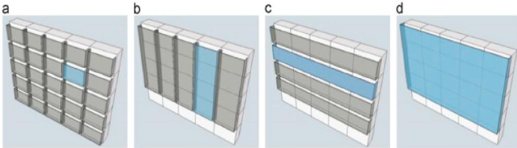
*Figure 195: Pictures of the DSF layouts: a) box window, b) shaft-box, c) corridor façade and d) multi-storey façade [20].*
