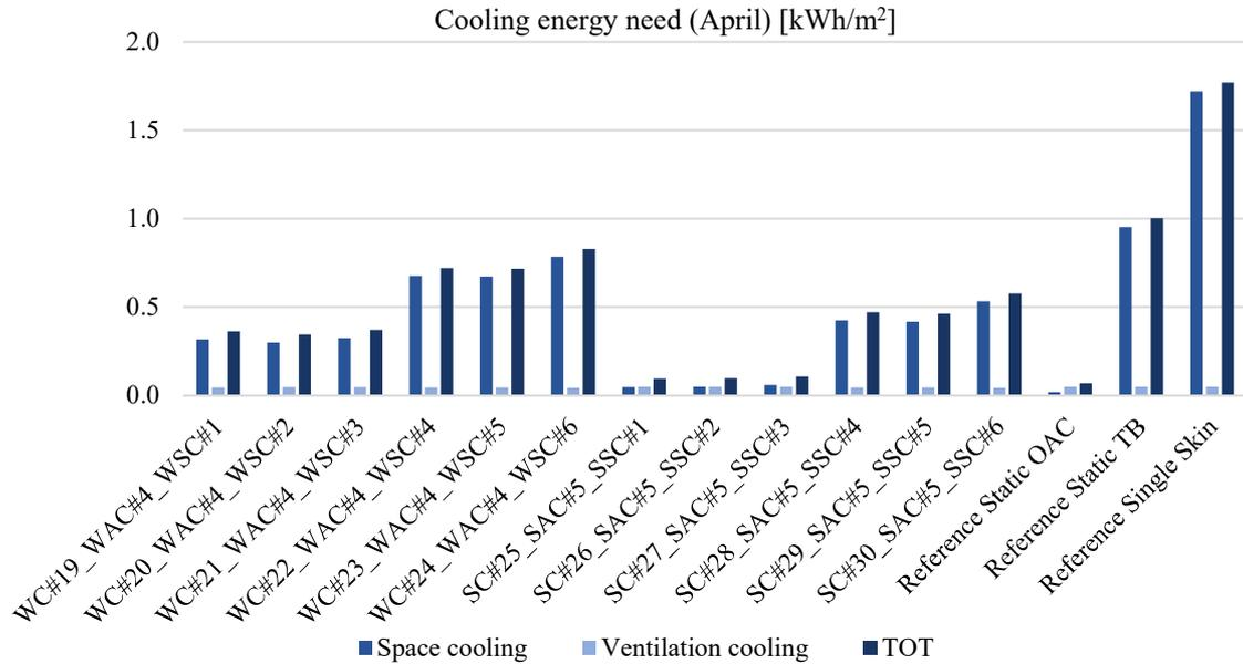
Figure 101: Cooling energy requirements for the different façade systems (April)
