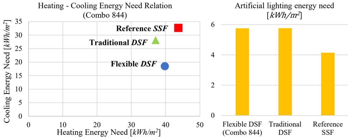
Figure 144: Relation between the heating and the cooling energy needs (left) for Combo 844 and related energy needs for artificial lighting (right).
