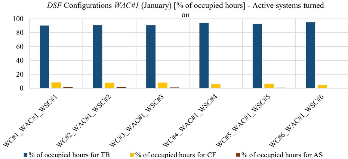
Figure 53: Percentages of occupied hours in the month (January) in which the different DSF configurations have been adopted (active systems turned on) with WAC#1 as airflow control
