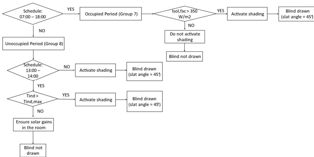
Figure 25: WSC#1 decision tree (Solar radiation activation + fixed slat angle)
