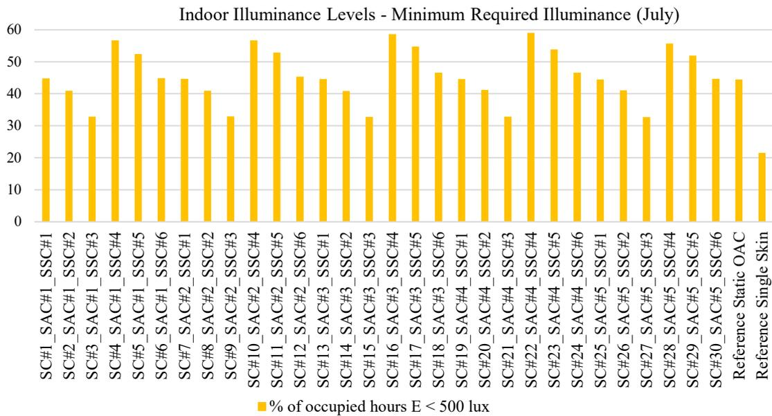
Figure 85: Percentage of occupied hours below the limit of 500 lux (July)
