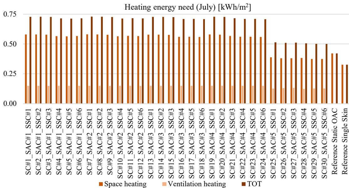
Figure 75: Heating energy requirements for the different façade systems (July)
