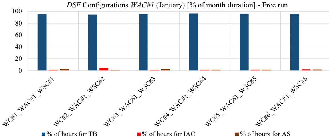
Figure 67: Percentages of hours in the month (January) in which the different DSF configurations have been adopted (active systems turned off) with *WAC#1* as airflow control
