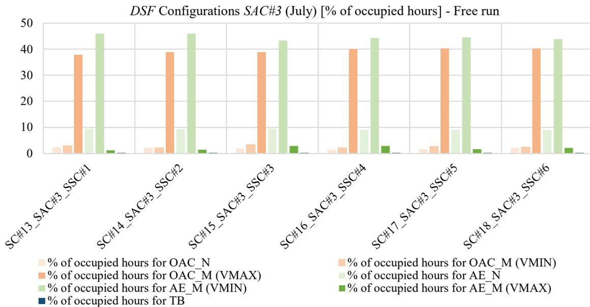
Figure 64: Percentages of occupied hours in the month (July) in which the different DSF configurations have been adopted (active systems turned off) with SAC#3 as airflow control
