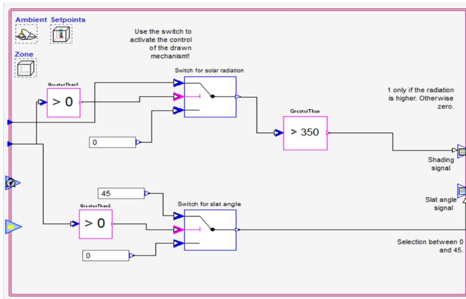
Figure 192: Control macro example from IDA ICE for the control of the shading system
