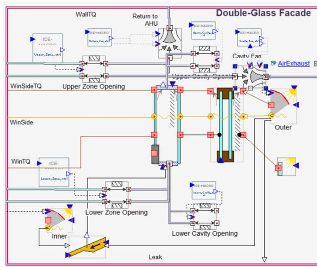
Figure 201: The modified configuration of the DSF system implemented inside IDA ICE
