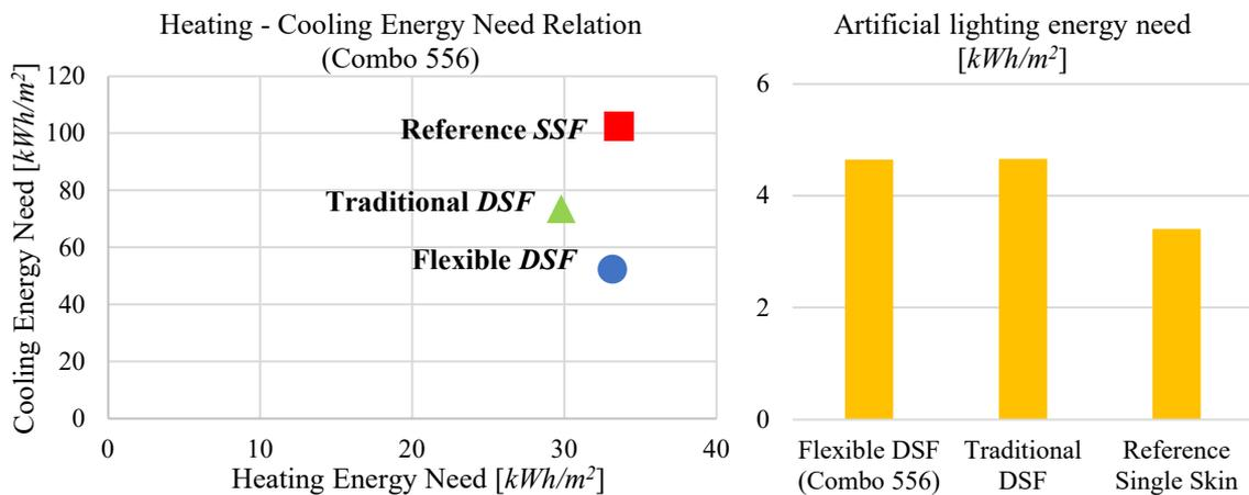
Figure 174: Relation between the heating and the cooling energy needs (left) for Combo 556 and the related energy needs for artificial lighting (right).
