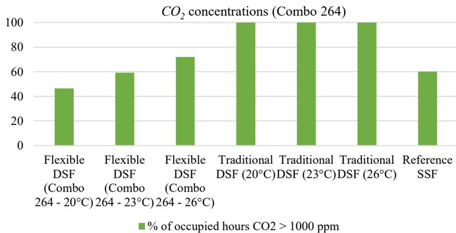
Figure 160: Percentage of occupied hours above the limit of 1000 ppm for the combination 264
