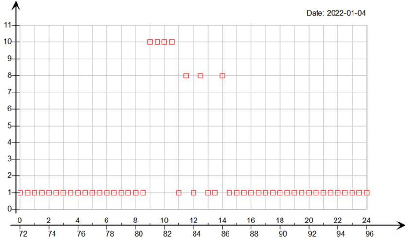
Figure 8: Variation of the flexible DSF configuration with the implementation of the control combination WC#16 in a typical winter day. (Output signal from IDA ICE). The configuration numbers are the ones illustrated in Table 2.
