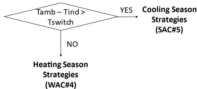
Figure 133: Selection of the cooling and heating season strategies for the *DSF* operations in function of the temperature difference between indoor and outdoor environment (active systems of the room turned on)
