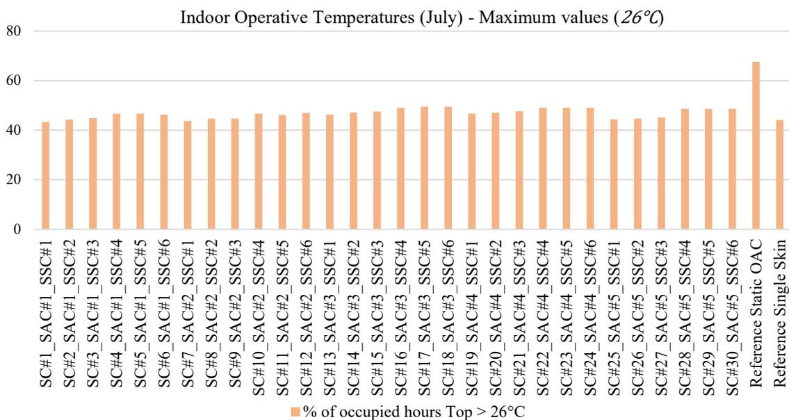
Figure 80: Percentages of occupied hours above 26°C for the different façade systems (July)
