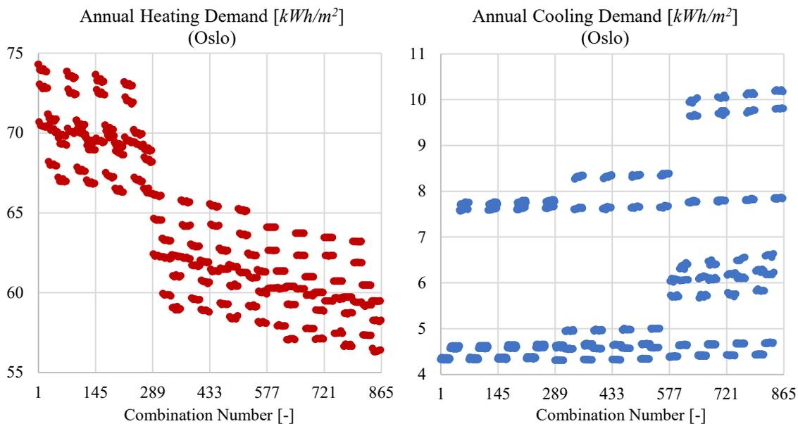
Figure 181: Heating (left) and cooling (right) energy need variation for the 864 different combinations in Oslo
