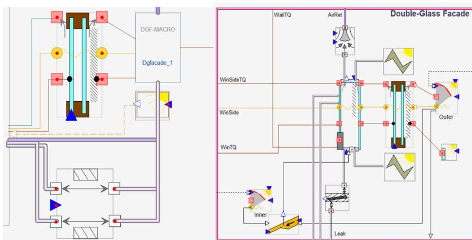
Figure 200: Schematic view of the DSF created on IDA ICE. On the left, it is visible the inner skin and the opening towards the zone, while on the right it is possible to see the ventilated cavity and the outer skin.
