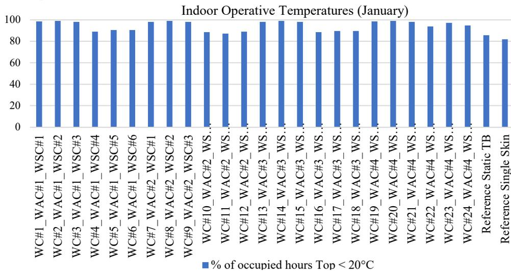
Figure 86: Percentage of occupied hours below  $20^{\circ}\text{C}$  for the different façade systems (January)
