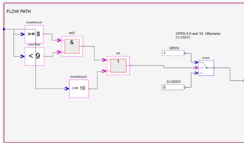
*Figure 206: Definition of the actuators state in function of the decision tree*
