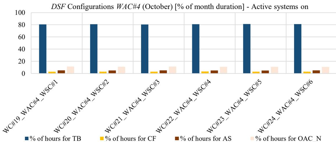
Figure 115: Percentages of hours in the month (October) in which the different DSF configurations have been adopted (active systems turned on) with WAC#4 as airflow control
