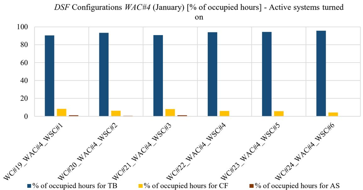
Figure 56: Percentages of occupied hours in the month (January) in which the different DSF configurations have been adopted (active systems turned on) with WAC#4 as airflow control
