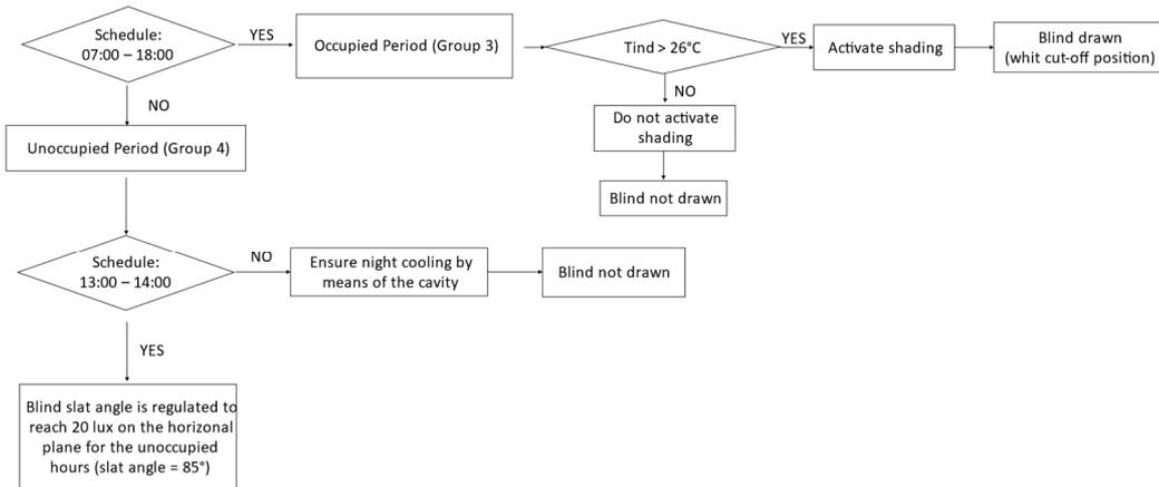
Figure 19: SSC#5 decision tree (Indoor air temperature activation + cut-off position)
