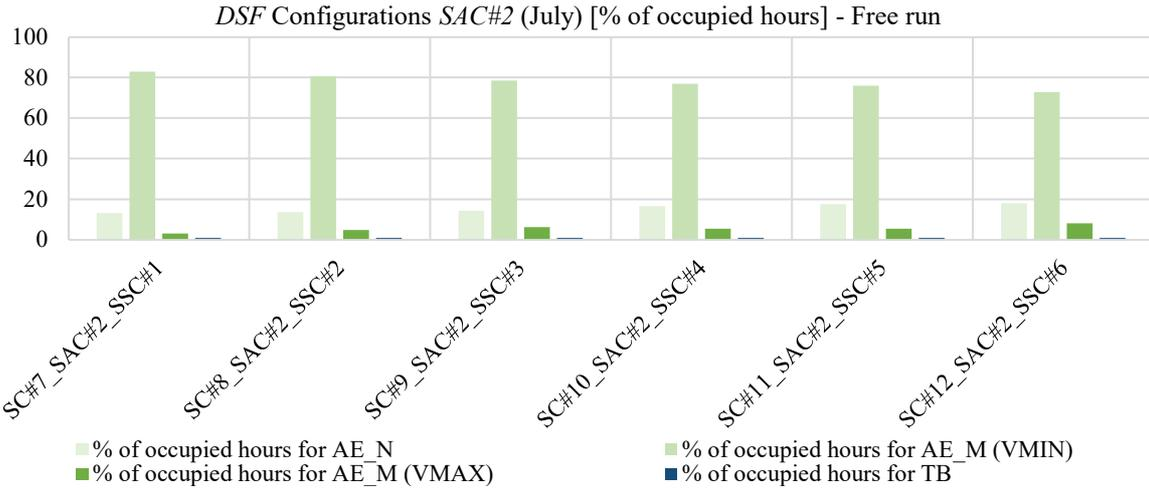
Figure 63: Percentages of occupied hours in the month (July) in which the different DSF configurations have been adopted (active systems turned off) with SAC#2 as airflow control
