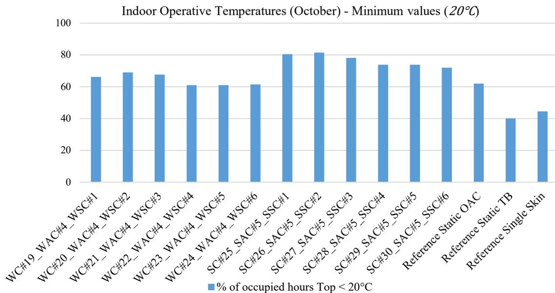
*Figure 126: Percentages of occupied hours below  $20^{\circ}\text{C}$  for the different façade systems (October)*
