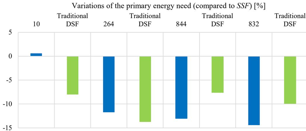
Figure 162: Variations (compared to SSF) of the primary energy need generated by the different combinations of values for the flexible DSF (green columns) and the traditional DSF (blue columns)
