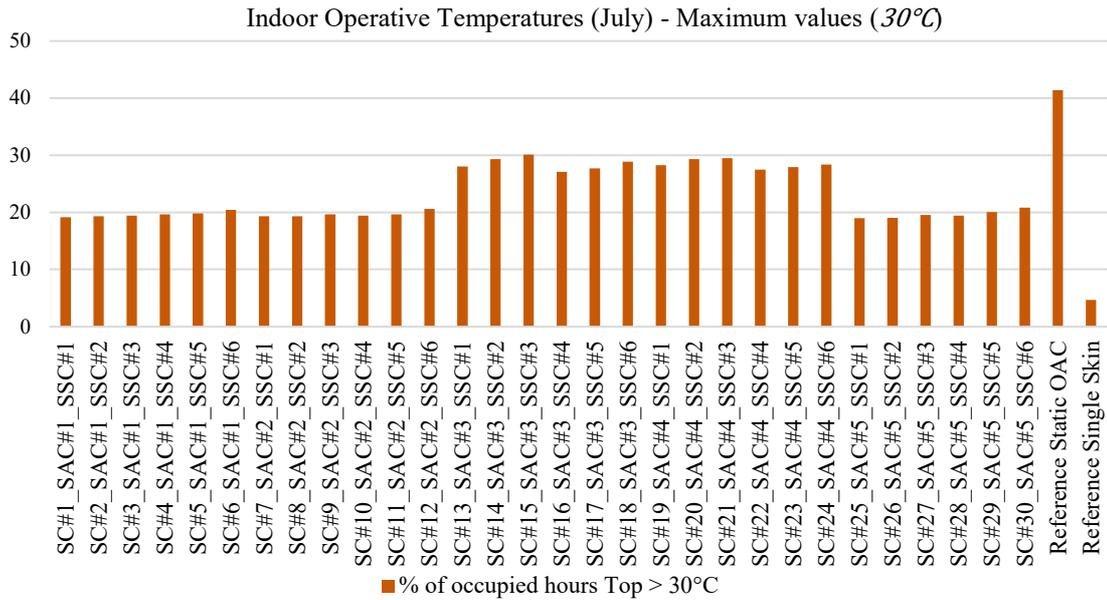
Figure 81: Percentages of occupied hours above 30°C for the different façade systems (July)
