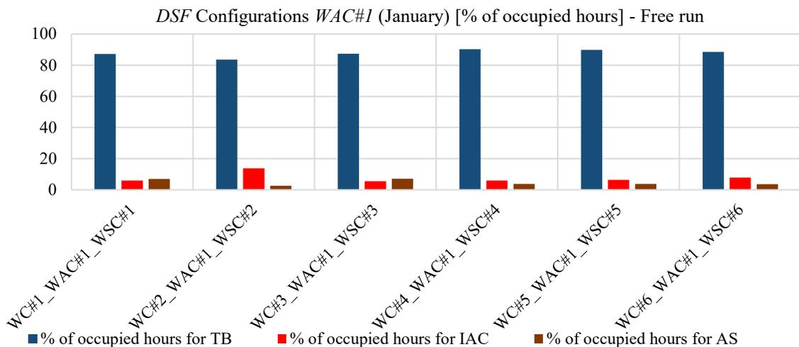
Figure 71: Percentages of occupied hours in the month (January) in which the different DSF configurations have been adopted (active systems turned off) with WAC#1 as airflow control
