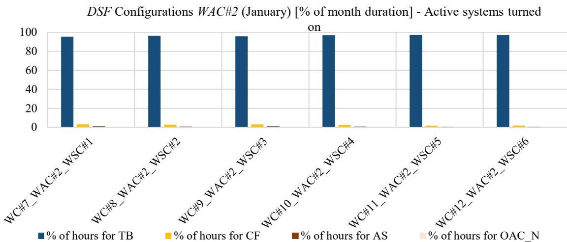
Figure 50: Percentages of hours in the month (January) in which the different DSF configurations have been adopted (active systems turned on) with *WAC#2* as airflow control
