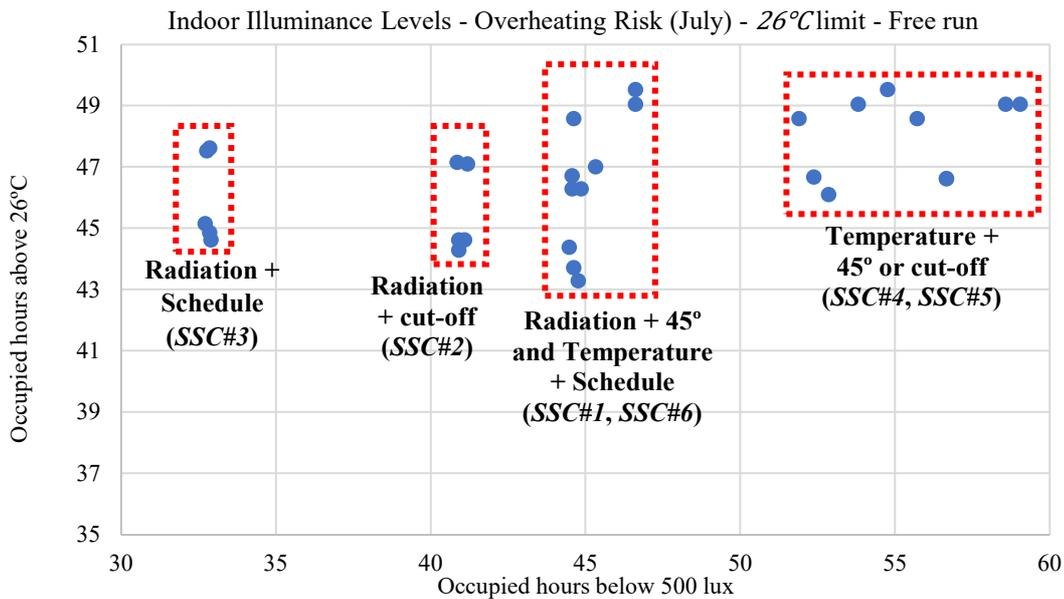
Figure 95: Relation between the percentages of occupied hours above 26°C and below 500 lux (July).
