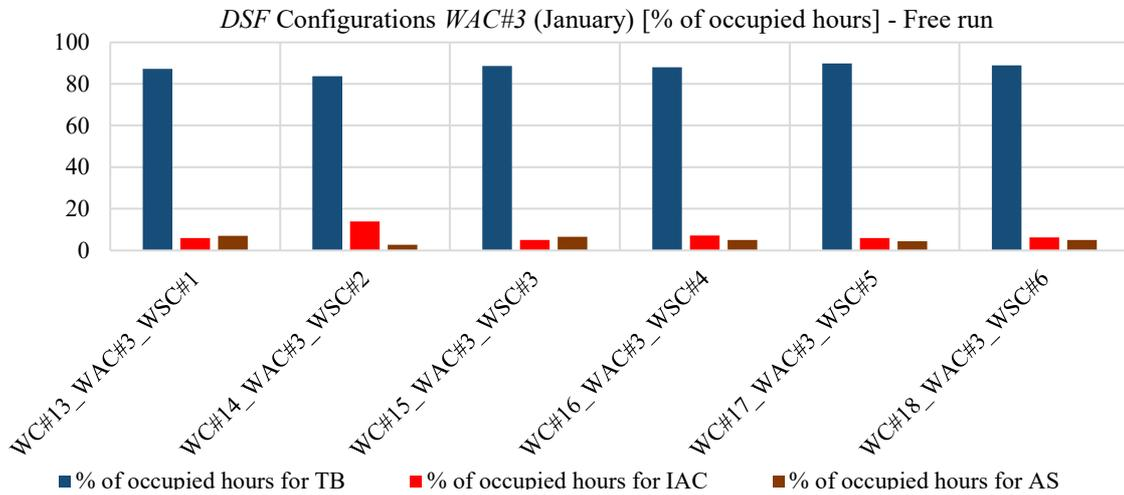
Figure 73: Percentages of occupied hours in the month (January) in which the different DSF configurations have been adopted (active systems turned off) with WAC#3 as airflow control
