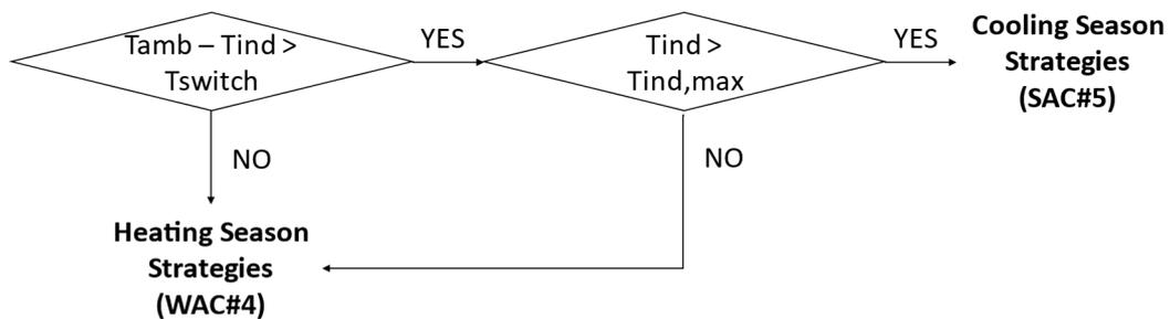
Figure 153: Selection of the cooling and heating season strategies for the *DSF* operations in function of the temperature difference between indoor and outdoor environment (active systems of the room turned off)
