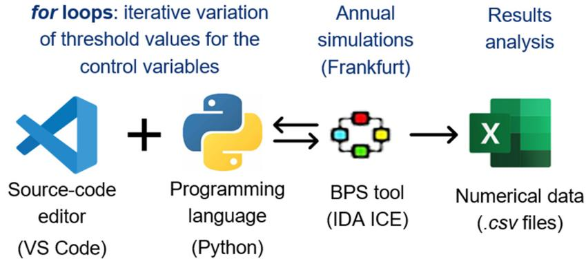
Figure 38: Parametric optimization process applied using the IDA Application Programming Interface
