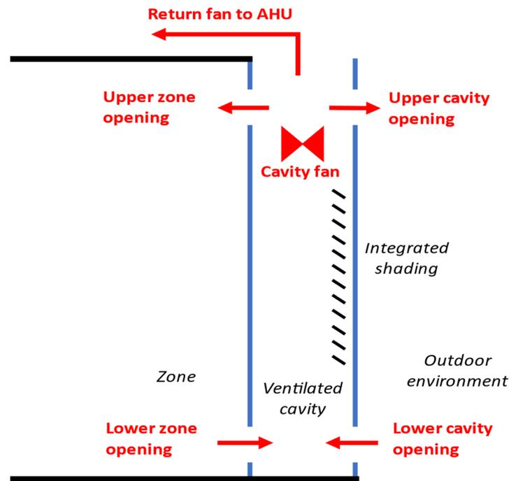
Figure 6: Functional scheme of the flexible DSF model with the different façade actuators
