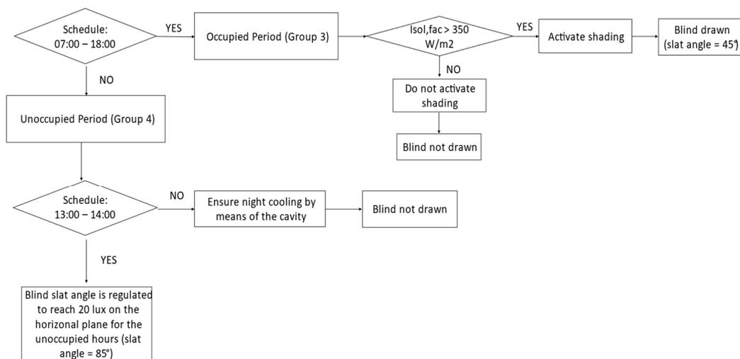
Figure 15: SSC#1 decision tree (Solar radiation activation + fixed slat angle)
