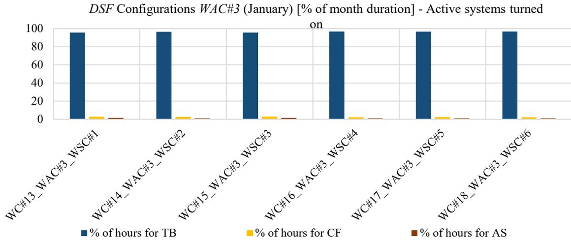
Figure 51: Percentages of hours in the month (January) in which the different DSF configurations have been adopted (active systems turned on) with WAC#3 as airflow control
