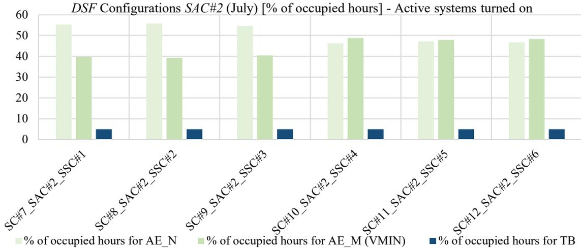
Figure 45: Percentages of occupied hours in the month (July) in which the different DSF configurations have been adopted (active systems turned on) with SAC#2 as airflow control
