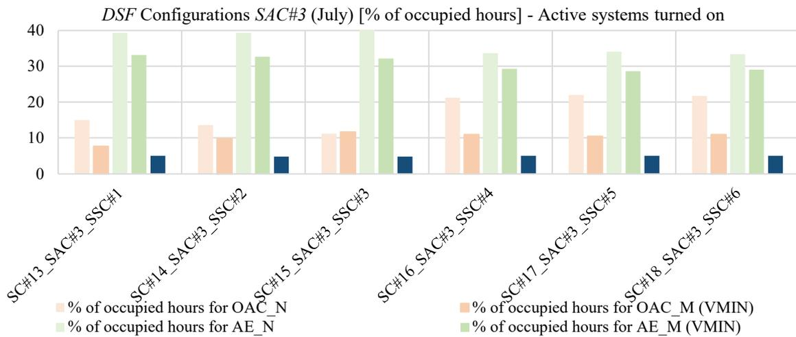
Figure 46: Percentages of occupied hours in the month (July) in which the different DSF configurations have been adopted (active systems turned on) with SAC#3 as airflow control
