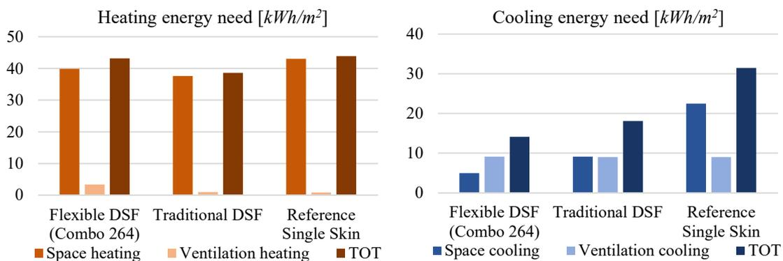
Figure 148: Heating (left) and cooling (right) energy need variation (Combo 264)
