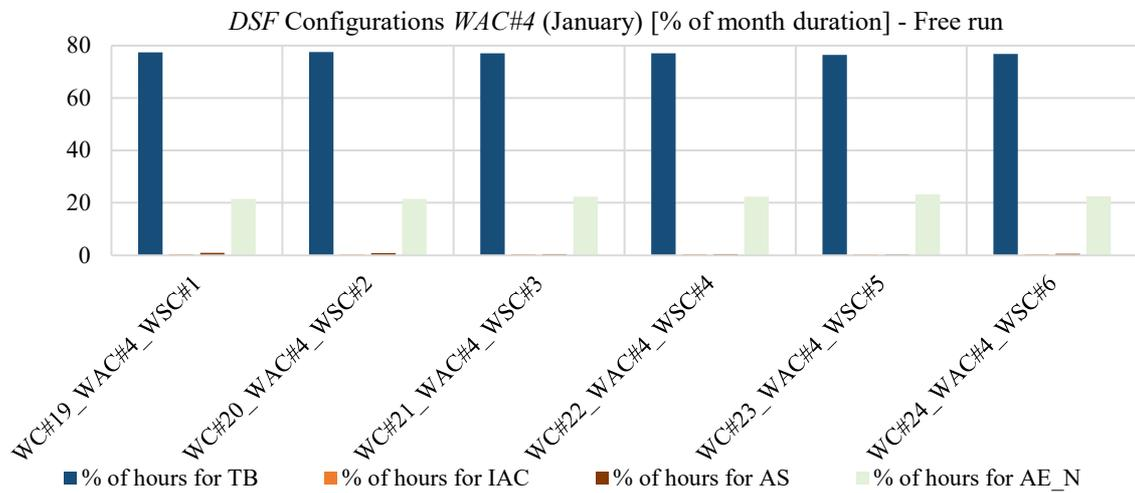
Figure 70: Percentages of hours in the month (January) in which the different DSF configurations have been adopted (active systems turned off) with WAC#4 as airflow control
