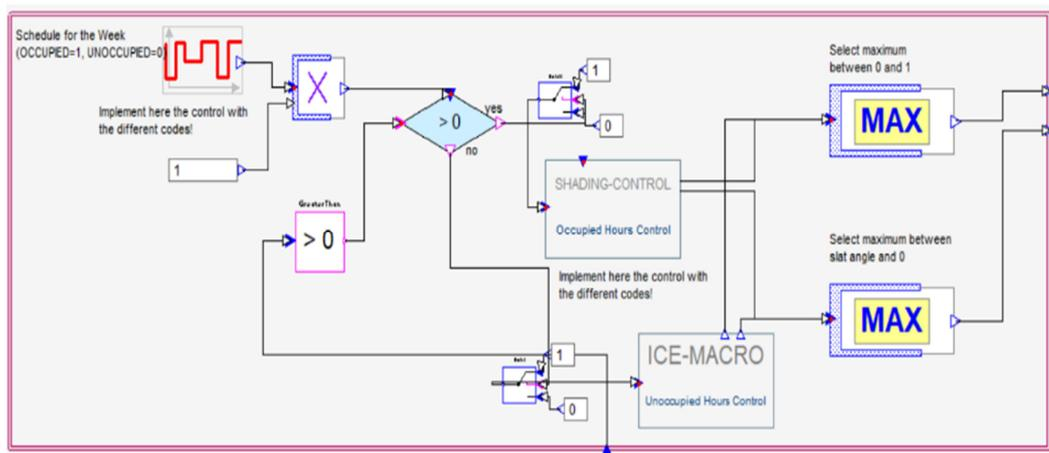
Figure 210: Distinction between the operating strategies for the shading system during the weekdays
