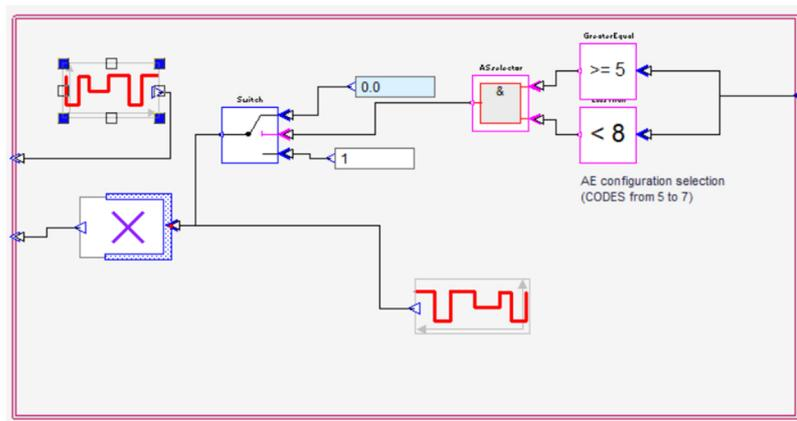
Figure 209: The Control Macro for the supply fan of the AHU
