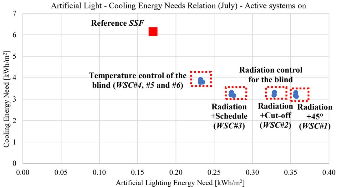
Figure 92: Relation between the artificial lighting and cooling energy needs of the room with the adoption of the different façade system (July).
