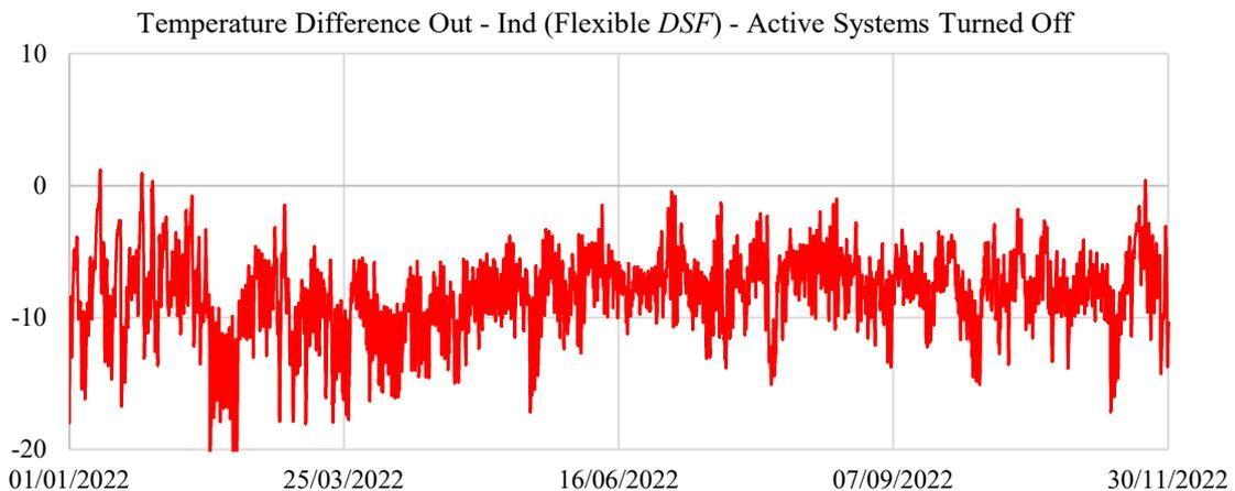
Figure 154: Variation through of the air temperature difference between the outdoor and the indoor environments, if the free running configuration of the model is considered (the flexible *DSF* system is considered)
