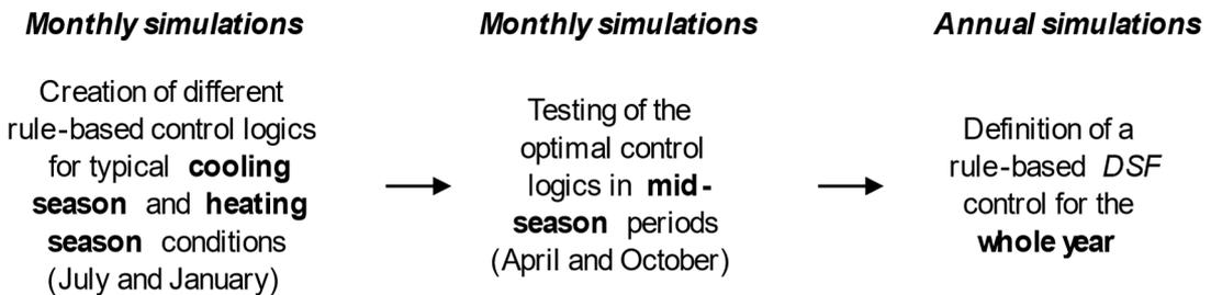
*Figure 4: The 3 different phases of the simulation workflow development for the creation of the rule based DSF control for the whole year*
