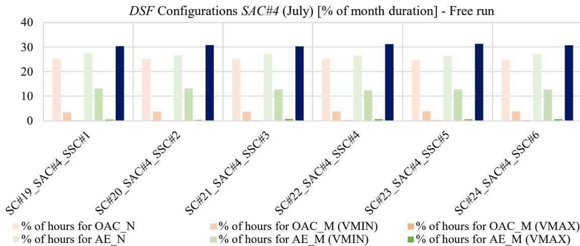
Figure 60: Percentages of hours in the month (July) in which the different DSF configurations have been adopted (active systems turned off) with SAC#4 as airflow control
