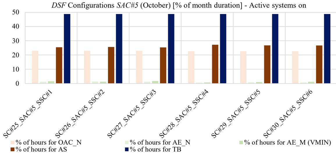
Figure 113: Percentages of hours in the month (October) in which the different DSF configurations have been adopted (active systems turned on) with SAC#5 as airflow control
