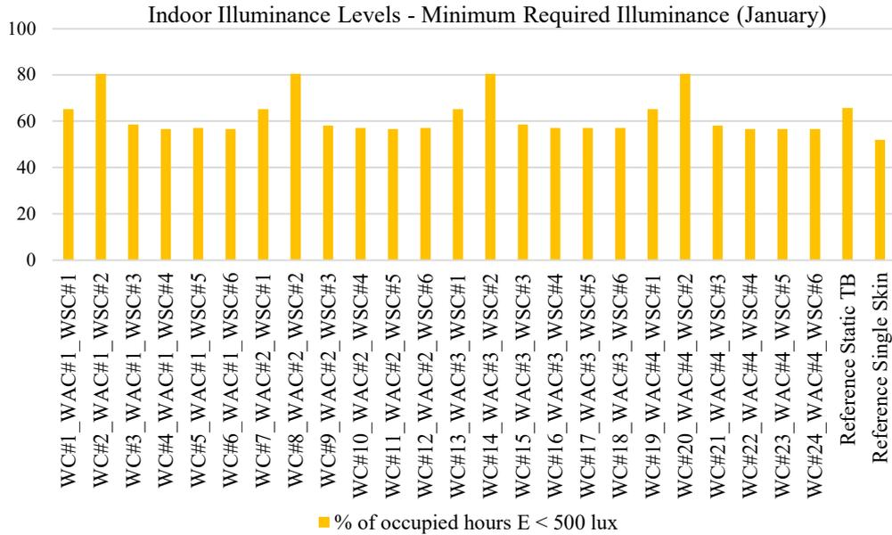
Figure 89: Percentage of occupied hours below the limit of 500 lux (January)
