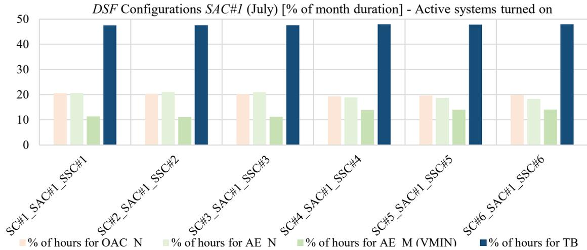
Figure 39: Percentages of hours in the month (July) in which the different DSF configurations have been adopted (active systems turned on) with SAC#1 as airflow control
