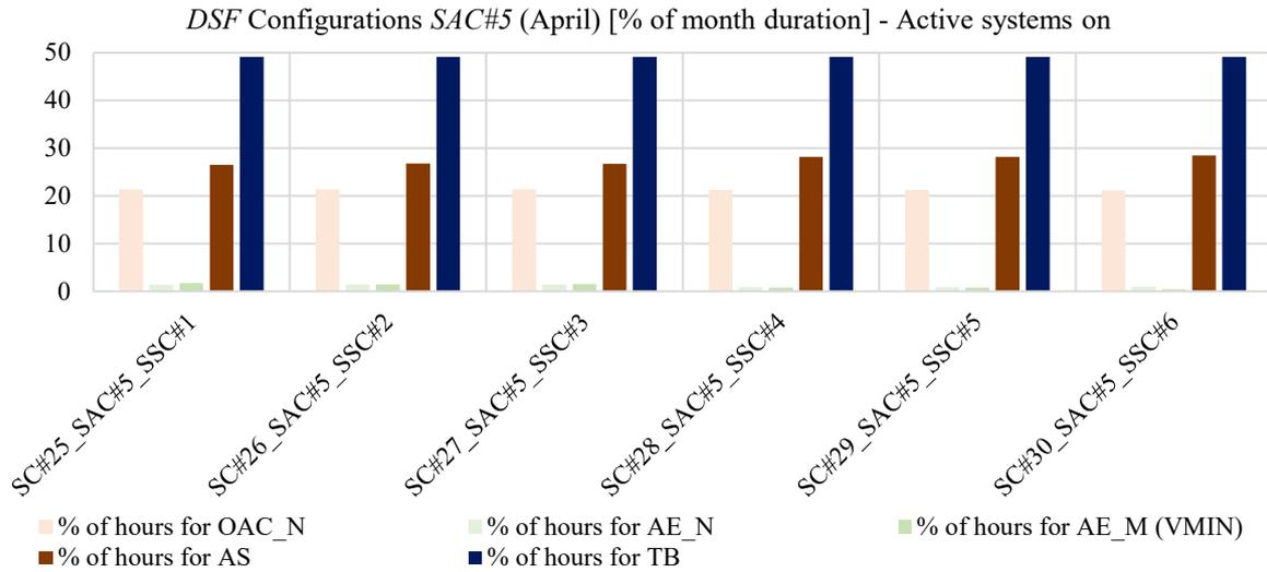
Figure 96: Percentages of hours in the month (April) in which the different *DSF* configurations have been adopted (active systems turned on) with *SAC#5* as airflow control
