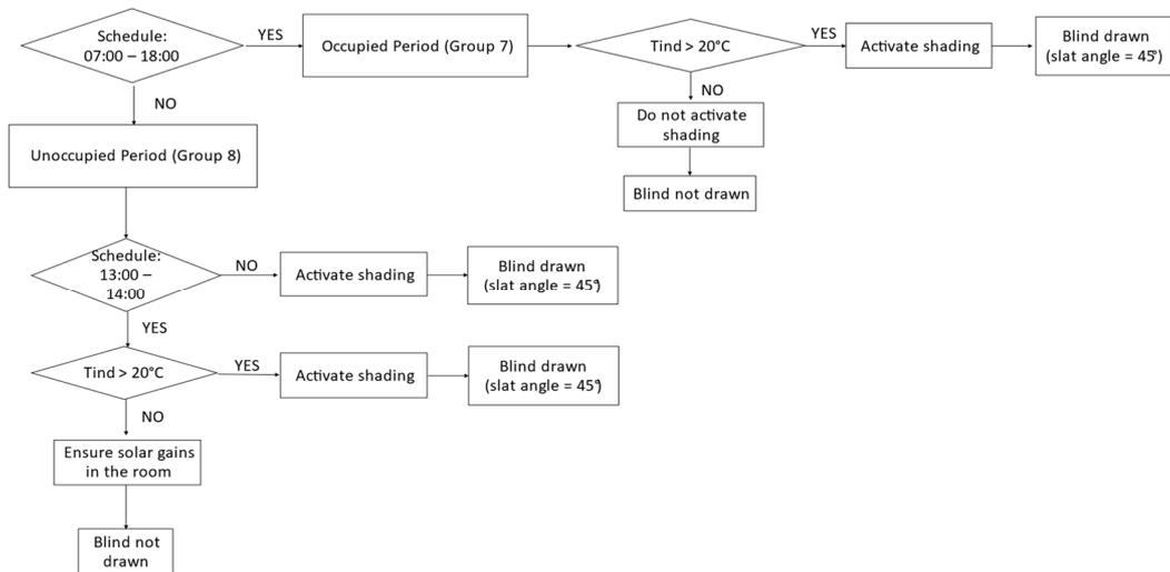
Figure 28: WSC#4 decision tree (Indoor air temperature activation + fixed slat angle)
