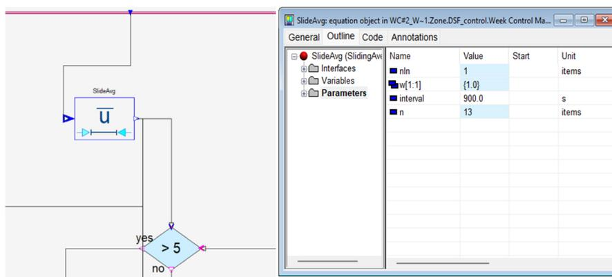
Figure 212: The Sliding Average module (left) and the definition of the interval parameter (right) in the Outline view
