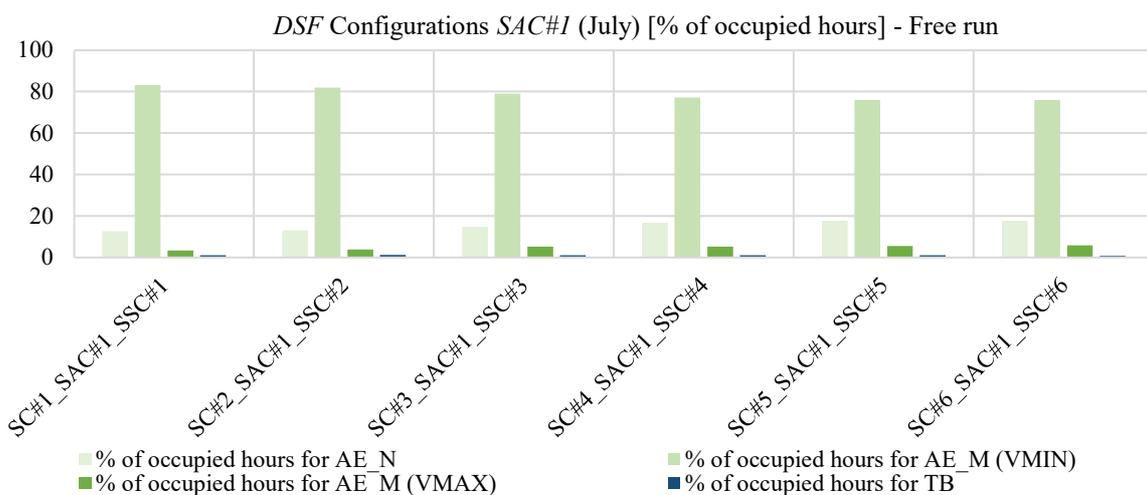
Figure 62: Percentages of occupied hours in the month (July) in which the different DSF configurations have been adopted (active systems turned off) with SAC#1 as airflow control
