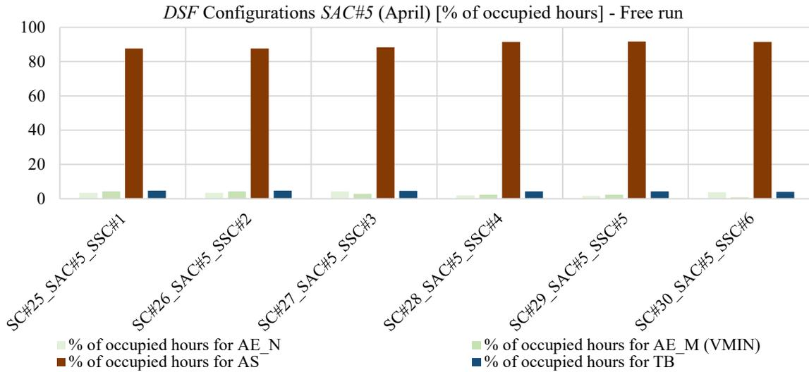
Figure 104: Percentages of occupied hours in the month (April) in which the different DSF configurations have been adopted (active systems turned off) with SAC#5 as airflow control
