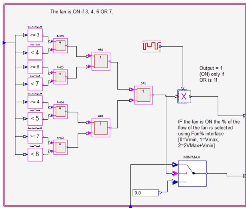
*Figure 207: Definition of the fan configuration (on/off) and the related air flow (min/mx) inside the cavity fan Control Macro*
