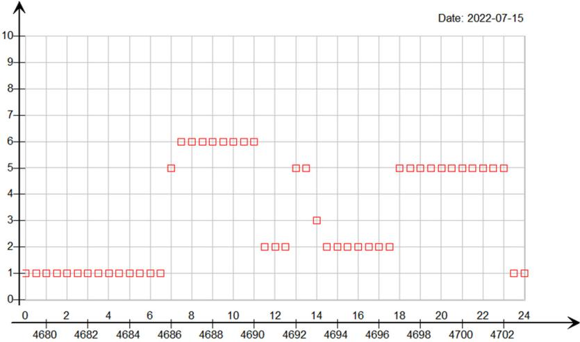
Figure 7: Variation of the flexible DSF configurations with the implementation of the control combination SC#22 in a typical summer day (Output signal from IDA ICE). The configuration numbers are the ones illustrated in Table 2.
