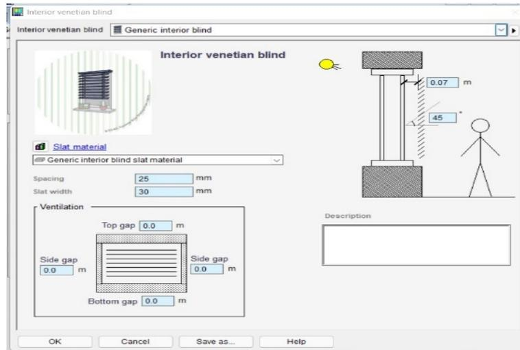
Figure 199: Definition of the shading system properties (in this case a venetian blind): materials, slat angle, distances.
