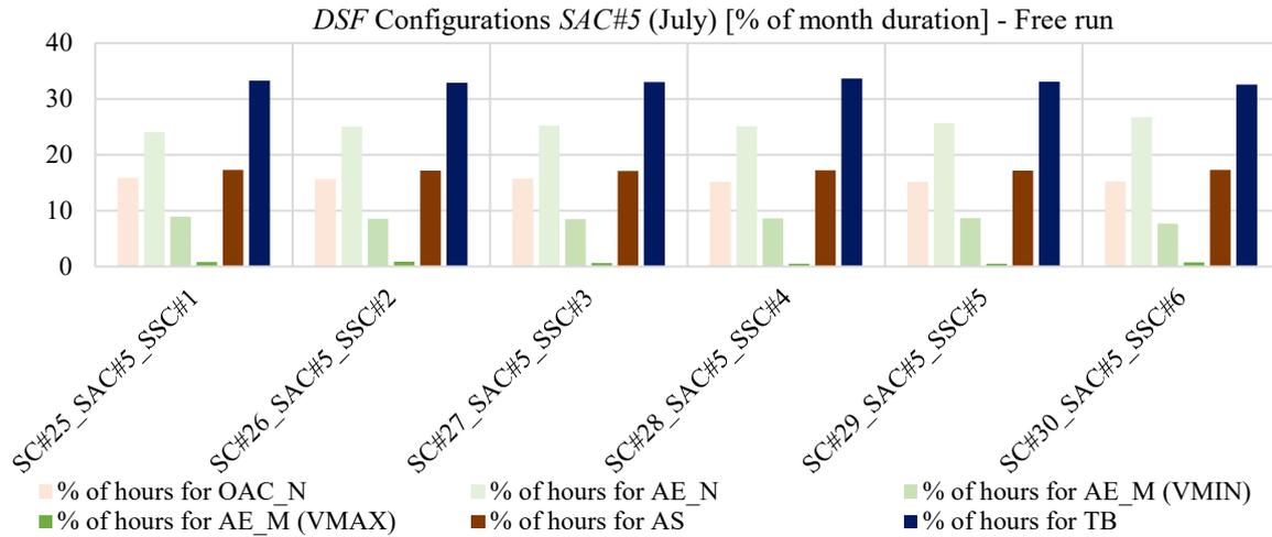
Figure 61: Percentages of hours in the month (July) in which the different DSF configurations have been adopted (active systems turned off) with SAC#5 as airflow control
