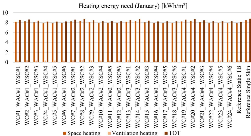
Figure 78: Heating energy requirements for the different façade systems (January)
