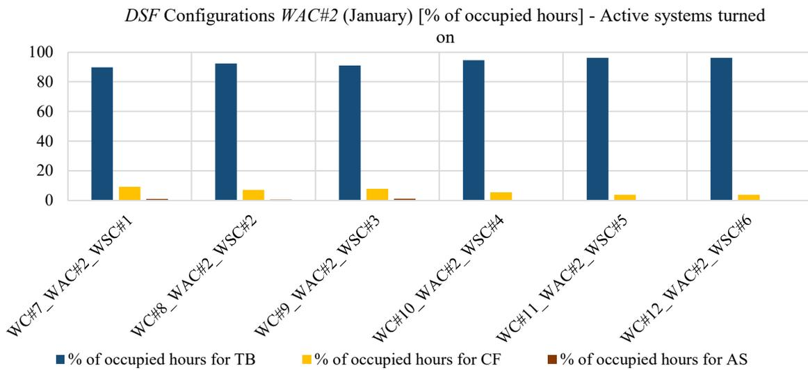
Figure 54: Percentages of occupied hours in the month (January) in which the different DSF configurations have been adopted (active systems turned on) with WAC#2 as airflow control
