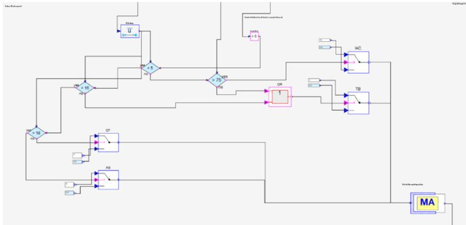
Figure 202: Example of decision tree for the cavity air flows built in IDA ICE
