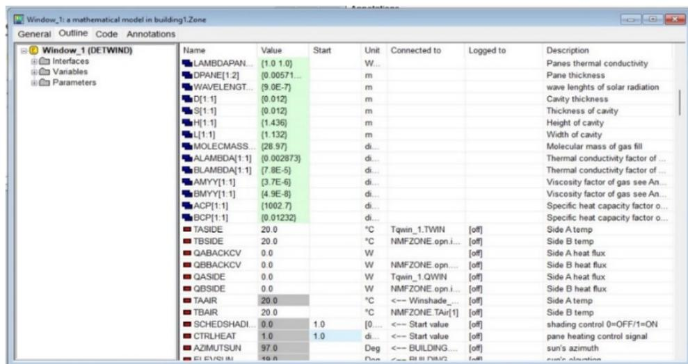
Figure 191: Mathematical model of a window in IDA ICE: list of interfaces, variables and parameter in the Outline tab of the element.
