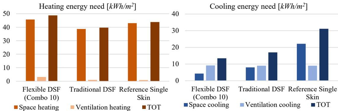
Figure 138: Heating (left) and cooling (right) energy need variation (Combo 10)
