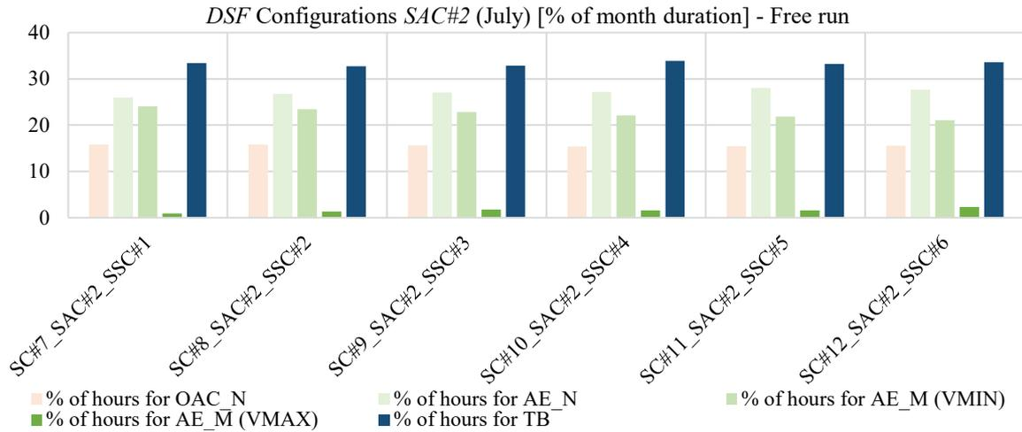
Figure 58: Percentages of hours in the month (July) in which the different DSF configurations have been adopted (active systems turned off) with SAC#2 as airflow control
