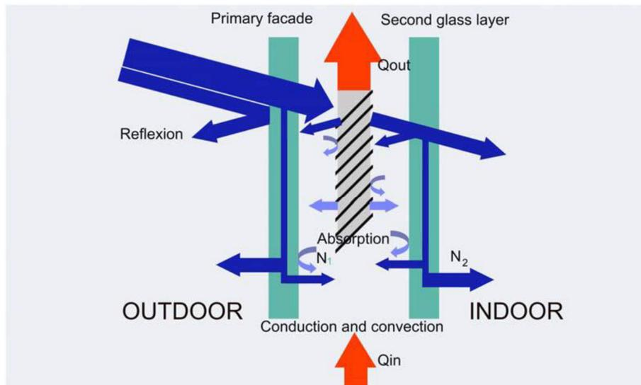
*Figure 194: Structure of a DSF, with the different components of the system: primary façade (outer skin), second glass layer (inner skin), cavity and integrated solar shading device [61].*
