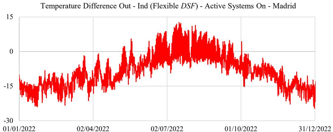
*Figure 164: Variation through of the air temperature difference between the outdoor and the indoor environments, if the active systems of the room are on (the flexible DSF system is considered) in Madrid*
