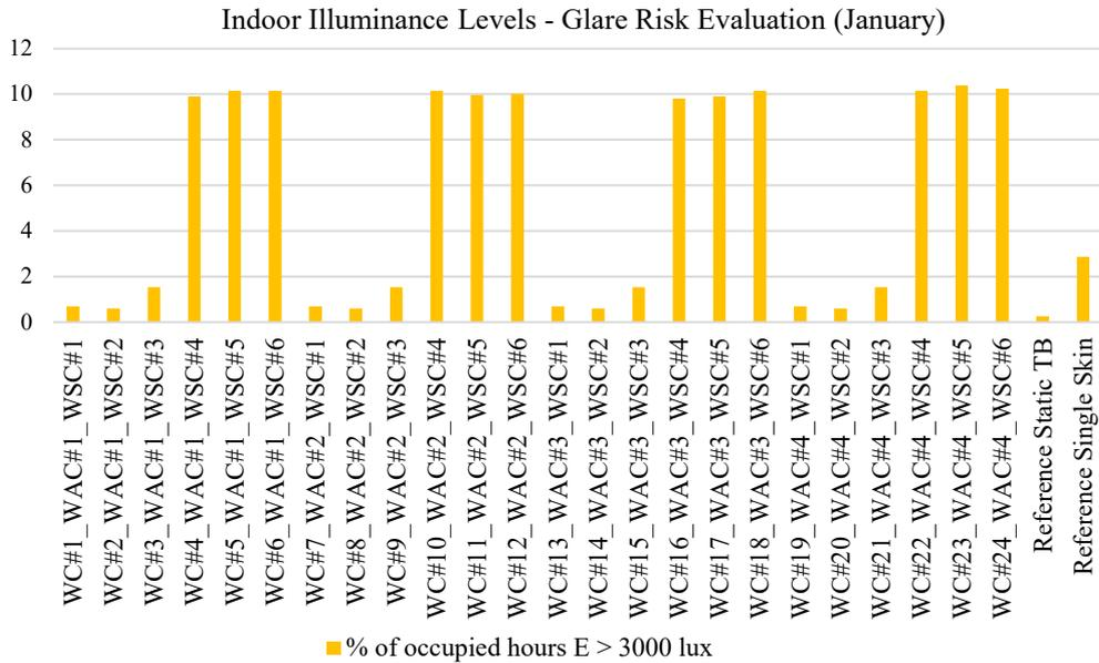
Figure 90: Percentage of occupied hours above the limit of 3000 lux (January)
