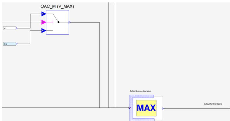
Figure 205: Application of the Max module for the definition of the output of the Macro
