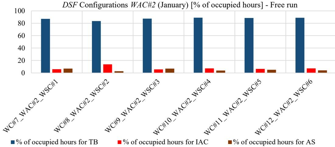
Figure 72: Percentages of occupied hours in the month (January) in which the different DSF configurations have been adopted (active systems turned off) with WAC#2 as airflow control
