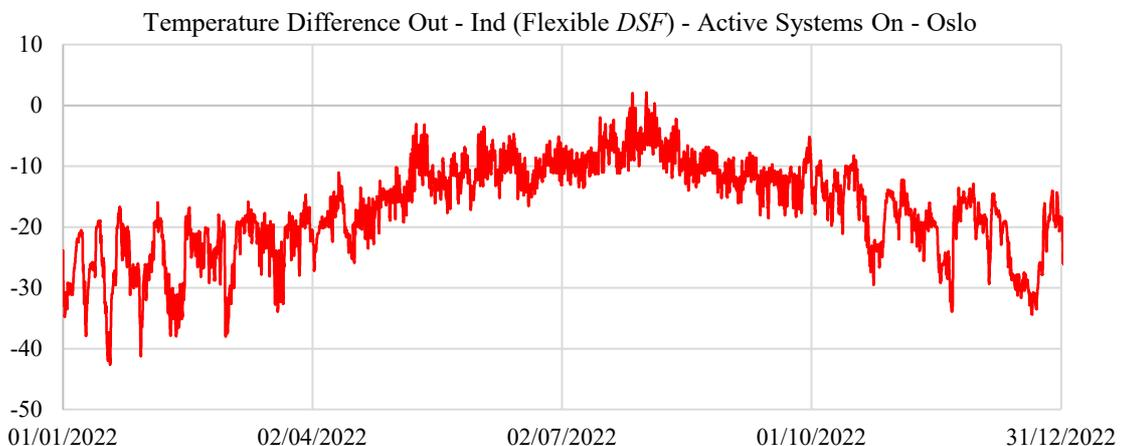
Figure 180: Variation through of the air temperature difference between the outdoor and the indoor environments, if the active systems of the room are on (the flexible DSF system is considered) in Oslo
