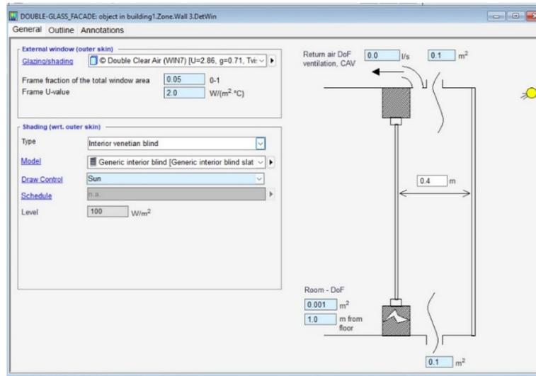
Figure 198: The form referred to the double glass façade component: here it is possible to define the properties of the external skin, the cavity and the integrated shading system.
