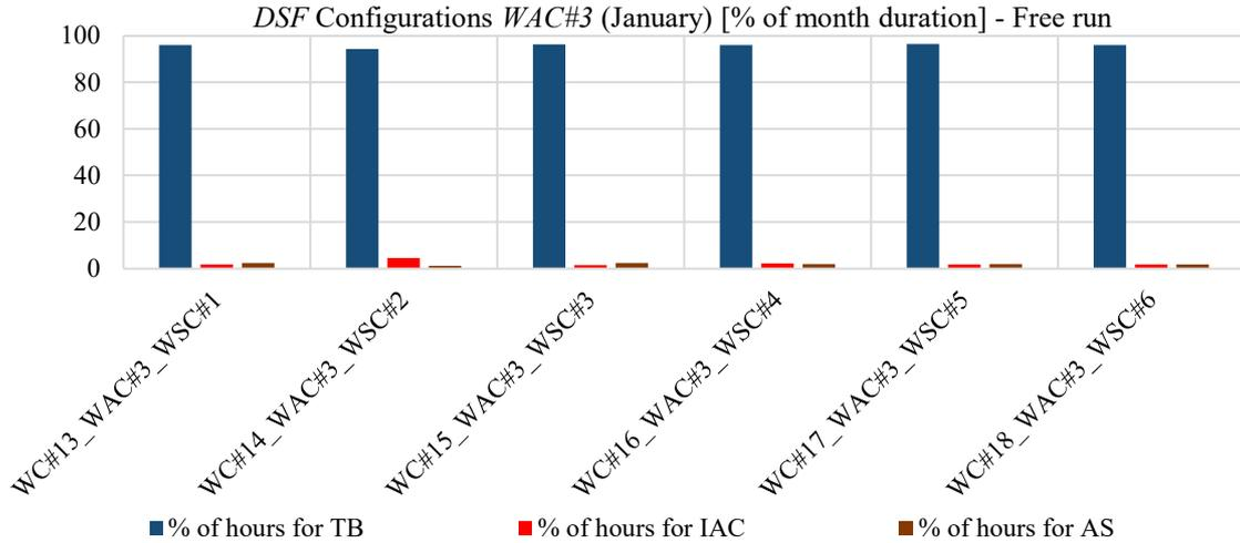
Figure 69: Percentages of hours in the month (January) in which the different DSF configurations have been adopted (active systems turned off) with WAC#3 as airflow control
