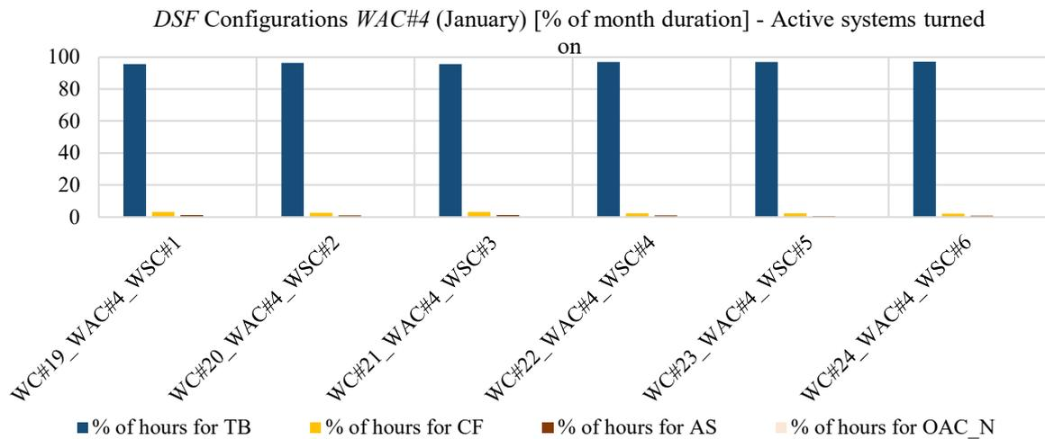
Figure 52: Percentages of hours in the month (January) in which the different DSF configurations have been adopted (active systems turned on) with WAC#4 as airflow control
