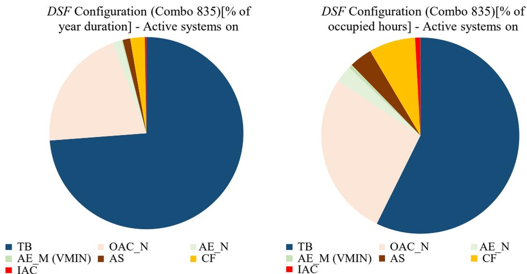
Figure 188: Flexible DSF configuration through the year for combo 835 in Madrid: overall month duration (left) and occupied hours (right)
