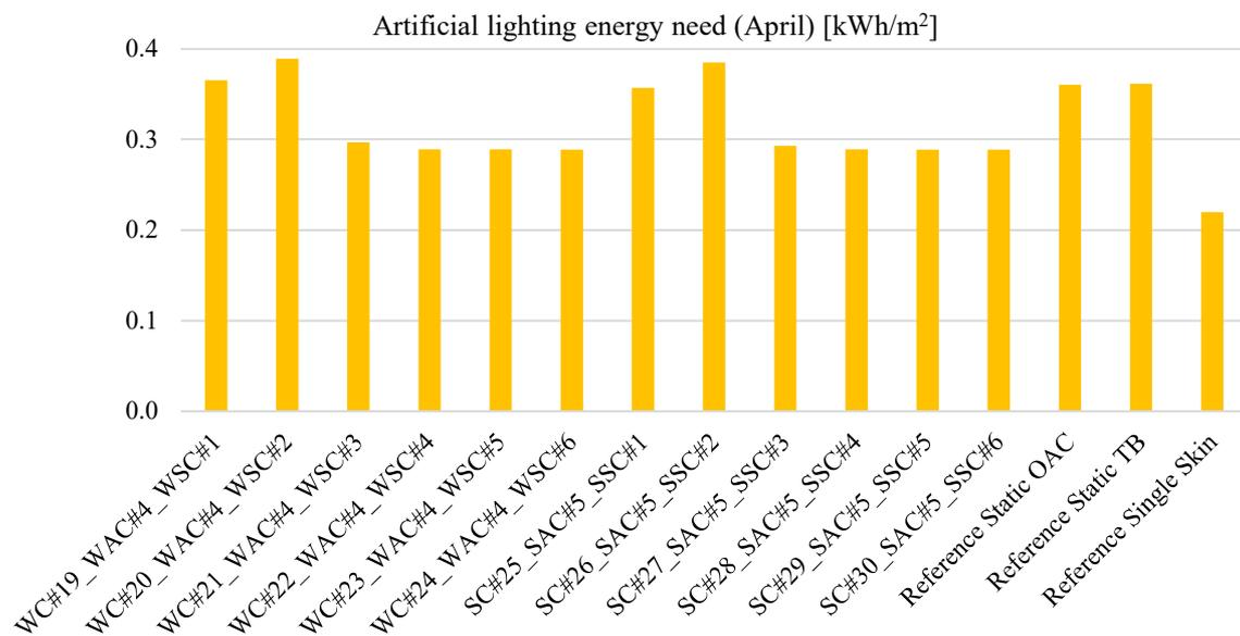
Figure 102: Artificial lighting energy requirements for the different façade systems (April)
