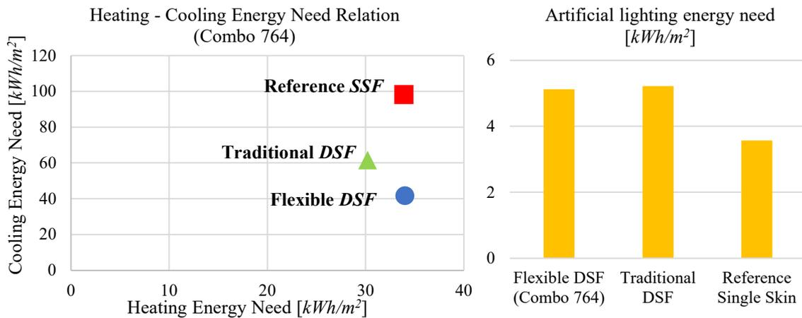
Figure 169: Relation between the heating and the cooling energy needs (left) for Combo 764 and related energy needs for artificial lighting in Madrid (right).
