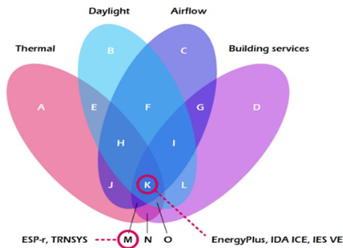
Figure 193: Intersection of all the different domains for different BPS tools [9].
