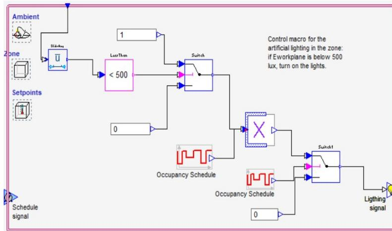
Figure 211: Definition of the control macro for the artificial lighting system of the room
