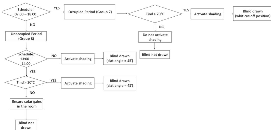
Figure 29: WSC#5 decision tree (Indoor air temperature activation + cut-off position)
