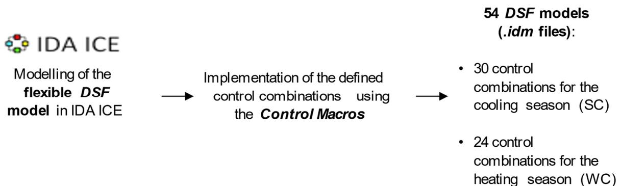
*Figure 31: DSF modelling workflow in IDA ICE for the creation of the different combinations of control for the flexible DSF for the heating and cooling season*
