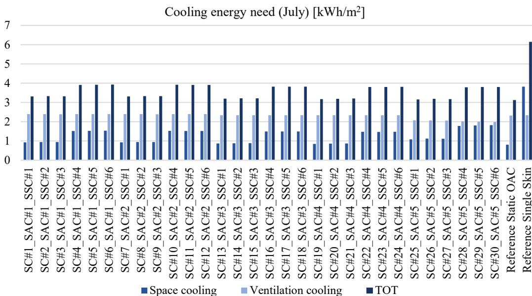
*Figure 76: Cooling energy requirements for the different façade systems (July)*
