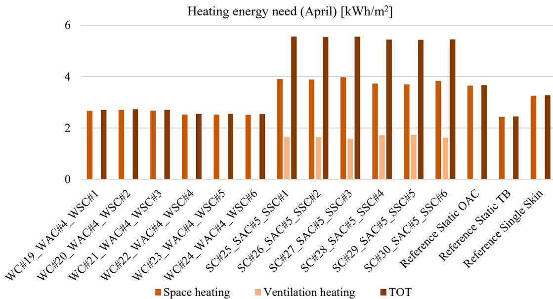
Figure 100: Heating energy requirements for the different façade systems (April)
