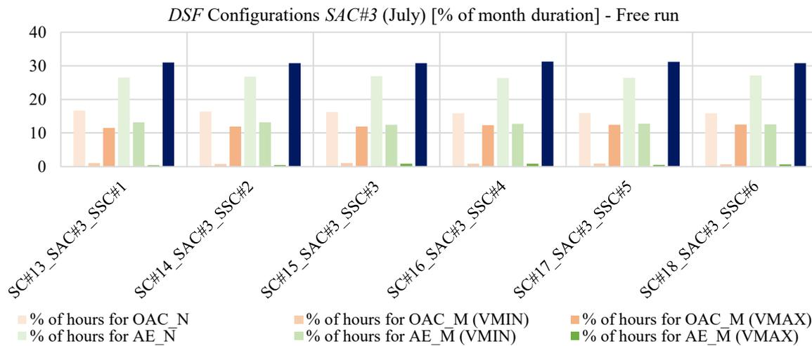
Figure 59: Percentages of hours in the month (July) in which the different DSF configurations have been adopted (active systems turned off) with SAC#3 as airflow control
