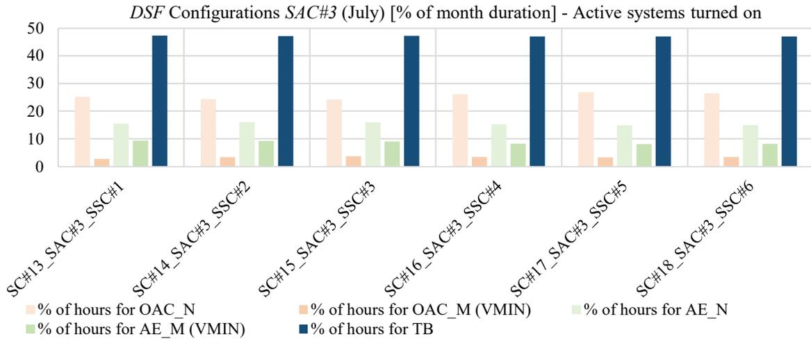
Figure 41: Percentages of hours in the month (July) in which the different DSF configurations have been adopted (active systems turned on) with SAC#3 as airflow control
