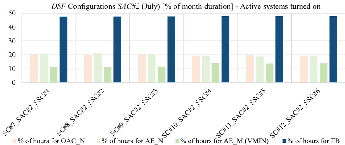
Figure 40: Percentages of hours in the month (July) in which the different DSF configurations have been adopted (active systems turned on) with SAC#2 as airflow control
