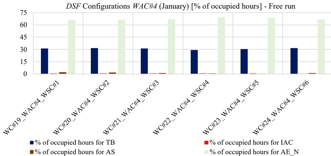
Figure 74: Percentages of occupied hours in the month (January) in which the different DSF configurations have been adopted (active systems turned off) with WAC#4 as airflow control
