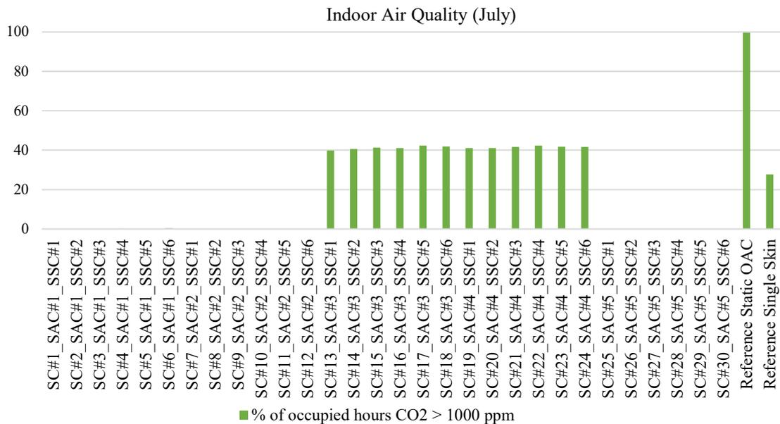
Figure 83: Percentages of occupied hours above 1100 ppm for the different façade systems (July)
