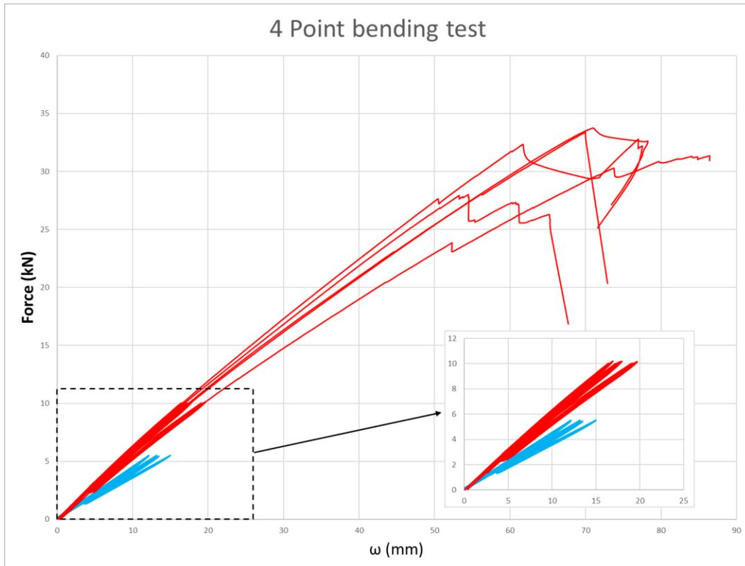
*Fig. 35: Load-deflection curves of the large-scale DLT panels.*
