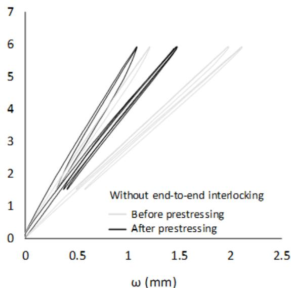
Fig. 27: Load-deflection curves of the small-scale DLT panels without end-to-end interlocking.
