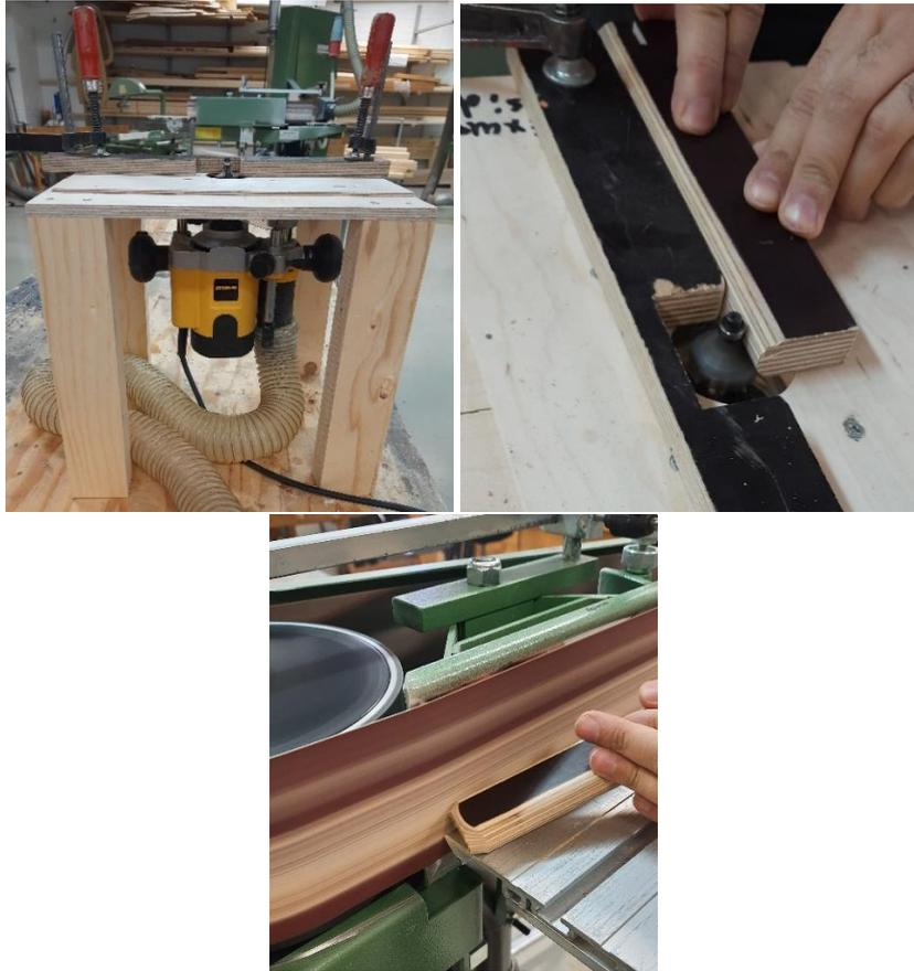
*Fig. 9: (a) jig used to create the rounded shape of the tenons, (b) procedure to create the rounded shape of the tenons, (c) procedure to create the smooth end to the tenons.*
