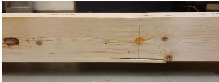
*Fig. 33: Bending failure D.*
