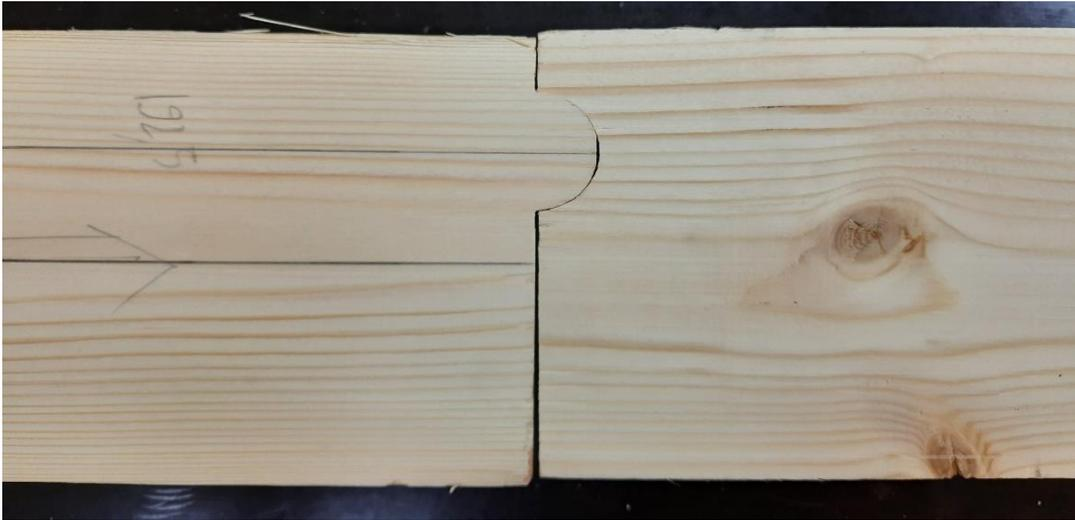
*Fig. A4: Mortise-tenon rounded shape interlocking pattern*
