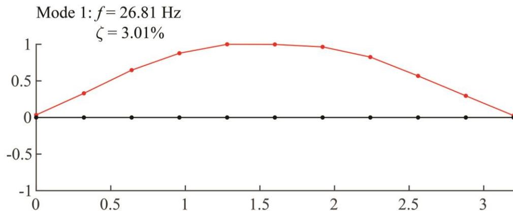
*Fig. A13: The first vibration mode of specimen A after prestressing.*
