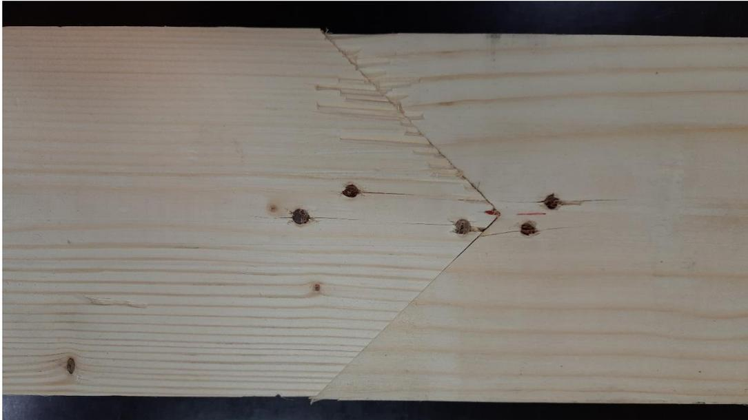
*Fig. A7: Mortise-tenon full board triangular shape interlocking pattern.*
