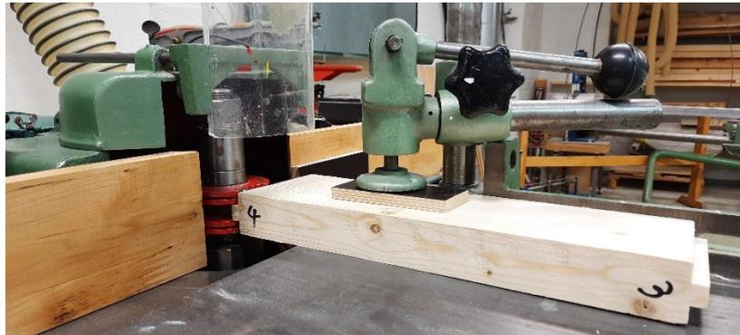
*Fig. 7: table router processing to create mortise and tenon shape (in the picture salvaged board with tenon shape).*
