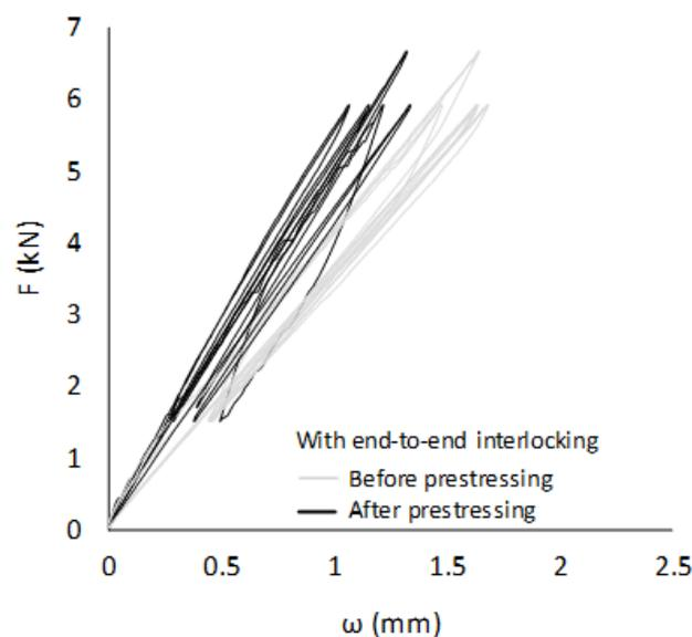
Fig. 26: Load-deflection curves of the small-scale DLT panels with end-to-end interlocking.
