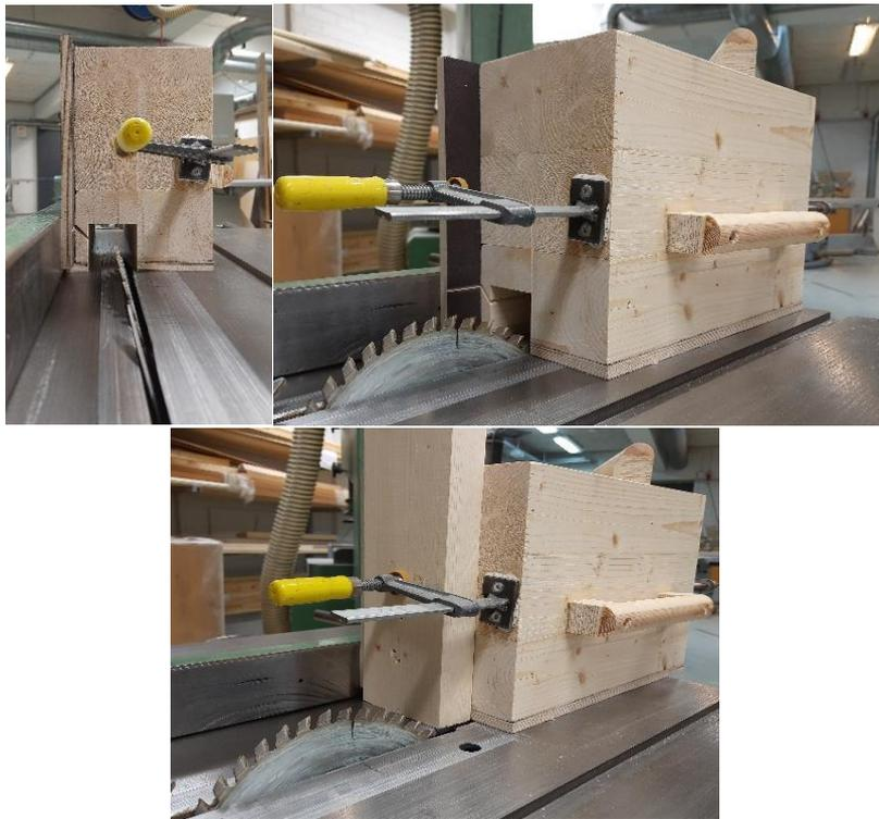
*Fig. A8: Jig used to cut the full board triangular shape interlocking pattern.*
