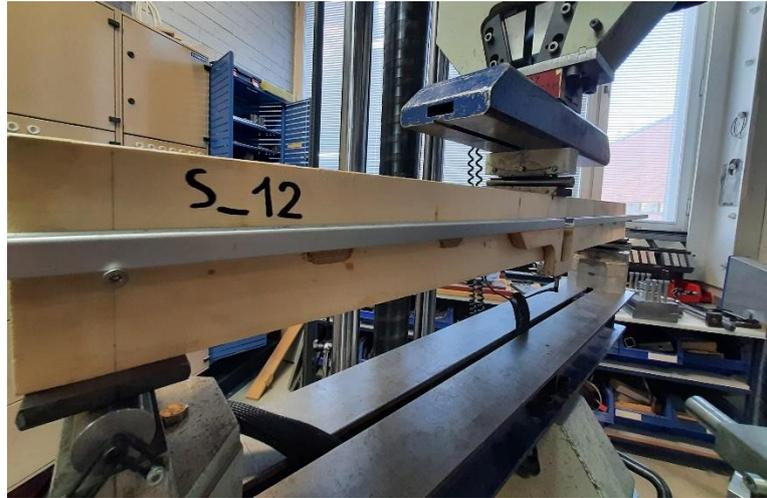
Fig. 12: Specimen S\_12 with end-to-end interlocking ready to be tested.
