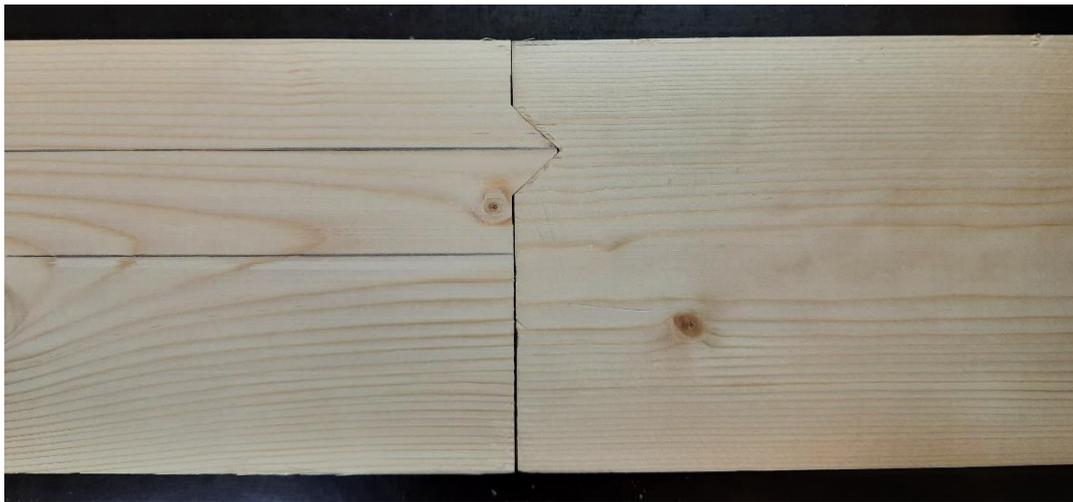
*Fig. A3: Mortise-tenon triangular shape interlocking pattern.*
