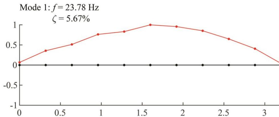
Fig. A18: The first vibration mode of specimen D before prestressing.
