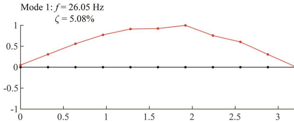
*Fig. A20: The first vibration mode of specimen E before prestressing.*
