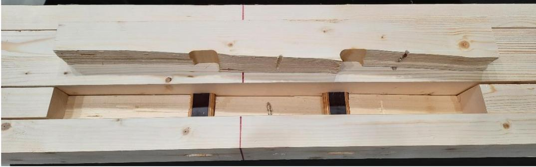
*Fig. 37: breaking of the salvaged timber board*
