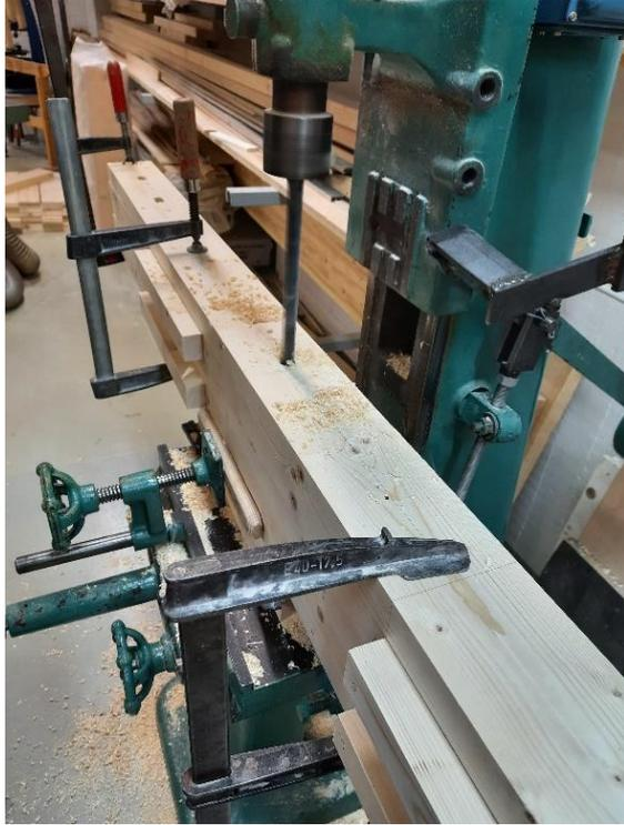
*Fig.20: Drilling procedure to make the holes for the plywood tenons.*
