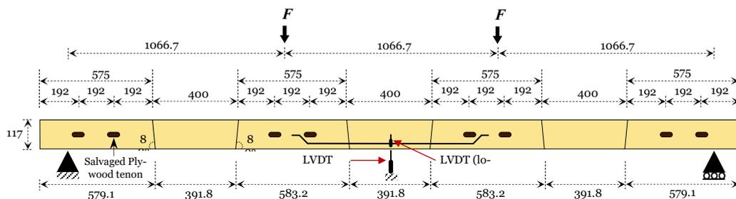
Fig. 19: Dimension of the salvaged timber elements in the large-scale DLT panels and the four-point bending test set-up. Dimensions in mm.
