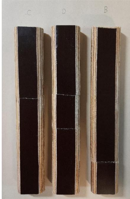
*Fig. 45: Failure mode of the tenons in the disassembled specimens, C D B respectively.*
