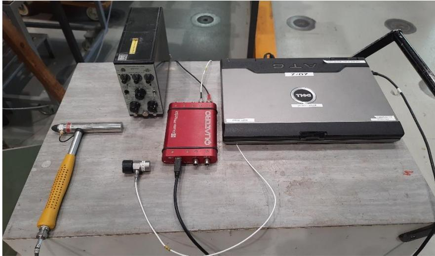
*Fig. 22: Tools used for the vibration test.*
