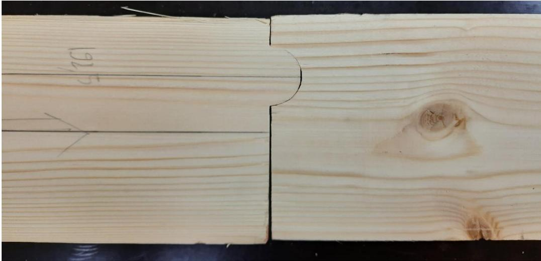
*Fig. A4: Mortise-tenon rounded shape interlocking pattern*
