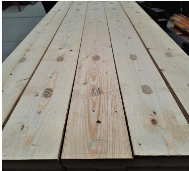
*Fig.4: Final pattern of the wooden dowels.*
