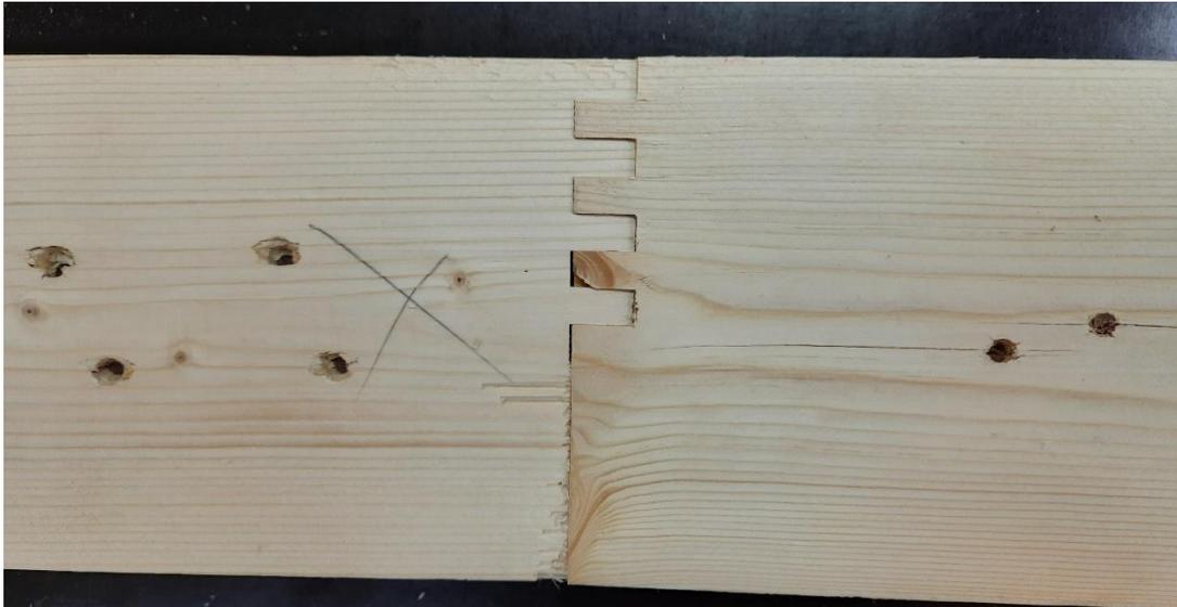
*Fig. A6: Finger joint interlocking pattern*
