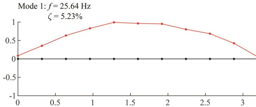
Fig. A17: The first vibration mode of specimen C after prestressing.
