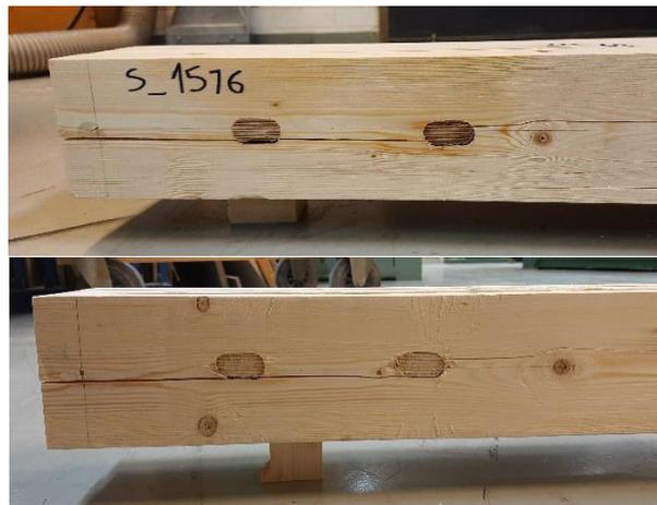
*Fig. 34: (a) Shear failure E, (b) shear failure F.*
