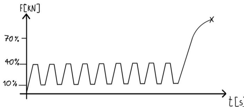
Fig. 24: (a) loading procedure for the four-point bending test without the piece in the middle (Stage N), (b) loading procedure for the four-point bending test with the piece in the middle (Stage Y).
