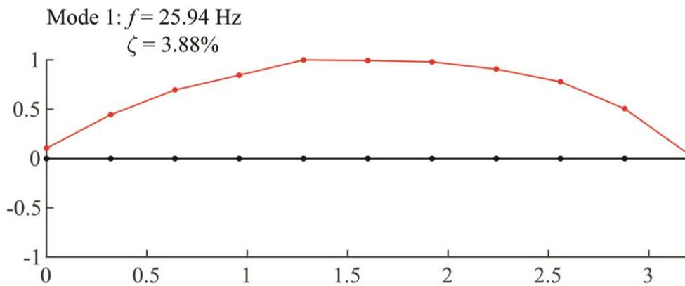
Fig. A15: The first vibration mode of specimen B after prestressing.
