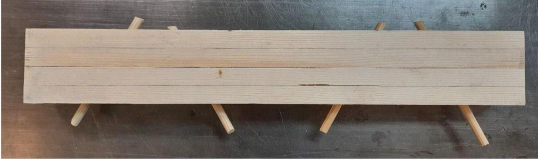
*Fig.3: Prototype with inclined dowels.*
