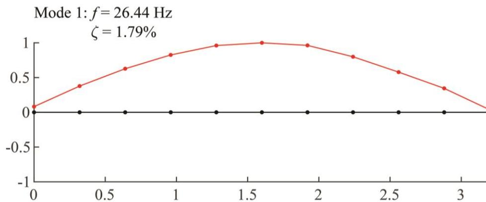
Fig. A19: The first vibration mode of specimen D after prestressing.
