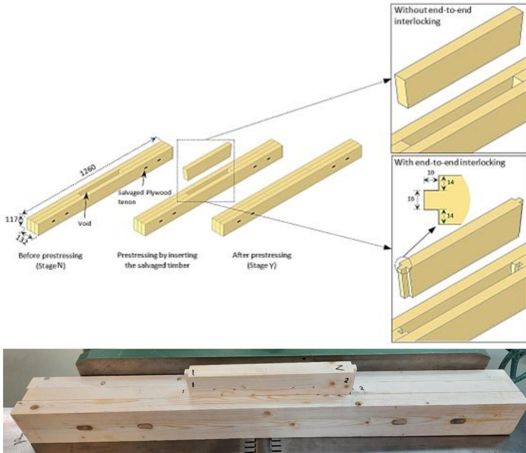
Fig.6: Configuration of the small-scale DLT panels before and after prestressing. Dimensions in mm.
