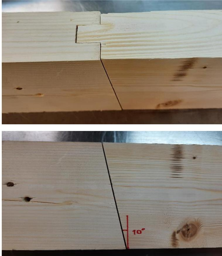
*Fig. A9: Vertical profiled mortise tenon interlocking pattern.*
