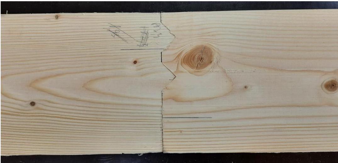
*Fig. A5: Double mortise-tenon triangular shape interlocking pattern.*
