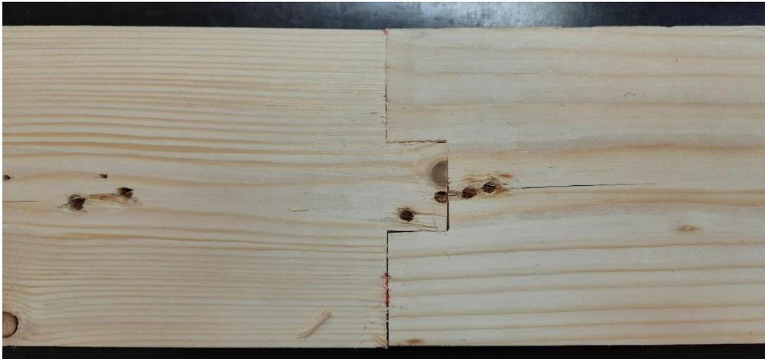
*Fig. A2: Mortise-tenon rectangular shape interlocking pattern.*
