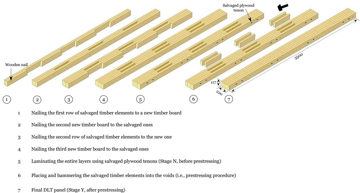
Fig. 18: Fabrication steps of the large-scale DLT panels. Dimensions in mm.
