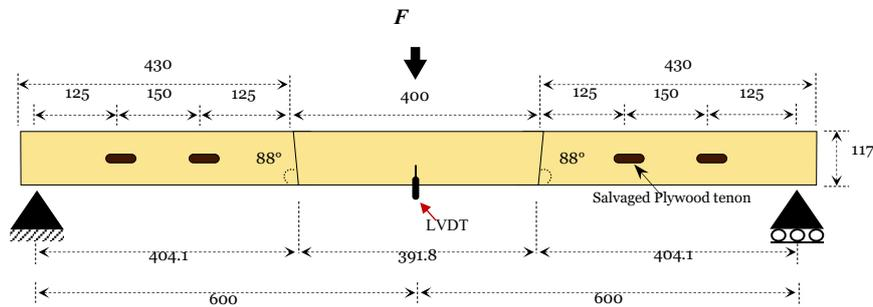
Fig.11: Dimensions of the salvaged timber elements in the small-scale DLT panels and the three-point bending test set-up. Dimensions in mm.
