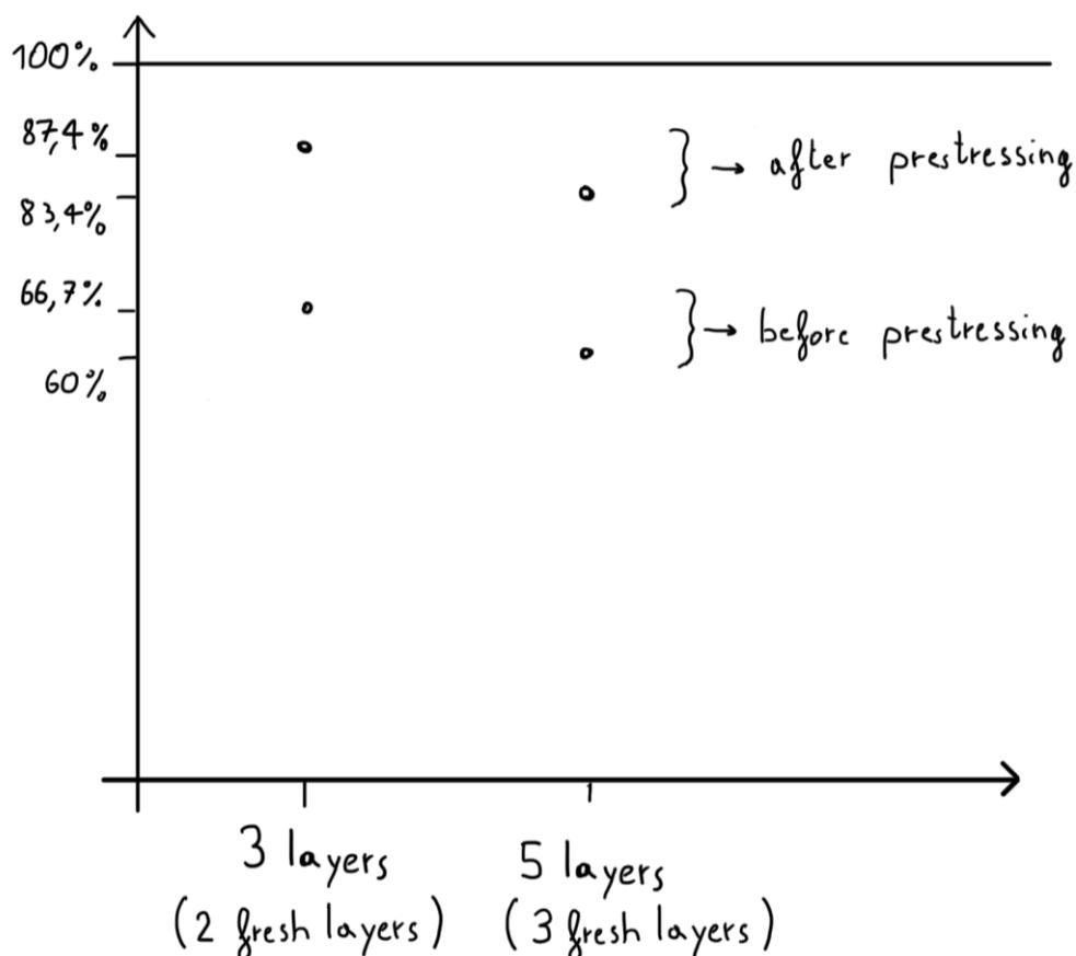
Fig. 43: Increment of stiffness due to the interlocking system for the three layers and five layers sample.
