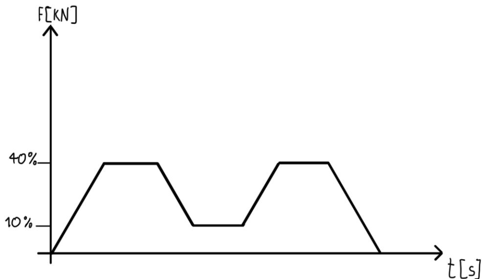
Fig. 13: Loading procedure for the three-point bending test.
