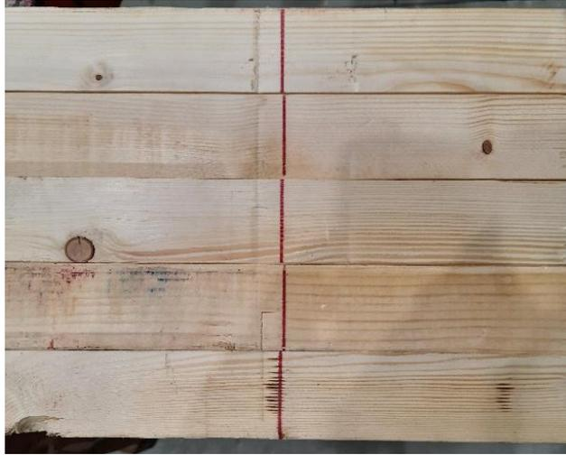
*Fig. 25: movement of the salvaged timber layers after the insertion of the middle boards*
