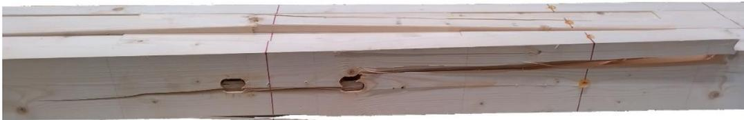
*Fig. 41: Failure mode of specimen D.*
