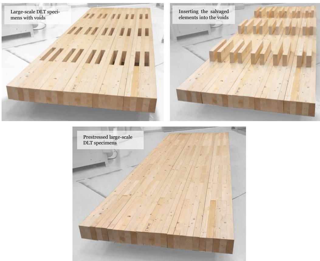
Fig. 23: (a) Slab system without the piece in the middle, (b) slab system during the insertion of the middle piece, (c) slab system at the end of the construction procedure.
