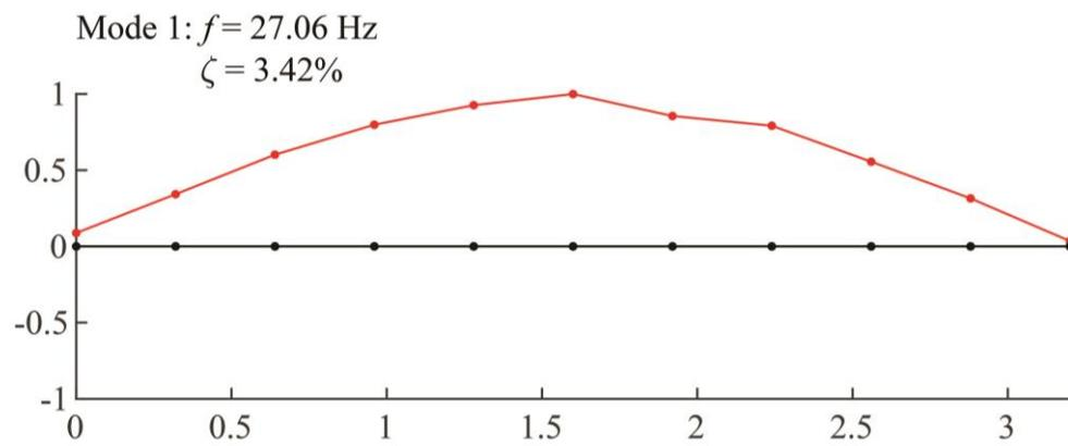
*Fig. A21: The first vibration mode of specimen E after prestressing.*
