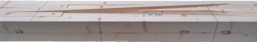
*Fig. 38: Failure mode specimen B*
