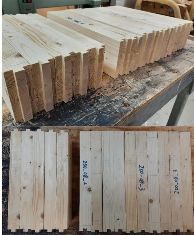
*Fig. 5: salvaged board profiled with mortises and tenons shape.*
