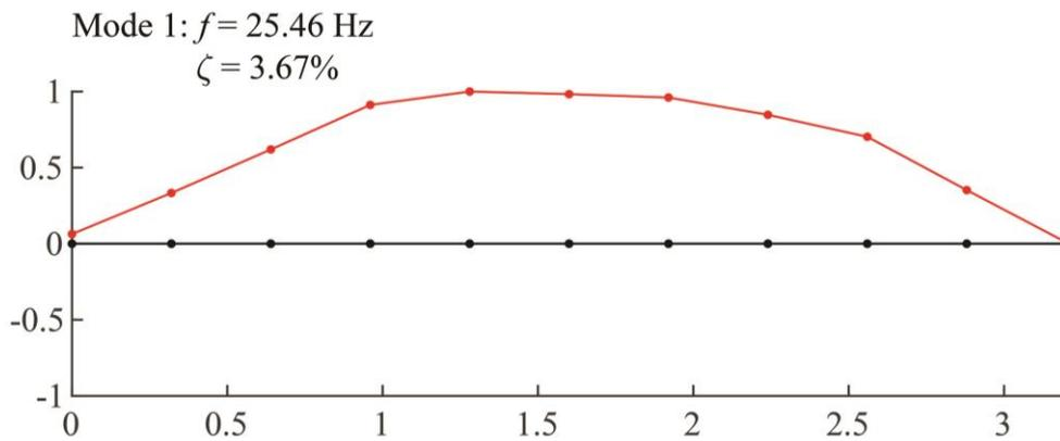
Fig. A16: The first vibration mode of specimen C before prestressing.
