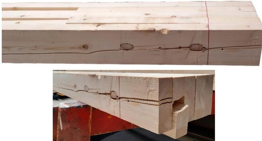
*Fig. 40: (a-b) Shear failure of specimen C.*
