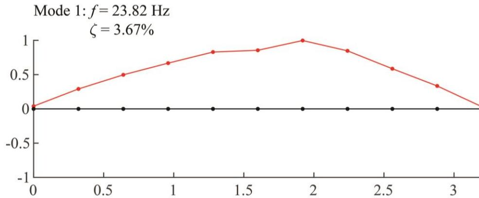
*Fig. A12: The first vibration mode of specimen A before prestressing.*
