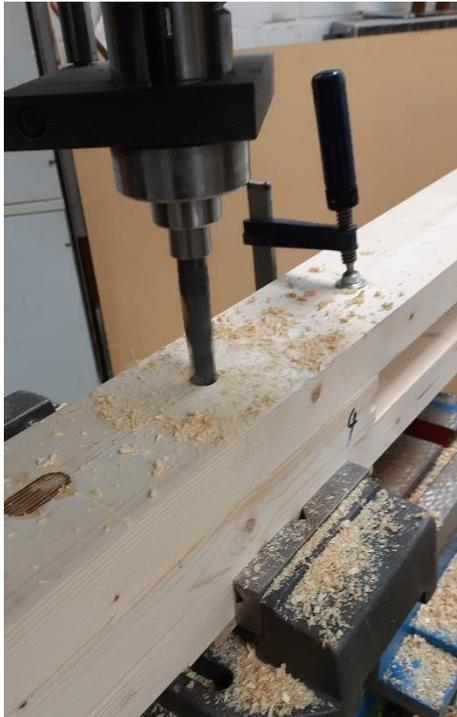
*Fig. 10: Drilling procedure to produce the hole for the tenon.*
