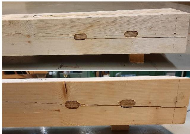
*Fig. 29: (a) shear failure A, (b) shear failure B.*
