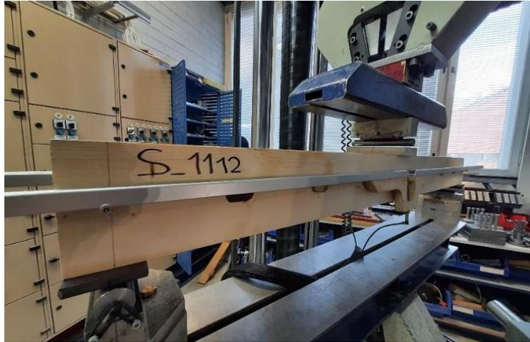
Fig. 15: Laminated system without end-to-end interlocking ready to be tested.
