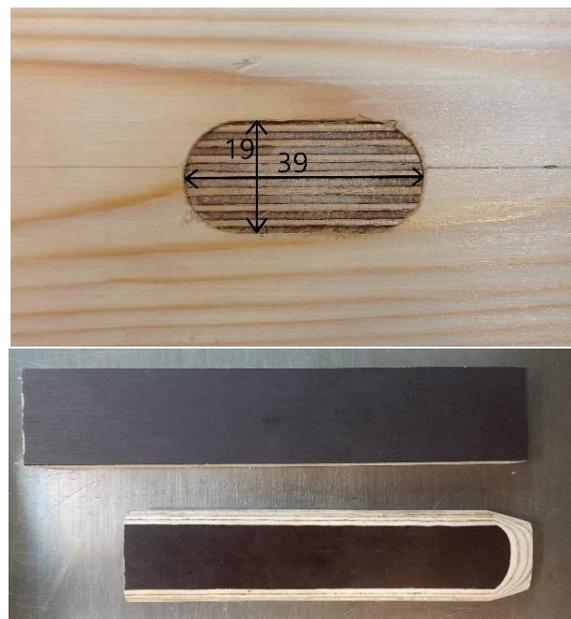
*Fig. 8: (a) dimension (in mm) of the salvaged plywood tenon; (b) plywood tenon before and after the processing.*
