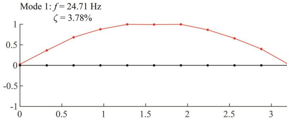
Fig. A14: The first vibration mode of specimen B before prestressing.
