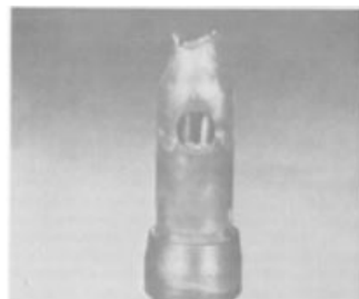
Figure 3.15: Missing probe tips, [16]
