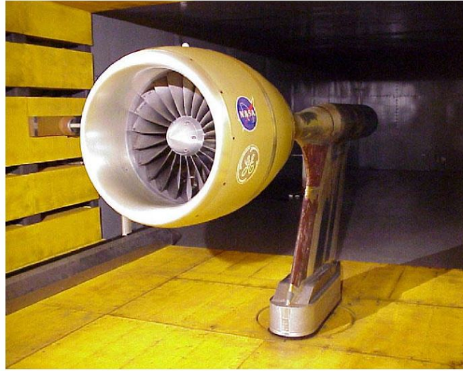
Figure 5.1: NASA SDT model installed at the NASA Glenn Wind Tunnel.
