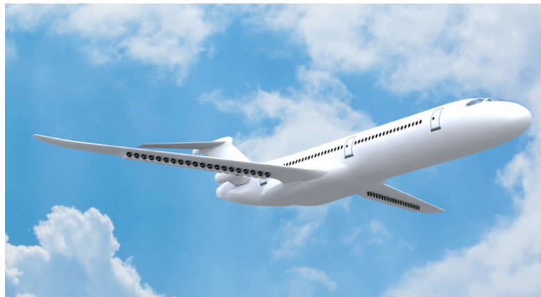
Figure 1.5: ONERA's DRAGON concept with distributed ducted fan
