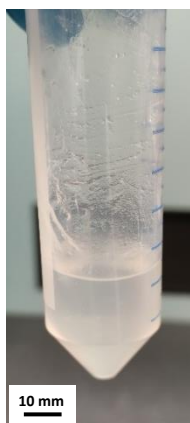
Figure 28- Transparency of the nanocomposite resin, thanks to well dispersed modified CNFs.
