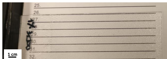
Figure 38- Transparency of UV-cured nanocomposite films with 1%vol Bu 4 NOH-hyMPS-TOCNF.
