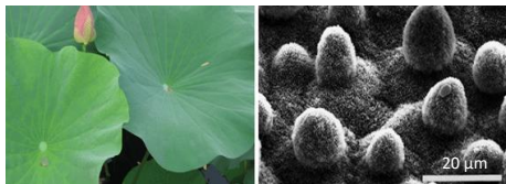
Figure 20- SEM image of lotus leaves nano-structure with nano-pillars [60].
