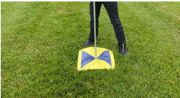
**Figure 5. 3** Modules of Ground Control Points (GCPs)
