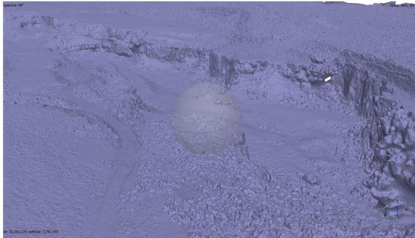
The mesh generated in Metashape from nadir & inclined images acquired in the Benchmark survey.
