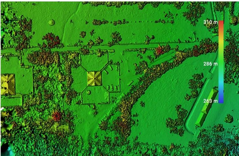
Digital Elevation Model of generated model by Metashape in the Villa Ghia survey.
