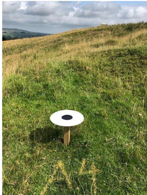
**Figure 4. 2** ICP and GCP target location of Benchmark. **Figure 4. 3** CP label sprayed for identification
