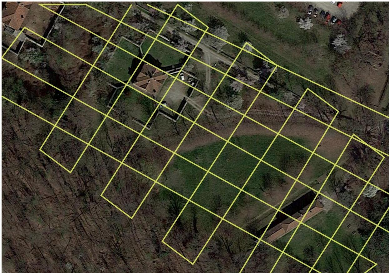
**Figure 4. 4** Flight Mission Path of the Villa Ghia test site.
