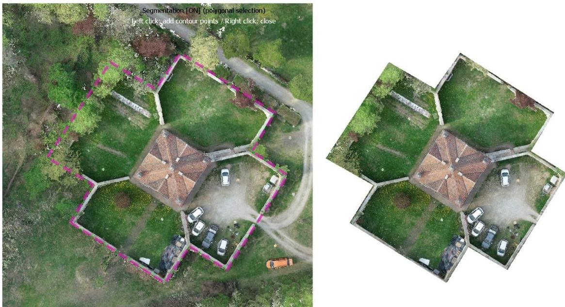
Figure 6.15. Specification and cut of the model area with Segment In option for the C2C distance analysis in CloudCompare.
