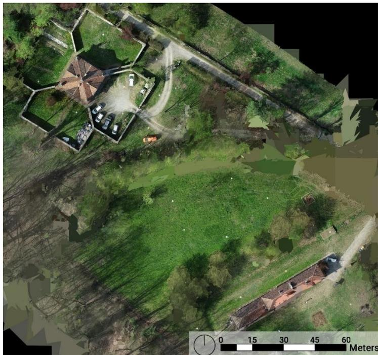
Figure 6. 15 Orthoprojection image of DJI Zenmuse L1 processed by Reality Capture
