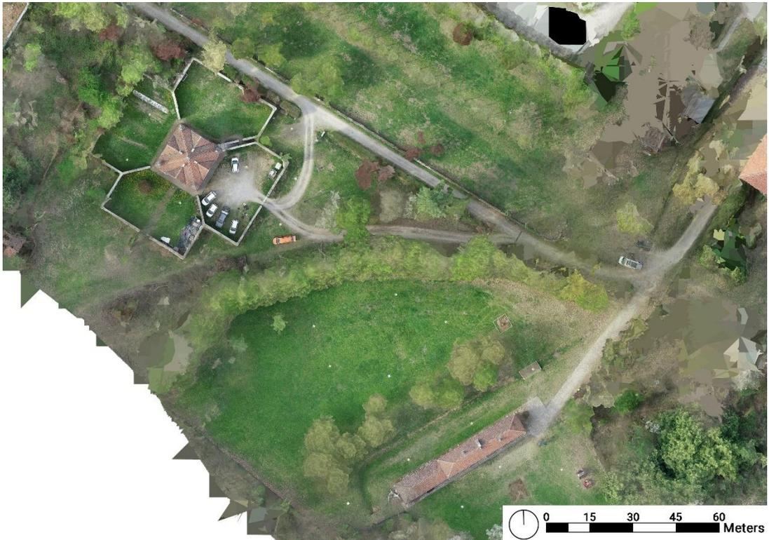
Figure 6. 17 Orthorectification image of DJI Phantom 4 RTK processed by Reality Capture
