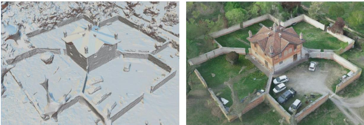
**Figure 5. 8 and Figure 5. 9** Generated Photogrammetric Model of Villa Ghia in Reality Capture, Mesh (left) and Textured Model (right)
