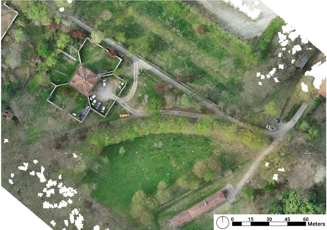
Figure 6. 16 Orthorectification image of DJI Phantom 4 RTK processed by Metashape
