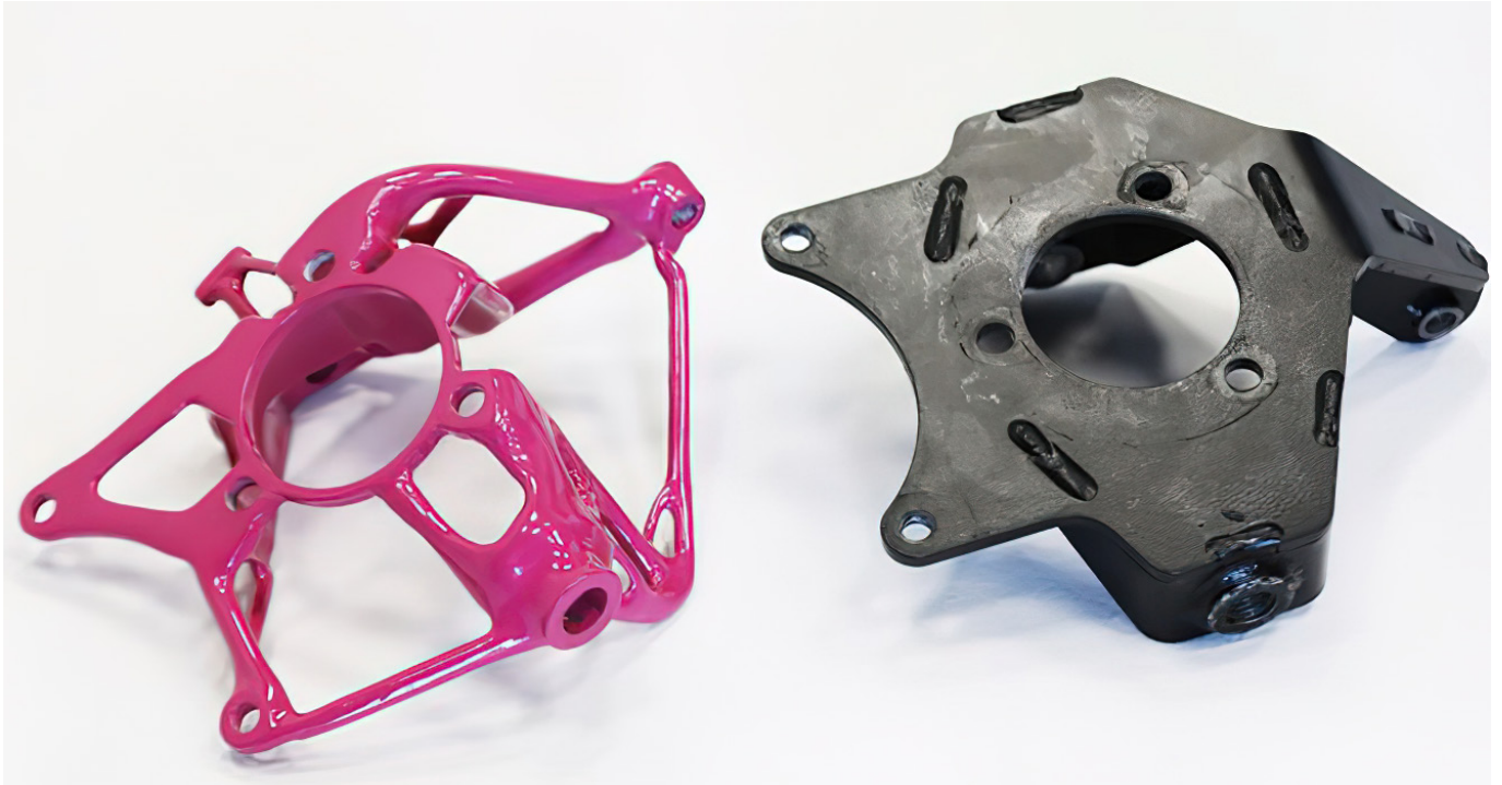
FUV Automotive 3D Printed Steering Knuckles(left), the original component is a nine-piece weldment weighing about 6 pounds (right)
