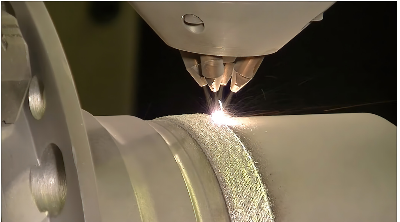
Optomec DED based LENS technology, 3D printing onto a premade metal surface
