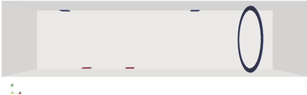
Figure 3.7: Hatches - start configuration. In one of the two head configurations, the hatches are placed at the top and bottom, corresponding to the axis of the autoclave.
