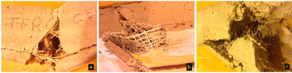
Figure 30. Specimens with bi-directional reinforcement in fiberglass and dispersed fibers after the flexural strength test [55].
