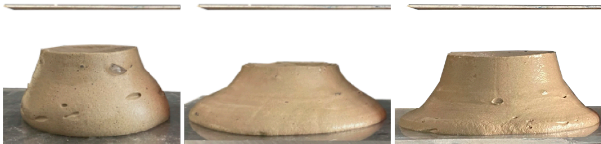
Figure 49. Image showing the influence of density on the slump for the second experimental campaign. On the left, mix 02-NF-100 presents a density of 100\text{kg/m}^3 ; in the middle, mix 02-NF-300 shows an admixture with a 300\text{kg/m}^3 density; on the right, mix 02-NF-500 shows the slump of an admixture with a 500\text{kg/m}^3 density.
