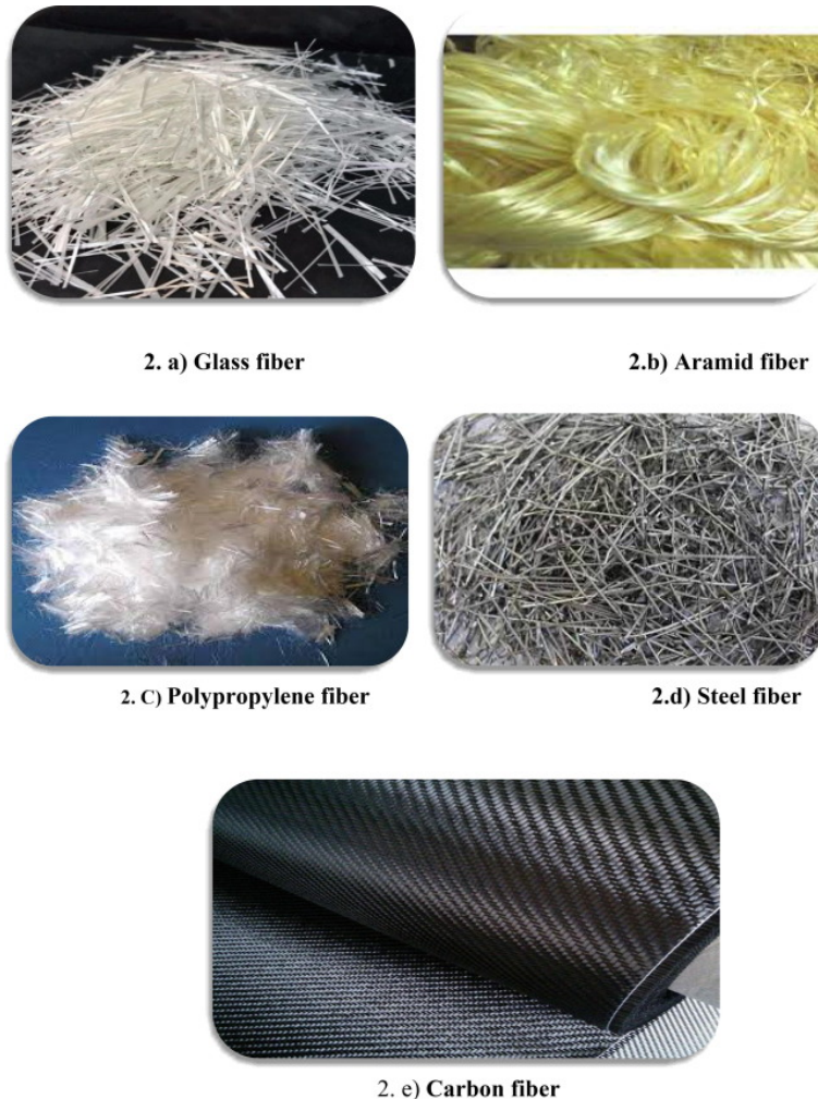
Figure 4. Various types of artificial fibers [21].
