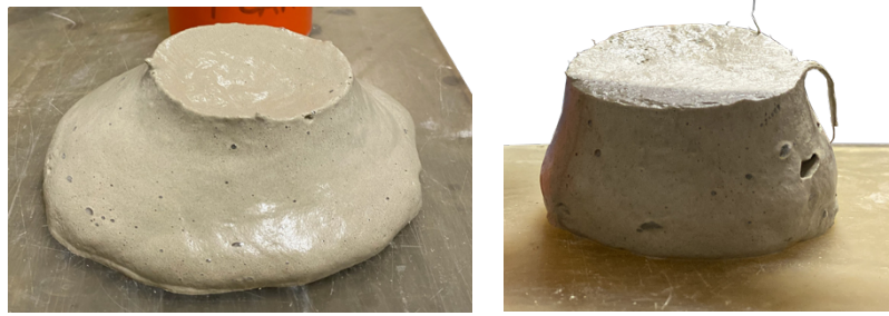
Figure 45. Image showing the influence of fiber addition on the slump for the first experimental campaign on the fiber treatment choice. On the left, mix 01-NF represents the slump without fibers; on the right, mix 01-NTF shows the slump of an admixture containing fibers.
