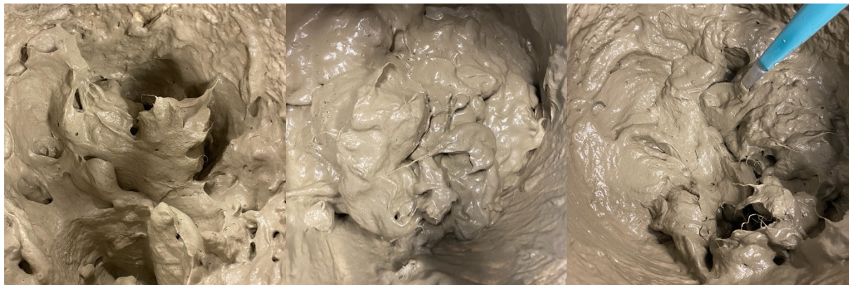
Figure 41. Images of final mixture with fibers: 100\text{Kg/m}^3 on the left, 300\text{Kg/m}^3 in the center, and 500\text{Kg/m}^3 on the right
