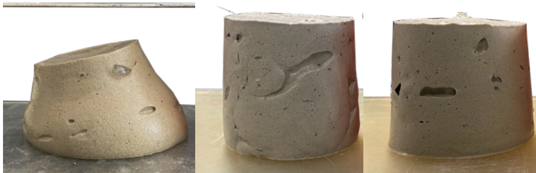
Figure 46. Image showing the influence of fiber addition on the slump for the second experimental campaign on the 100 \text{ kg/m}^3 density. On the left, mix 02-NF-100 represents the slump without fibers; in the middle, mix 02-NTF-100-2,5% shows an admixture with a 2,5% F/C ratio; on the right, mix 02-NTF-100-5% shows the slump of an admixture with a 5% F/C ratio.
