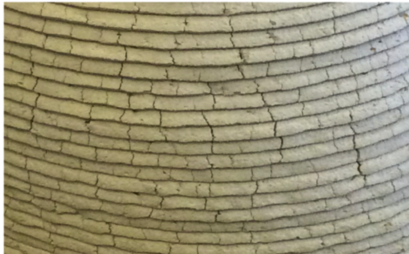
Figure 25. Example of shrinkage cracks in an element made using 3D Concrete Printing [53].
