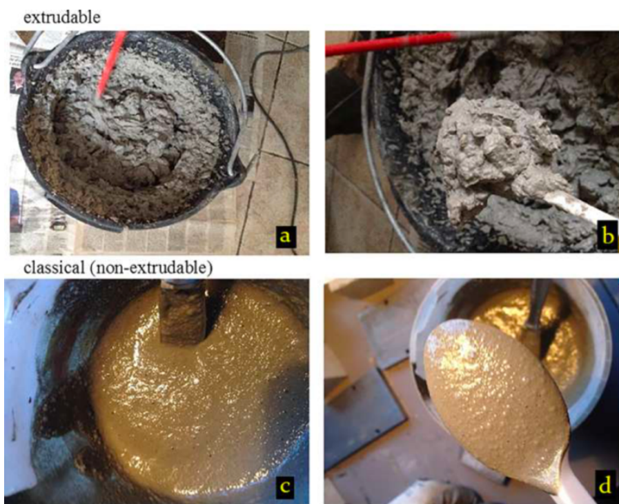
Figure 36. Quality comparison in terms of consistency, cohesion and viscosity in the fresh state between an extrudable foamed concrete mix (above) and a classic foamed concrete mix (below) both made to obtain a final density of 600 \text{ kg/m}^3 [55].
