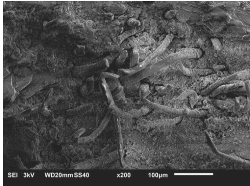
Figure 9. SWF reinforced mortar stored on air with visible wool filaments [34].
