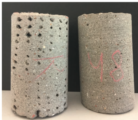
Figure 24. Elements characterized by variable filament density on the left and constant filament density on the right. In the first case, the various layers and voids of various sizes are recognized, while in the second, the element is homogeneous [51].
