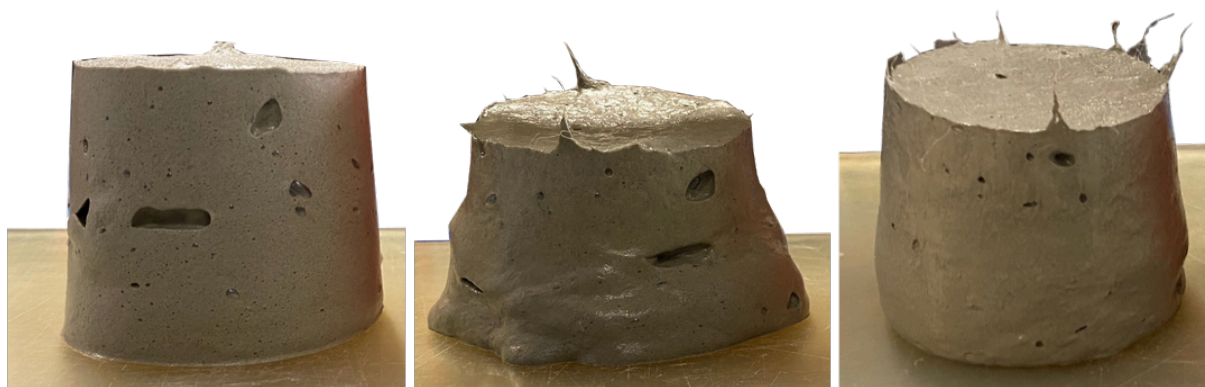
Figure 47. Image showing the influence of fiber addition on the slump for the second experimental campaign on the 300\text{kg/m}^3 density. On the left, mix 02-NF-300 represents the slump without fibers; in the middle, mix 02-NTF-300-2,5 shows an admixture with a 2,5% F/C ratio; on the right, mix 02-NTF-300-5 shows the slump of an admixture with a 5% F/C ratio.
