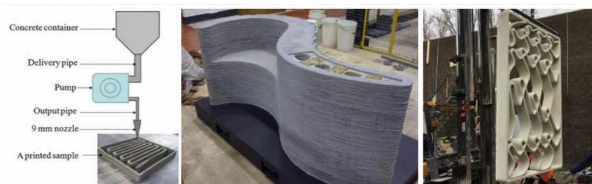
Figure 20. CP construction process (left), CP built wall-bench (center), and façade element projected parametrically by Bruil (2019) (right) [50].
