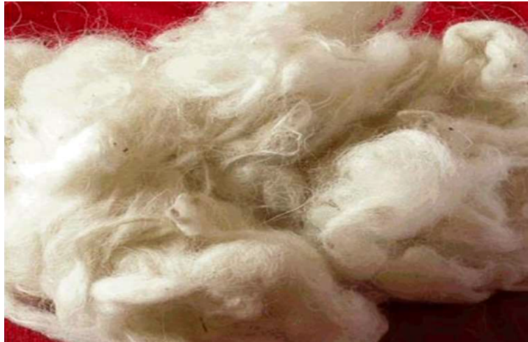
Figure 6. Ordinary sheep wool fibers used in concrete reinforcement [34].
