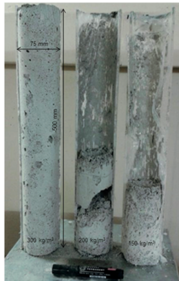
Figure 12. Example of instability in ultralightweight foamed concrete. From left to right, density is equal to 300, 200, and 150 kg/m 3 [48].
