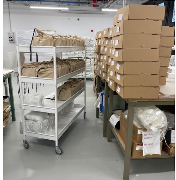
**FIGURA 14: PRESENZA DI NUMEROSI CARRELLI DI SEMILAVORATO IN ATTESA, ELEVATO HANDLING, TANTO SPAZIO OCCUPATO DAI CARRELLI**
