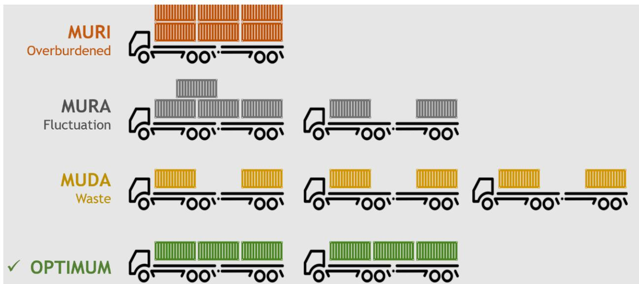
FIGURA 3: DISTURBI DELLA PRODUZIONE MUDA-MURI-MUDA
