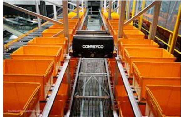
**Figura 2.5 – Shuttle mini-load**
