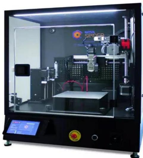
Figure 27. Novaspider V5 elettrospinning instrument in Polito<sup>BIO</sup>Med Lab.
