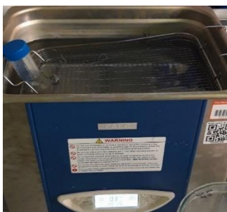
Figure 30 Operating ultrasonic bath, with a falcon filled with acetone and the mould
