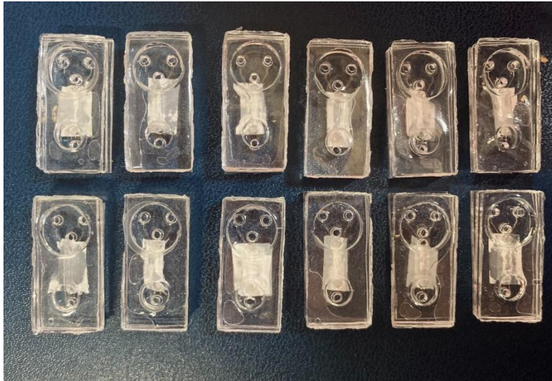
Figure 46 Assembled devices realized to perform permeability test and for cells seeding
