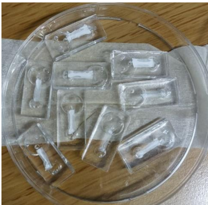
Figure 34 Top layers bonded with reservoir layers and membranes
