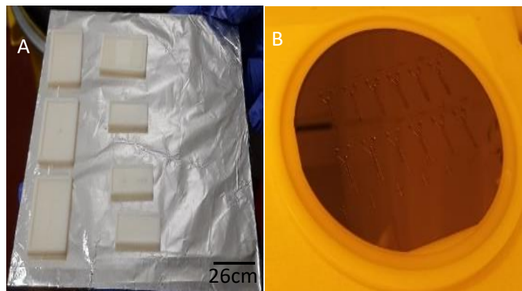
Figure 31 A) Top and reservoir layer replicas after the thermal polymerisation ; B) bottom layer replica before the thermal polymerisation.
