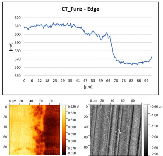
Figure 14: Kelvin Probe of CT functionalized vs CT Ti6Al4V measured at the edge.
