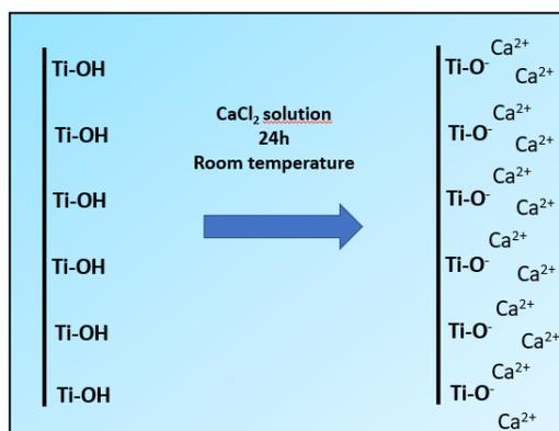
Figure 7: Scheme of possible interaction of  $\text{Ca}^{2+}$  ions with the titanium alloy surface.
