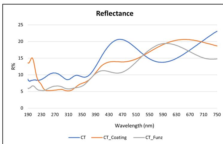
Figure 19: Diffuse reflectance spectra of CT Ti6Al4V, CT functionalized and CT coated samples.
