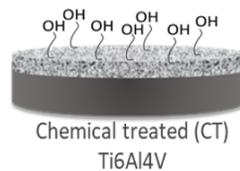
Figure 6: Chemical Treated (CT) Ti6Al4V
