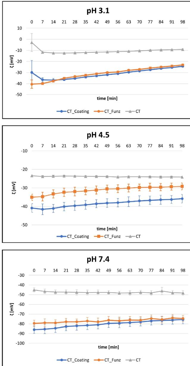
Figure: Zeta potential at constant pH vs. time of CT Ti6Al4V, CT functionalized and CT coated samples.
