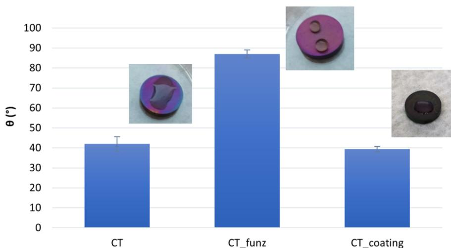
Figure 11: Contact angle measurement of CT Ti6Al4V, CT coated and CT-functionalized samples.
