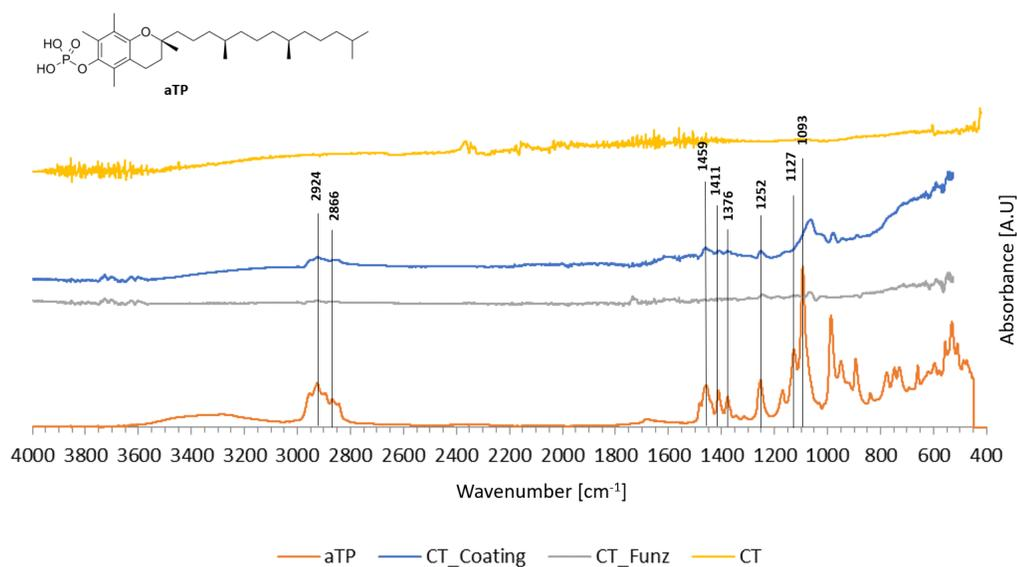
Figure 16: FTIR analysis of CT functionalized and CT coated samples and pure  $\alpha$ -tocopherol phosphate.
