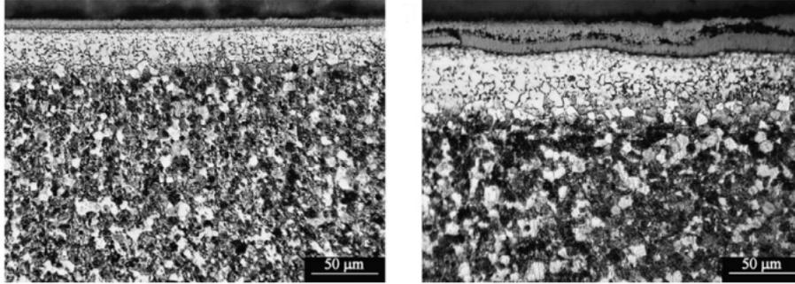
Figure 5: LOM micrographs of Ti-6Al-4V oxidised through thermal treatments.
