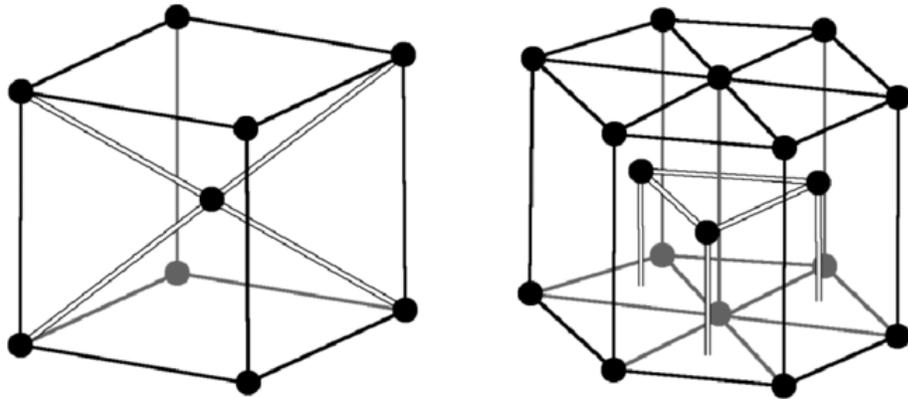
Figure 3: Crystal structure of Titanium. Left:  $\beta$  structure (bcc) Right:  $\alpha$  structure (hcp) [29]
