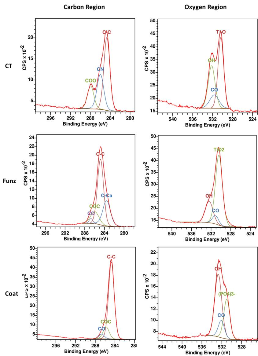
Figure 18: High resolution XPS spectra of C and O regions of CT, CT functionalized and CT coated samples.
