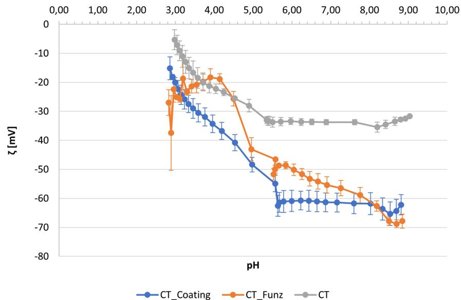
Figure 12: Zeta potential vs. pH of CT Ti6Al4V, CT functionalized and CT coated samples.
