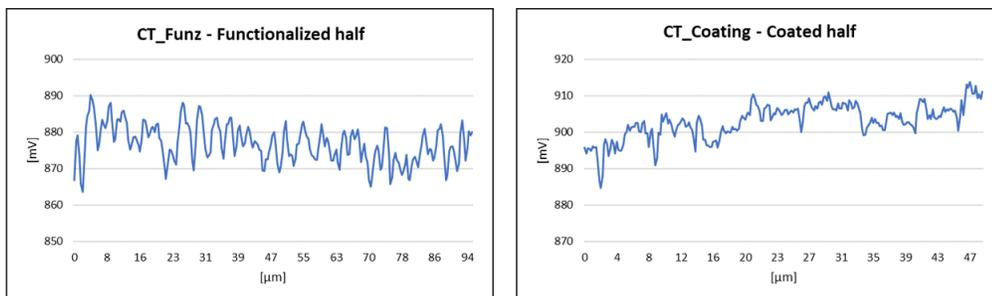
Figure 15: Kelvin Probe analysis of the functionalized and coated half.
