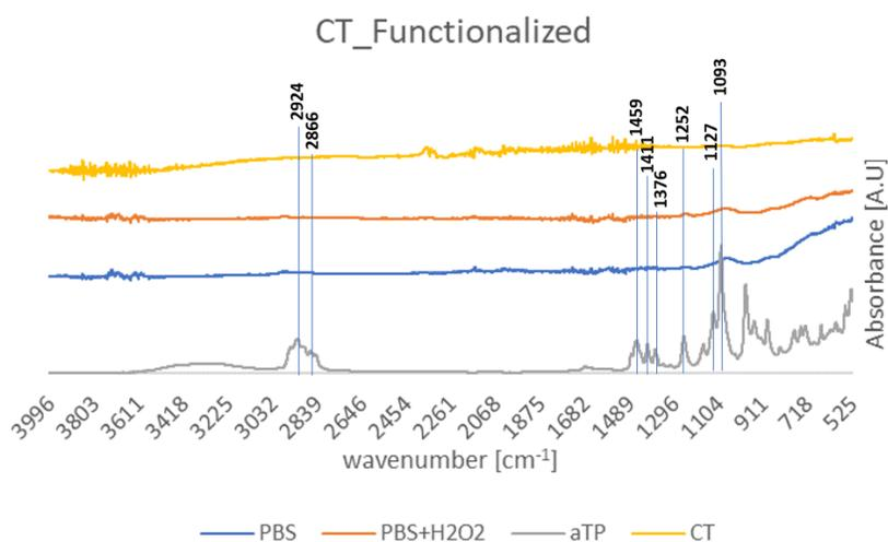
Figure 24: FTIR of the CT functionalized sample after immersion in PBS and PBS+H<sub>2</sub>O<sub>2</sub>.
