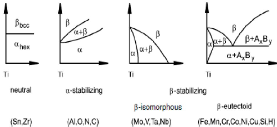
Figure 4: Effects of different alloying elements on Ti alloys. [30]
