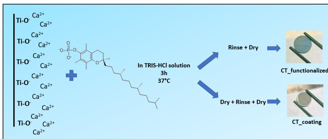
Figure 9: CT Ti6Al4V alloy coated and functionalized.
