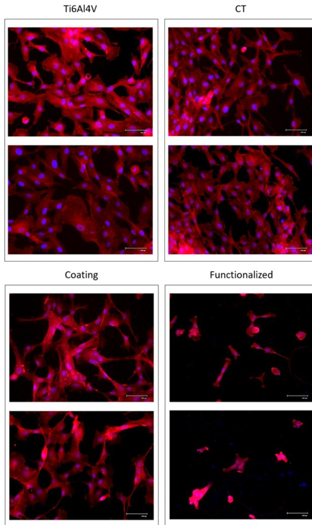
Figure 27: Alpha-tocopherol doped materials – fluorescence staining (cytoskeleton and nuclei) of hMSC-human mesenchymal stem cells.
