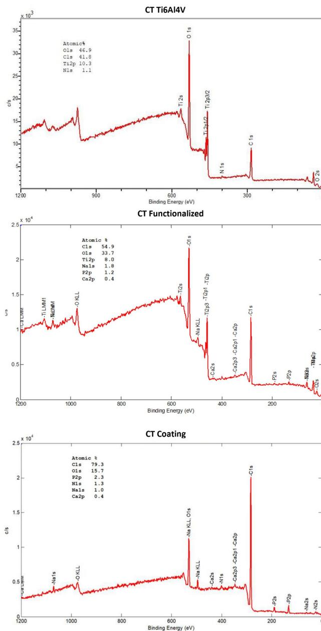
Figure 17: XPS spectra of CT, CT Functionalized and CT coated samples.
