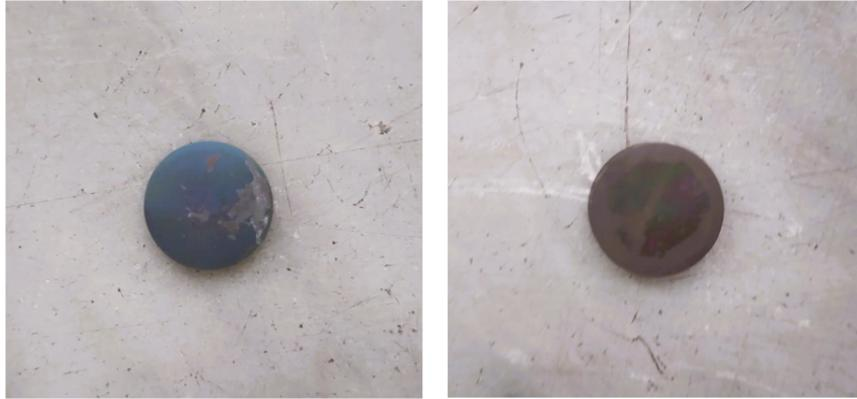
Figure 21: Detached coating on the CT coated samples after a two weeks immersion in PBS (left) and PBS+H<sub>2</sub>O<sub>2</sub> (right).
