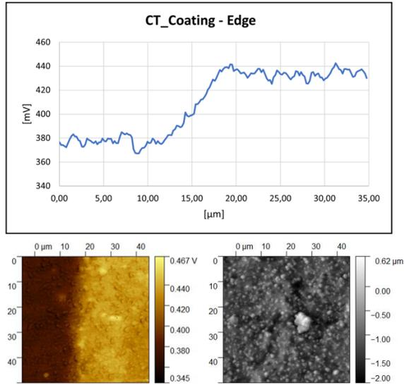
Figure 13: Kelvin Probe of CT coating vs CT Ti6Al4V measured at the edge.
