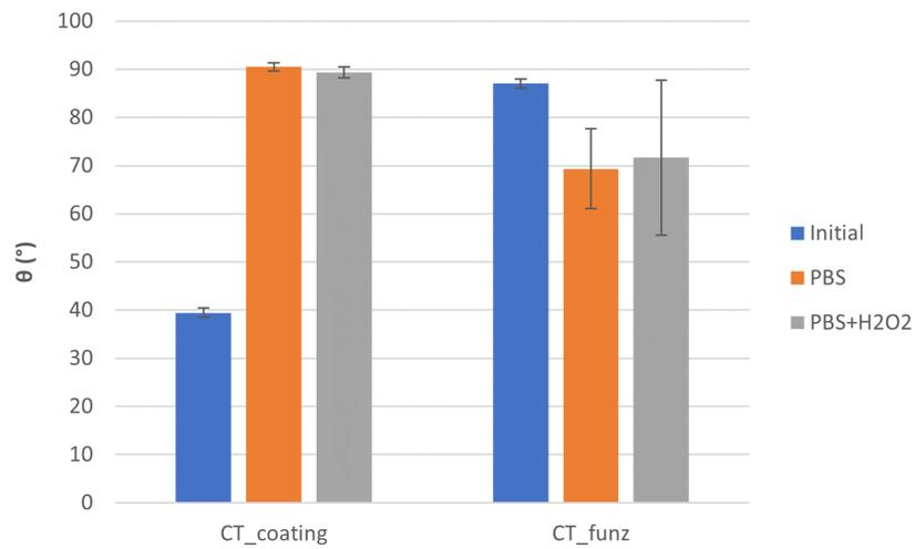
Figure 22: Comparison between the contact angle values obtained for the CT functionalized and CT coated sample before and after the immersion in PBS and PBS+H<sub>2</sub>O<sub>2</sub>.
