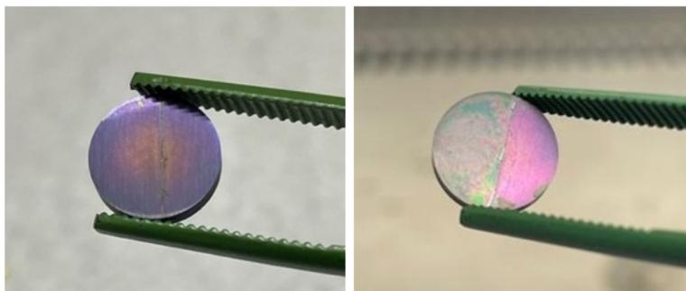
Figure 10: KP samples: CT-functionalized on the left and CT-coated on the right.
