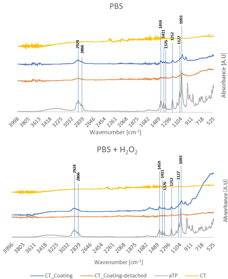
Figure 23: FTIR of the CT coated sample after immersion in PBS and PBS+H<sub>2</sub>O<sub>2</sub>.
