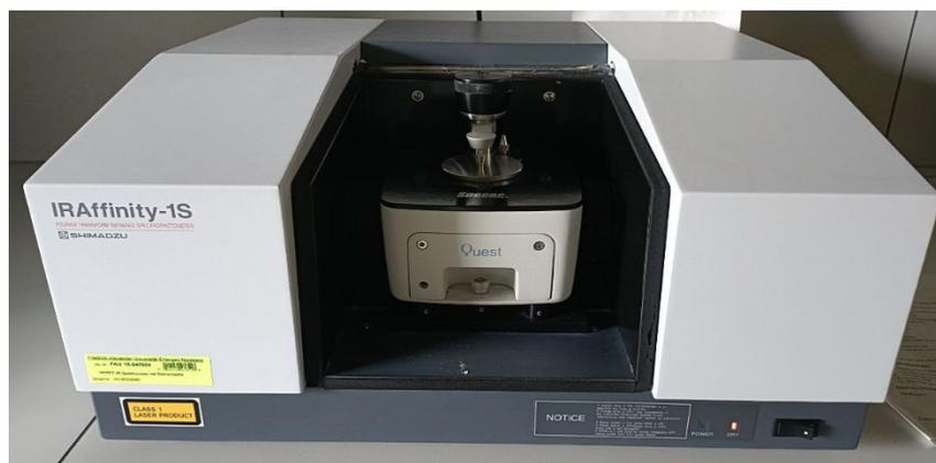
Figure 15. FTIR device (IRAffinity-1S Shimadzu).
