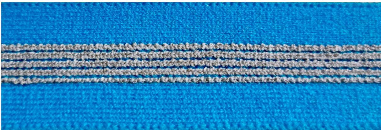
**Figure 4.3:** A close-up picture of the aWare strap belt. A silver coated yarn is interweaved in the nylon and spandex matrix.
