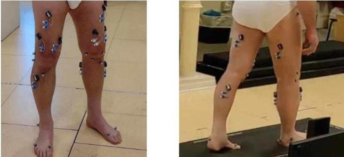
*Figure 5-7: EMG electrodes placements*
