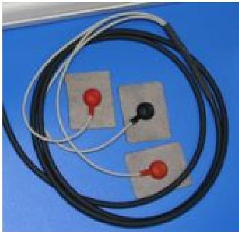
**Figure 2.5:** Surface EMG electrodes.
