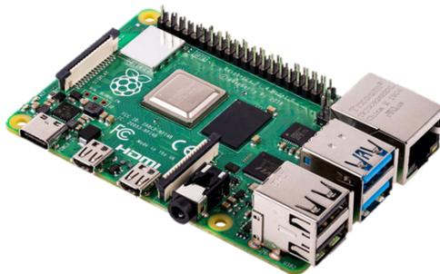
**Figure 7.1:** Raspberry Pi 4B board. Processor: quad-core Cortex-A72 (ARM v8) 64-bit SoC @ 1.5GHz.
