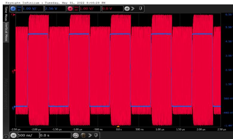
**Figure 4.22:** Output signal after the amplification;  $V_{OUT}^{pp}=7.93$  V.
