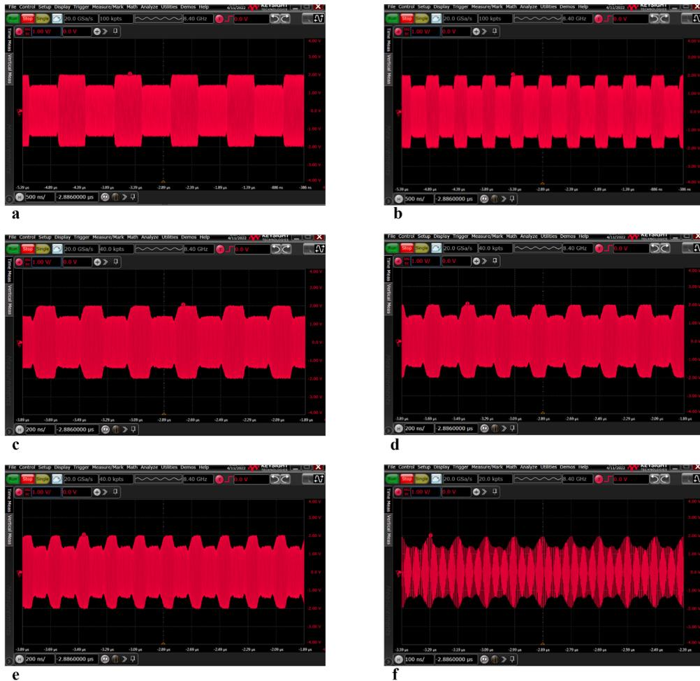
**Figure 3.12:** Received signal at different data rate: a) 2 Mbps, b) 4 Mbps, c) 6 Mbps, d) 8 Mbps, e) 10 Mbps, f) 20 Mbps.
