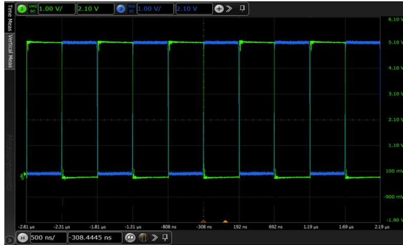
**Figure 4.7:** TTL input signal after the inverter. *Green trace:* the original signal sent from the waveform generator. *Blue trace:* the signal after passing the inverter.
