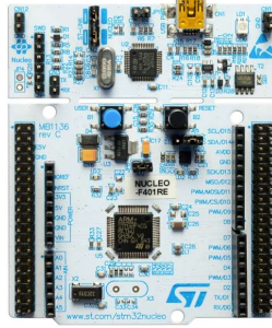
Figure 38: STM32 Nucleo-64 development board with STM32F446RE Micro-Controller Unit. The image comes from the ST website.
