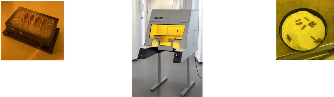
Figure 5: 4a) green samples before cleaning phase; 4b) Lithoz Cera Cleaning Station Ultra; 4c) green samples after cleaning
