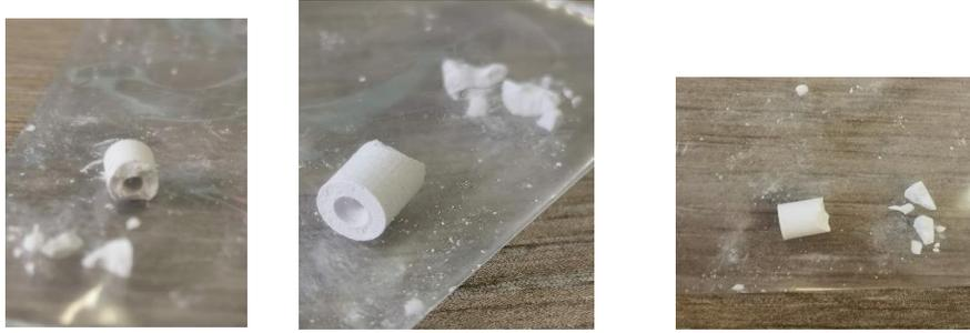
Figure 12: Green bodies after the camera-oven test
