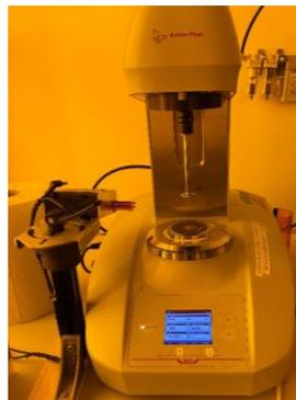
*Figure 16: Rheometer used for the viscosity test*
