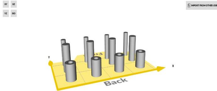
Figure 17: Virtual Tray of the cylinders set for the shrinkage test
