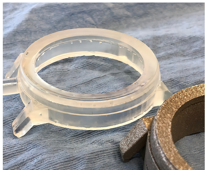
Vat photopolymerization's high resolution makes layering effects almost invisible
