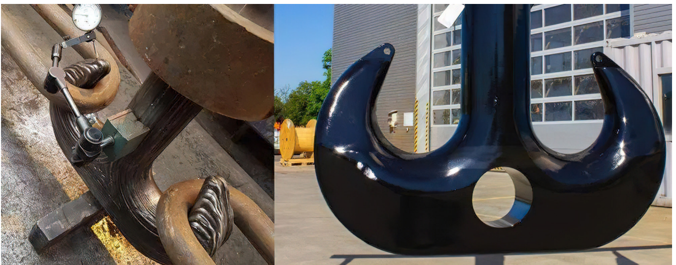
Crane hooks printed with WAAM 3D printing technology
