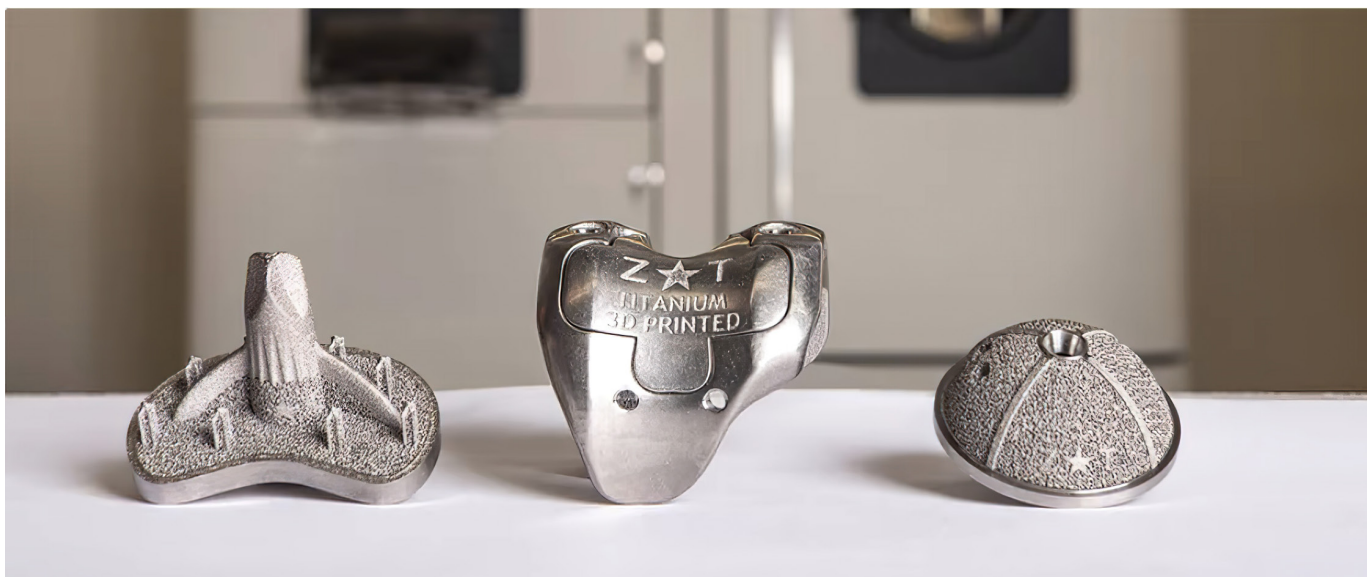
Sample orthopedic implants 3D printed in titanium by Zenith Tecnica using GE's electron beam melting technology
