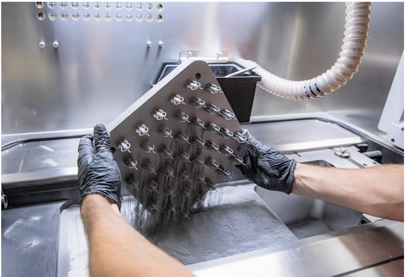
Removing a DMLS print from the powder.
