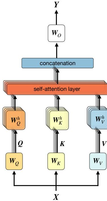
Figure 4.7: Multi-Head Attention layer. The matrix input  $\mathbf{X}$  is mapped into Query, Key and Value matrices ( $\mathbf{Q}, \mathbf{K}, \mathbf{V}$ ). These are re-mapped and fed in parallel to  $H$  self-attention layers. The results of these are concatenated and finally mapped into output matrix  $\mathbf{Y}$ .
