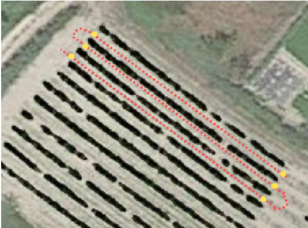
**Figure 1.2:** Aerial view of a vineyard. The estimated waypoints are shown in yellow, the global path in red and the occupancy grid (segmented vineyard) in black. They allow a UGV to move along the vinerows.
