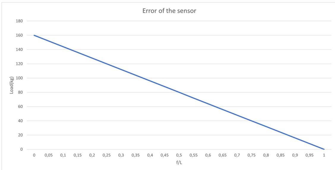
Figure 3.6: Error of the sensor measuring the load
