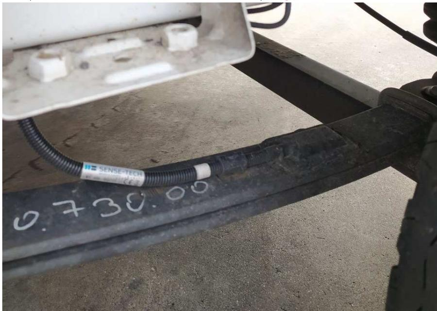
Figure 1.3: SG sensor on a leaf spring
