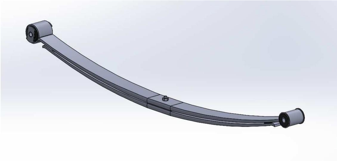
Figure 2.2: Model of the parabolic leaf-spring with Solidworks
