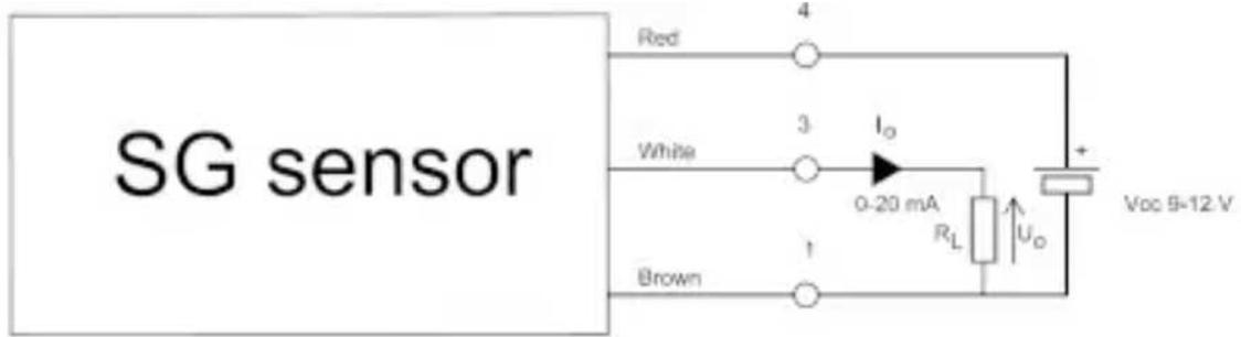
Figure 6.16: Resistive load connection to the strain gauge
