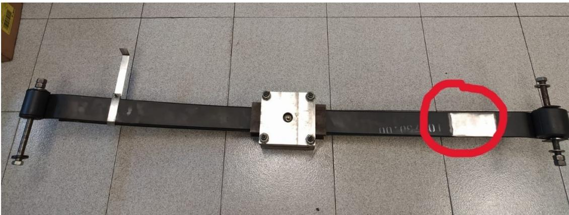
Figure 3.12: Grinding of the leaf spring material
