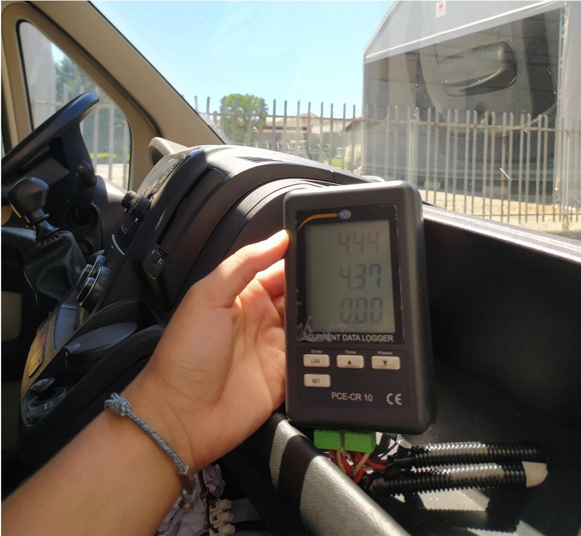
Figure 6.5: Data logger installation on the truck
