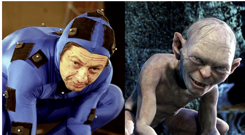
Figure 1.11: Andy Serkis during the shoot of The “Lord of The Rings: The Two Towers” (2002) posing in a motion capture suit to perform Gollum [18].
