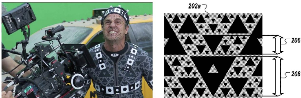
Figure 1.17: On the left a scene from “Avengers” [24], on the right the fractal pattern used on the mocap suit [25]
