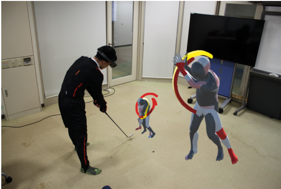
Figure 2.3: Using the AR HMD the user can see himself or herself playing with the golf-club and also the teacher avatar and his or her own avatar [61].
