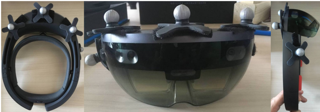
Figure 3.2: Optitrack tracker placed on HoloLens to be recognized from the optical system
