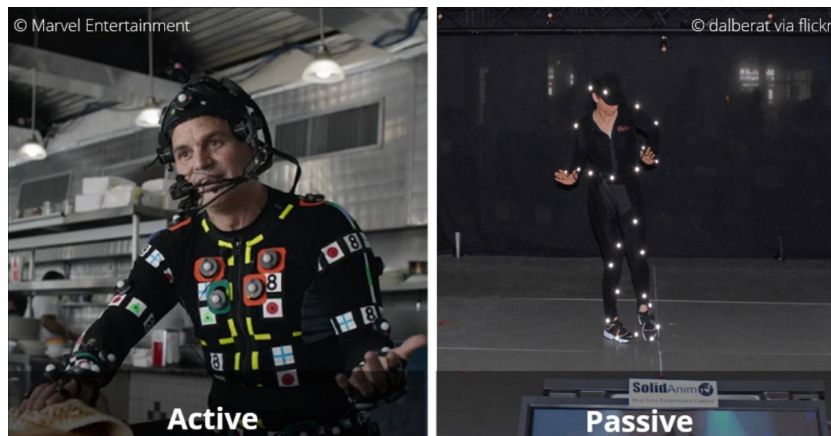
Figure 1.14: Examples of active and passive markers [22].
