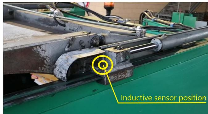
**Figure 3.12:** Inductive sensor position
