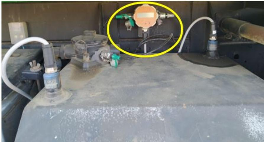
**Figure 3.8:** C optical sensor installation
