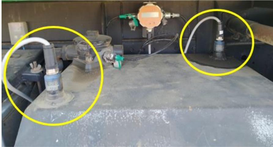
**Figure 3.6:** Oil level sensors location
