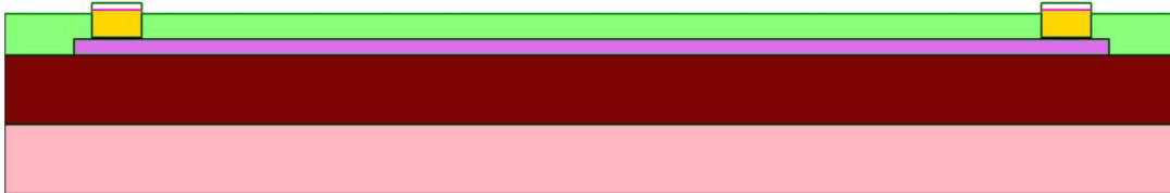
Figure 4.24. Cross-section view of the final structure with surrounding gas-like material (green).
