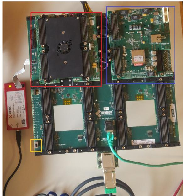
Figure 5.1: Top view of the proFPGA system. Image taken from [6].
