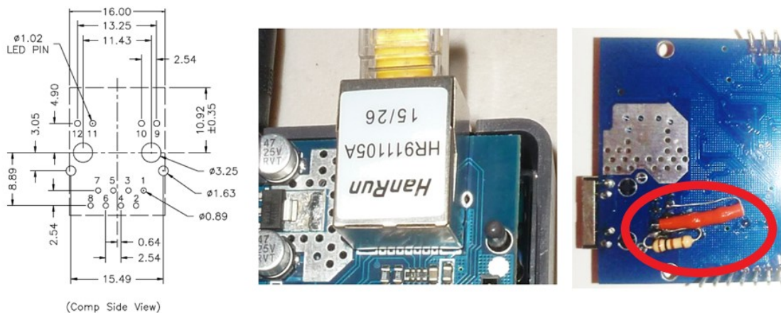
Figure 3.5: Ethernet Shield Connector Fixing
