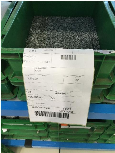
**Figura 4.6:** Cassetta odette verde identificata tramite C.D.I.
