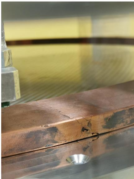
Figure 3.8: Copper rim defect
