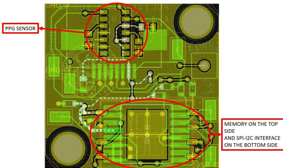
Figure 9.3: PulsECG: PPG board
