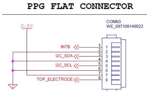
Figure 5.42: Würth Elektronik 687108149022 schematics
