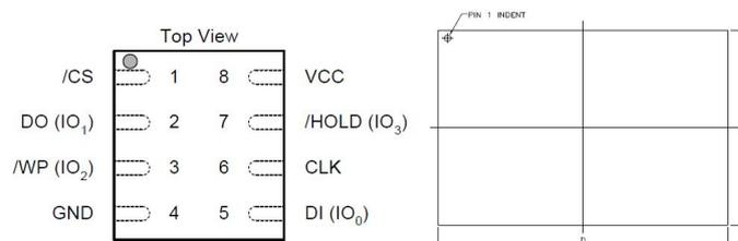
Figure 5.57: W25N01GV pinout and dimensions
