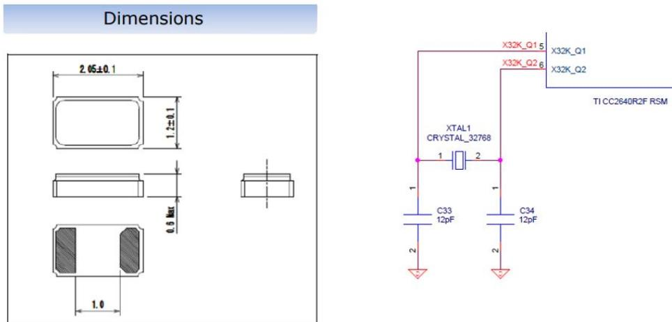
Figure 5.51: SC20S-12.5PF20PPM schematics
