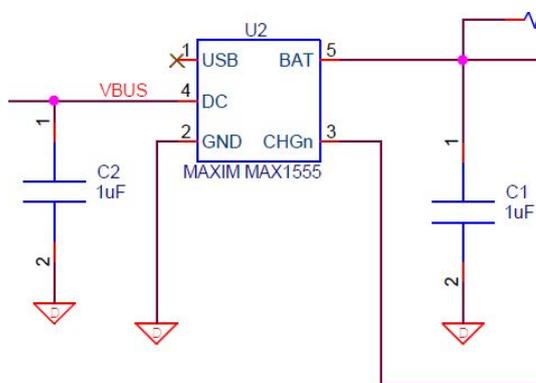
Figure 5.17: MAX1555 schematic
