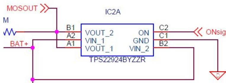
Figure 5.31: Mosfet TPS22924BYZZR schematic
