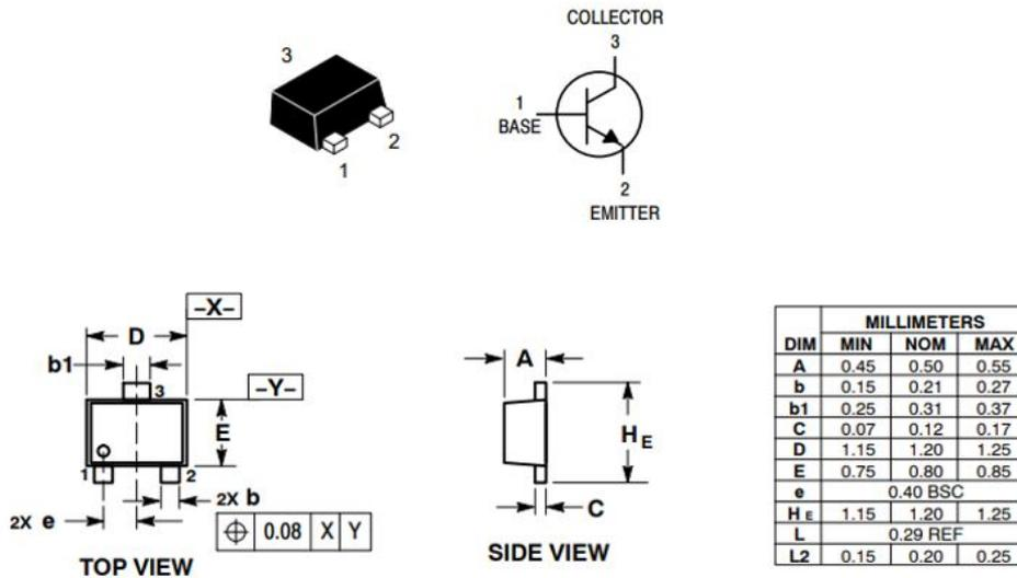
Figure 5.32: BJT MMBT2222AM3T5G pinout and dimensions
