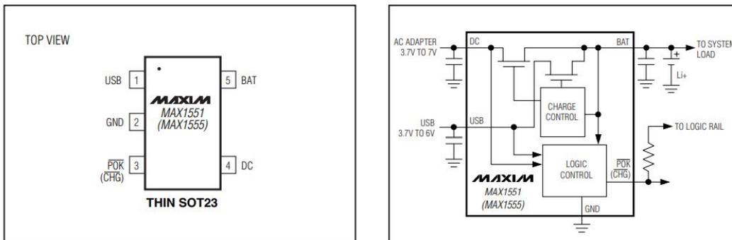
Figure 5.16: Charger module MAX1555: pinout and typical circuit
