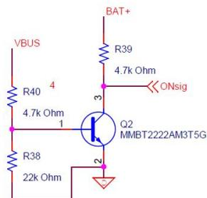
Figure 5.33: BJT MMBT2222AM3T5G schematic
