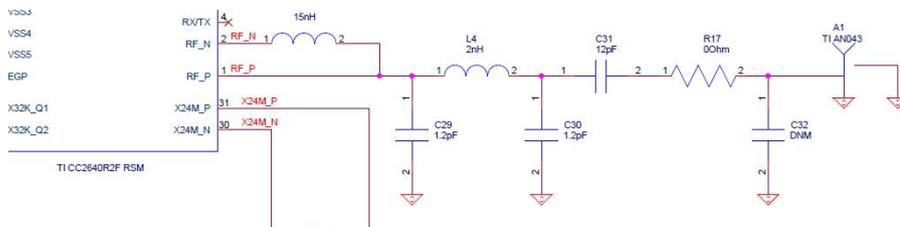
Figure 5.6: Antenna schematic
