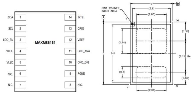
Figure 5.54: MAX86161 pinout
