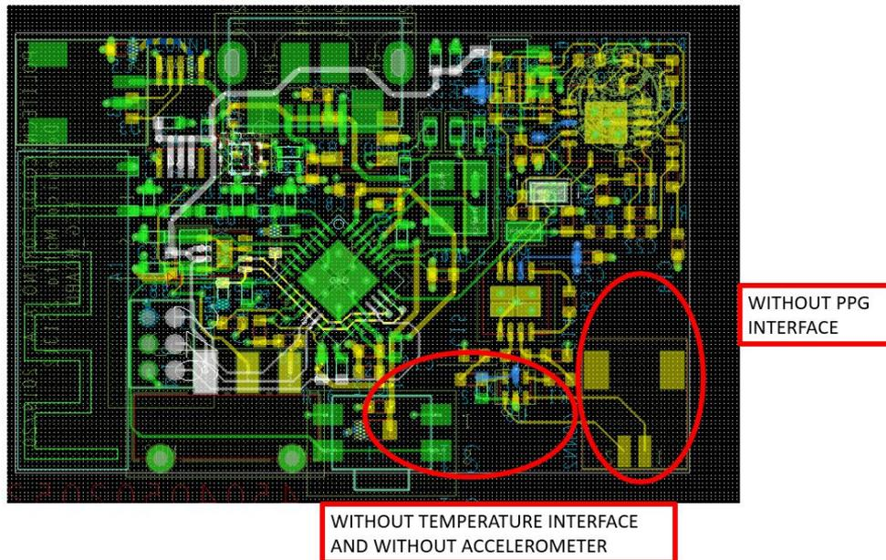
Figure 9.6: ECG watch board
