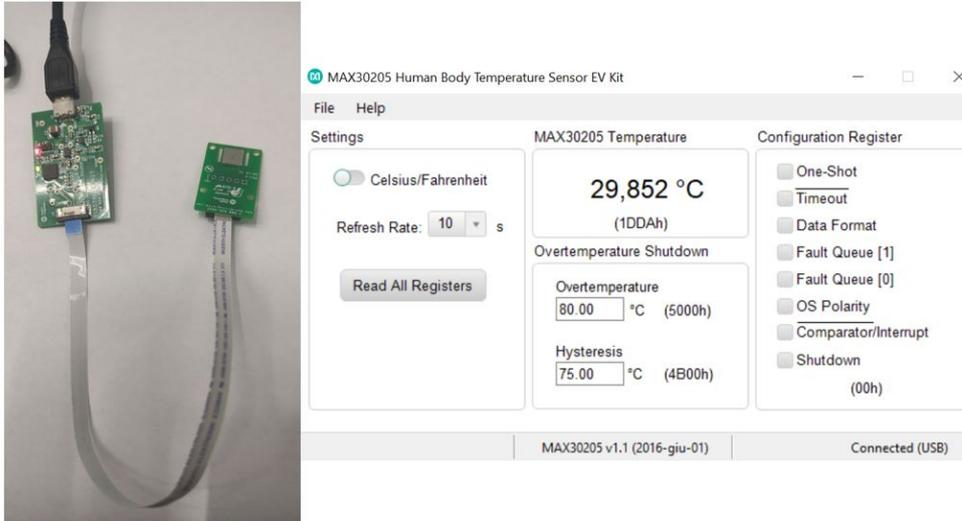
Figure 11.5: Ambient temperature with evaluation board
