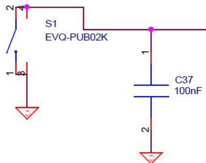
Figure 5.46: Push button EVQ-PUB02K schematic
