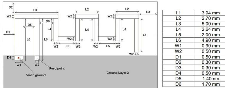
Figure 5.5: Antenna AN043 design
