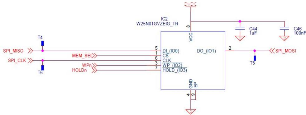
Figure 5.58: W25N01GV schematics
