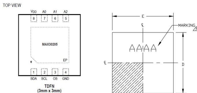
Figure 5.63: MAX30205 pinout and dimensions
