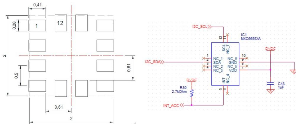
Figure 5.8: MEMSIC MXC6655XA - 3-axis accelerometer
