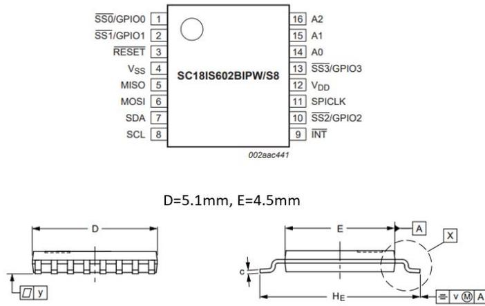
Figure 5.60: SC18IS602BIPW/S8HP - i2c to spi pinout aand package
