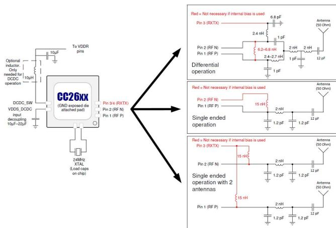
Figure 5.4: Antenna schematic options
