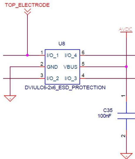
Figure 5.22: DVIULC6-2M6 schematic
