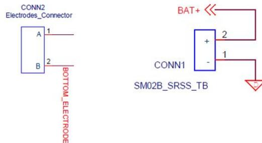
Figure 5.39: Connectors SM02B-SRSS-TB schematic
