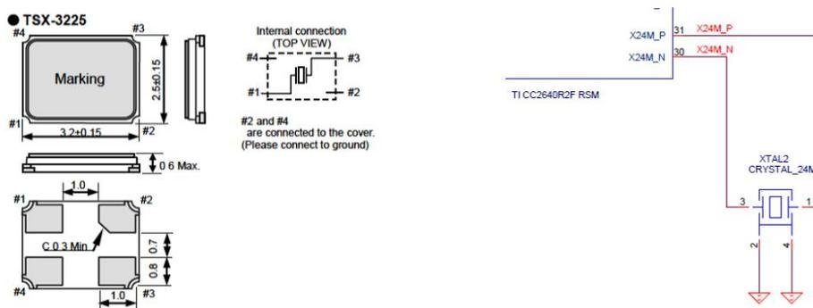
Figure 5.52: TSX-3225 24.0000MF20X-B schematics
