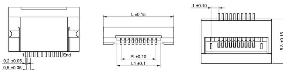
Figure 5.41: Würth Elektronik 687108149022 dimensions
