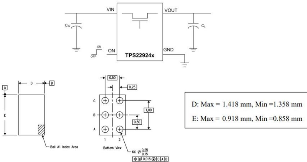
Figure 5.30: Mosfet TPS22924BYZZR pinout and dimensions
