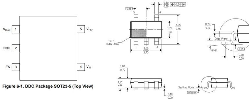
Figure 6-1. DDC Package SOT23-5 (Top View)
