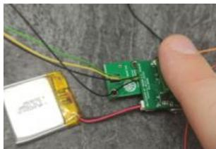
Figure 11.7: Finger temperature measurement mode
