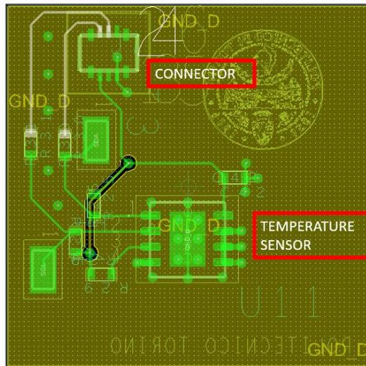
Figure 9.4: PulsECG: temperature board
