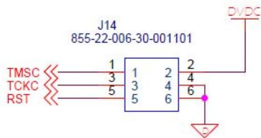
Figure 5.70: Mill-Max 855-22-006-30-001101 schematics
