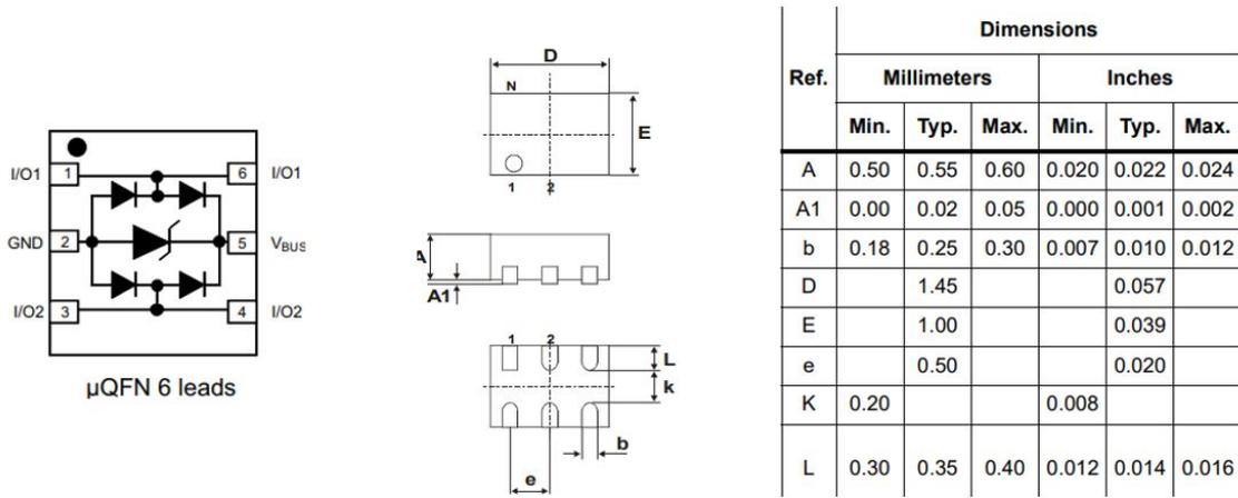
Figure 5.21: DVIULC6-2M6 pinout and package
