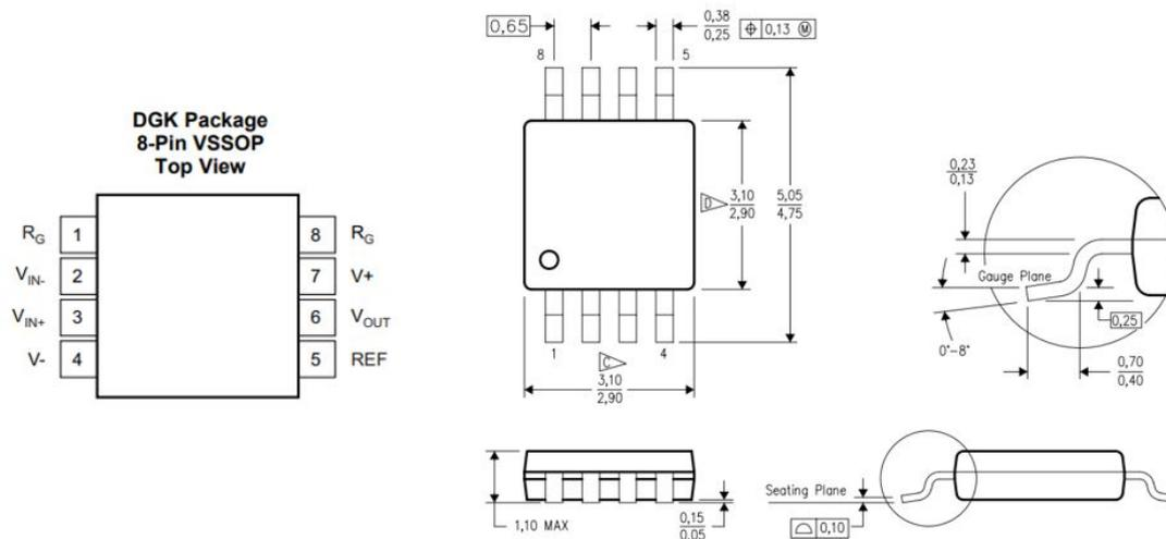
Figure 5.23: INA333 pinout and package
