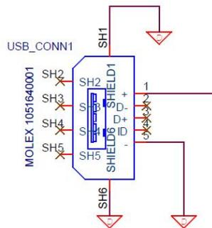
Figure 5.35: Micro-USB schematic
