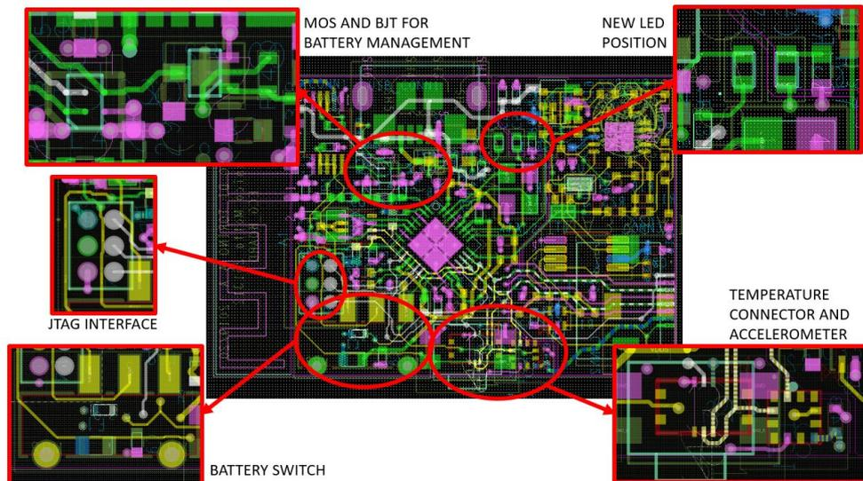
Figure 9.2: ECG board focus
