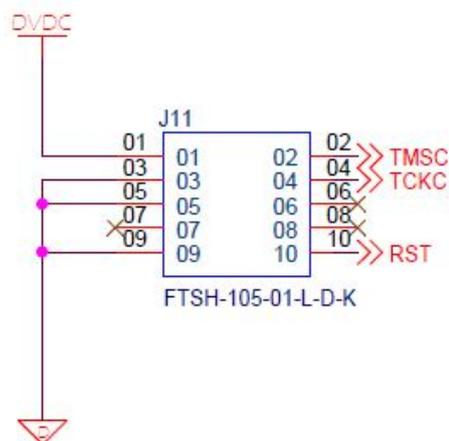
Figure 5.68: JTAG Connector FTSH-105-01-L-D-K schematics
