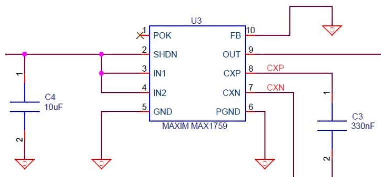
Figure 5.20: MAX1759 schematic
