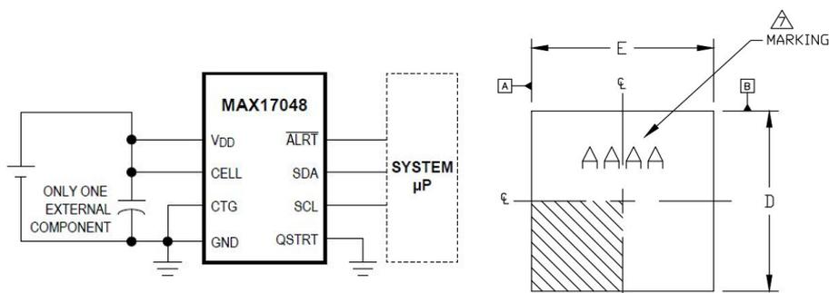
Figure 5.13: Battery gauge module MAX17048: pinout and package
