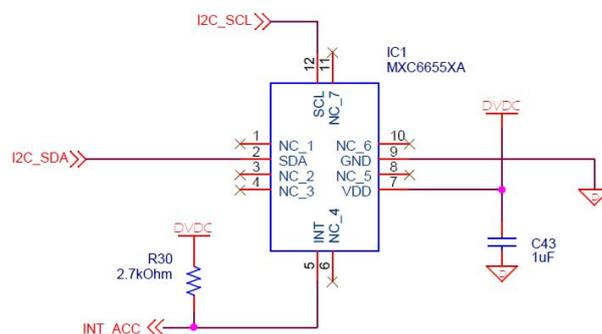
Figure 5.9: Accelerometer schematic
