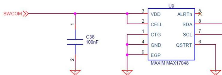
Figure 5.14: MAX17048 schematic
