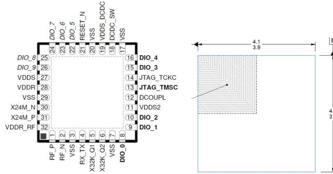
Figure 5.2: CC2640R2F: pinout and dimensions
