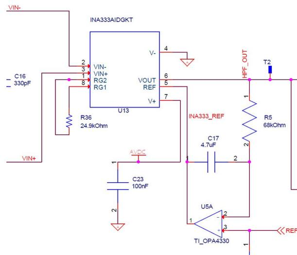
Figure 5.24: INA333 schematic
