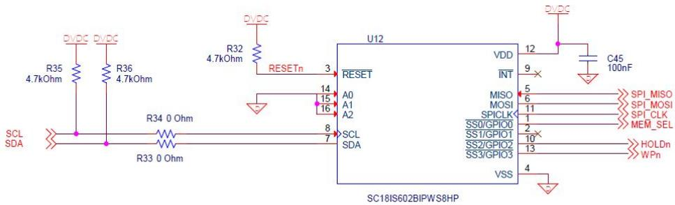
Figure 5.61: SC18IS602BIPW schematics
