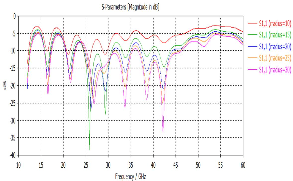
Fig. 3.8(b): Vivaldi Antenna Bending Analysis
