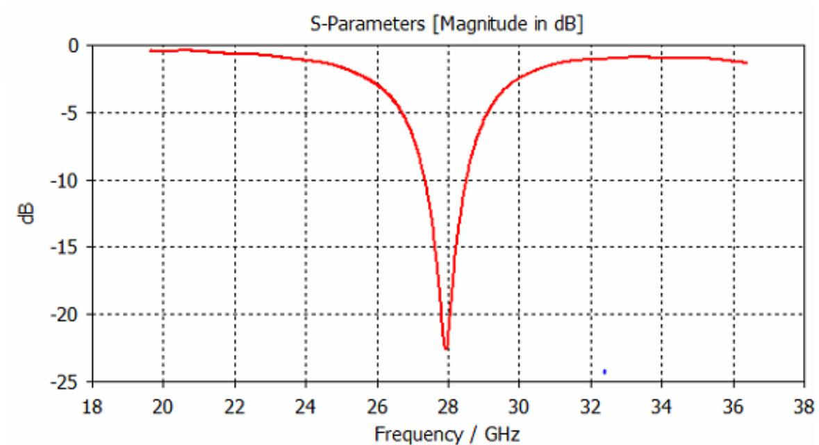
*Fig. 4.2: substrate Rogers 5880 and patch material copper*
