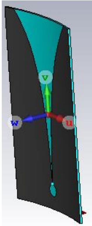
Fig. 3.8(a): Vivaldi Antenna Bending Analysis
