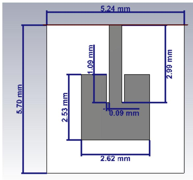
Fig. 3.1: Patch Antenna Dimensions
