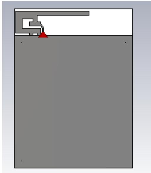
*Fig. 3.2: PIFA Antenna Design*
