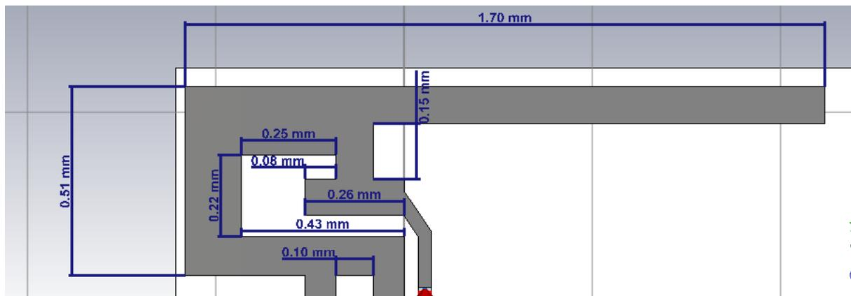
*Fig. 3.3(a): PIFA Antenna Dimensions*
