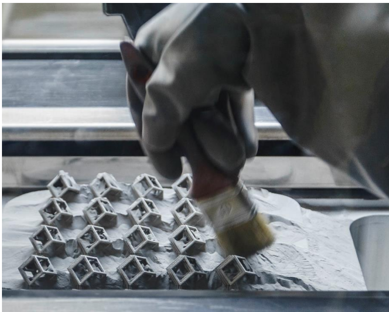
Figure 21, operator during the removing of untreated powder [37]
