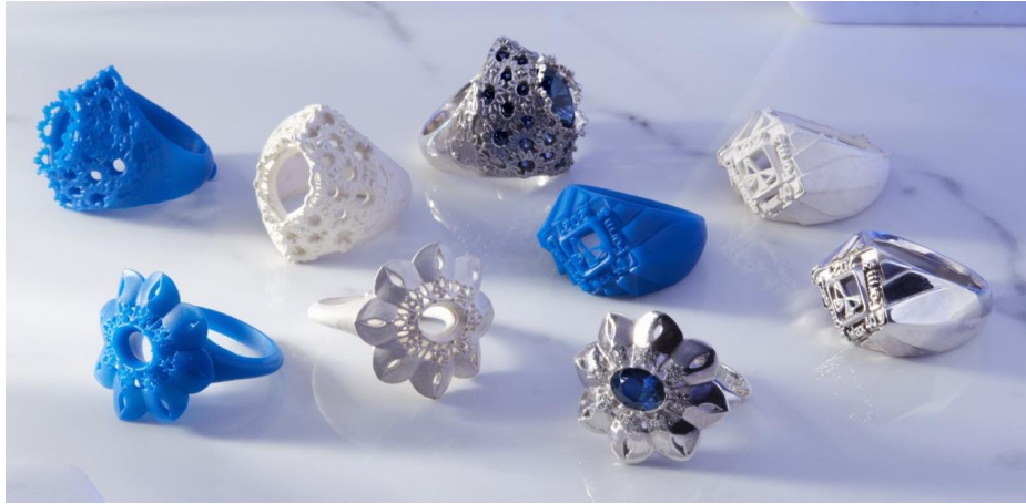
Figure 6, 3d printed and relative casting pieces [12]
