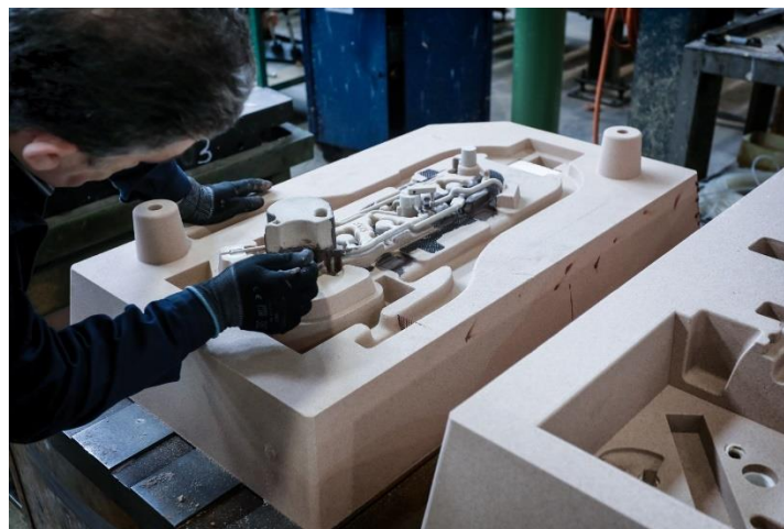
Figure 1, mold with sand cores 3d printed [3]
