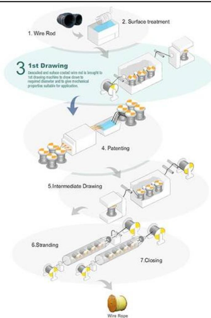
Fig.25 Manufacturing of wire rope
