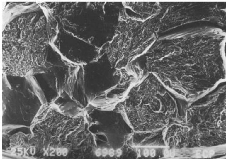
Fig.71: Intergranular fracture of steel
