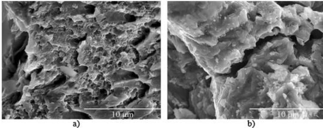
Fig.74: a) void coalescence and secondary cracking; b) Intergranular failure
