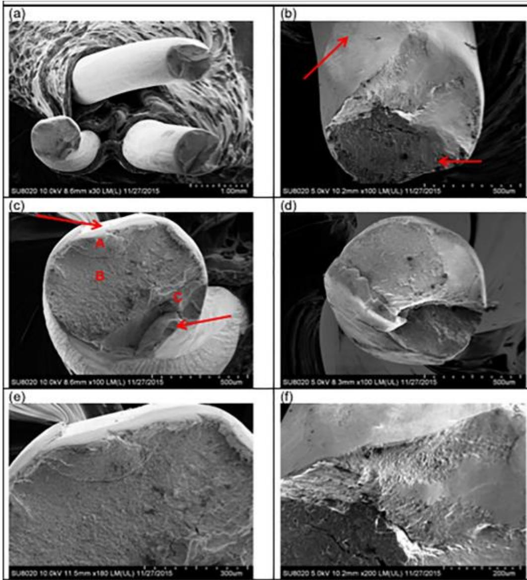
Fig.77: (a, c, e) Representative wires of the core, (b, d, f) representative wires of the external part [135]
