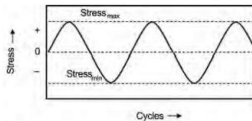
Fig.2: Fatigue (Cyclic Loading)
