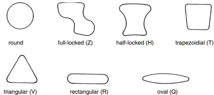
Fig.6: Wire cross-sections for wire ropes [4]
