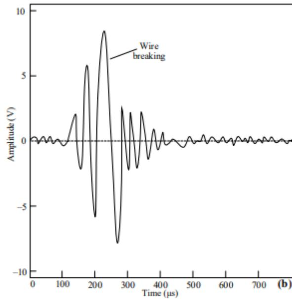
Fig.37: Sketch map of wire breaking signal
