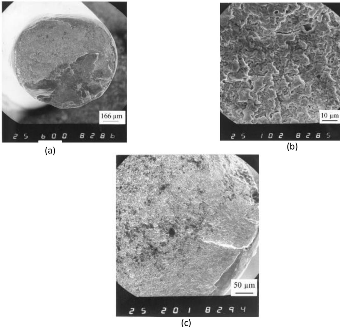
Fig.78: Fatigue Fracture with a) damaged edges b) micro-cracks c) Initial Crack [137]
