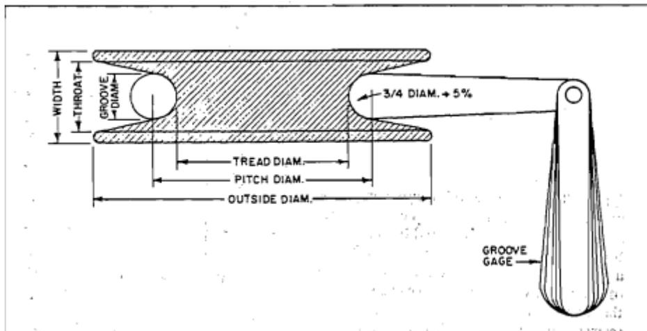
Fig.66: Schematic of sheave dimensions and gage usage
