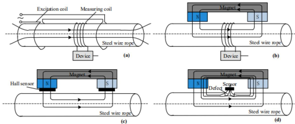
Fig.35: Electromagnetic non-destructive detection principle of steel wire rope.
