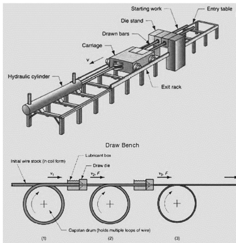
Fig.31: Continuous Wire Drawing Draw Bench
