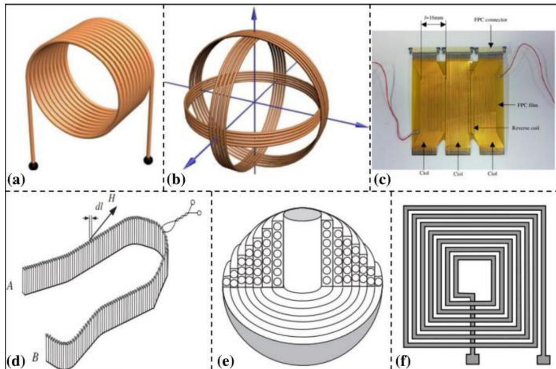
Fig.45: different types of inductive coil sensors. a)The spiral coil, b) three-axis perpendicular coil, c) flexible printed coil, d) Rogowski coil, e) spherical coil, f) Planar thin film coil
