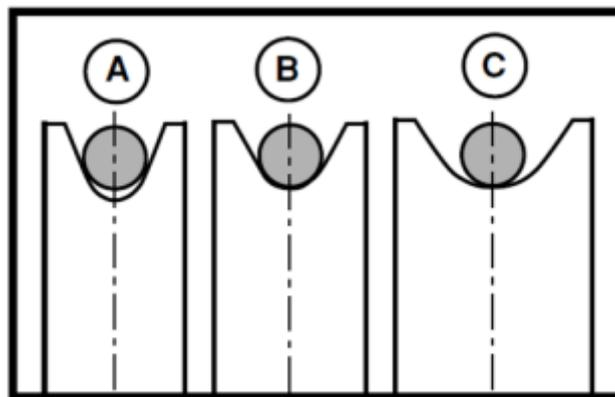
Fig.58: Conditions of small, optimum and large sheave diameter
