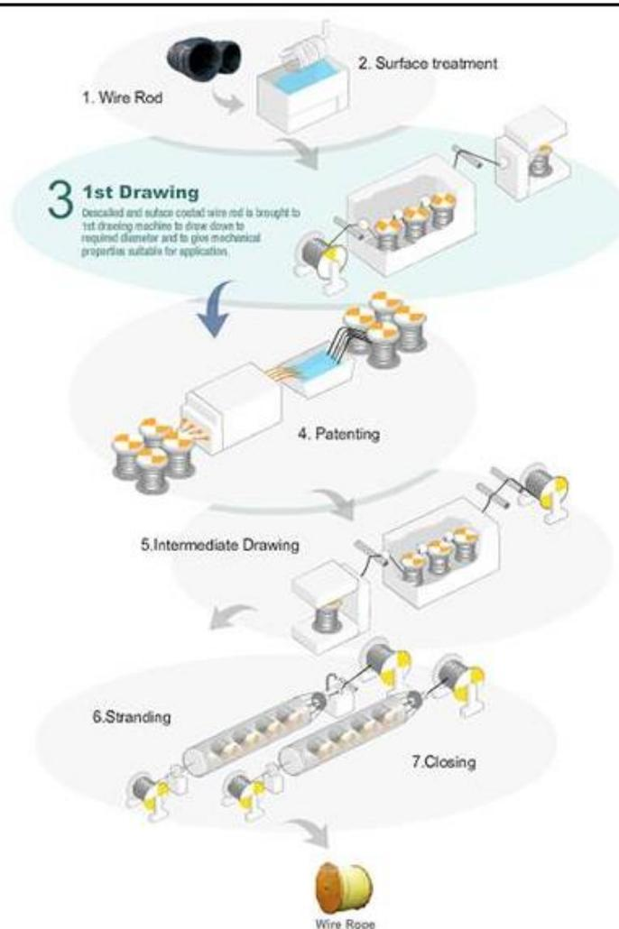
Fig.25 Manufacturing of wire rope
