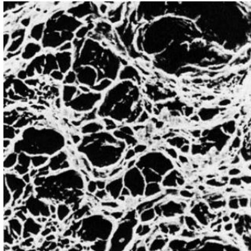
Fig.69: Dimpled ductile fracture [124]
