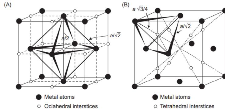
Fig.20: Interstitial voids in fcc structure [11]
