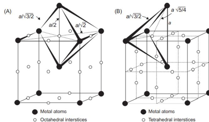
Fig.21: Unit cell structure of ferrite [11]
