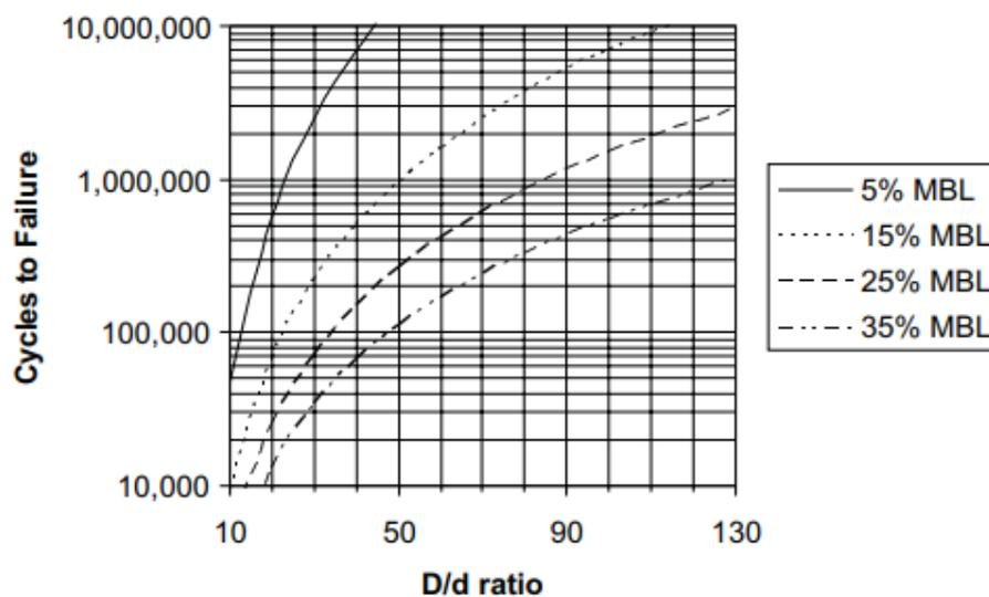
Fig.33: The mean number of cycles to failure in bending-over sheaves fatigue as predicted by Feyrer (1995) as a function of  $D/d$  Ratio in terms of minimum breaking load [23]
