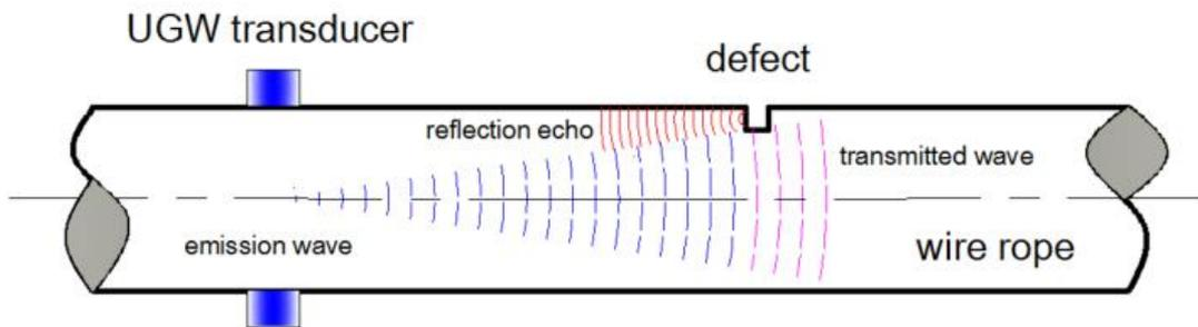
Fig.41: Working Principle of UGWTM
