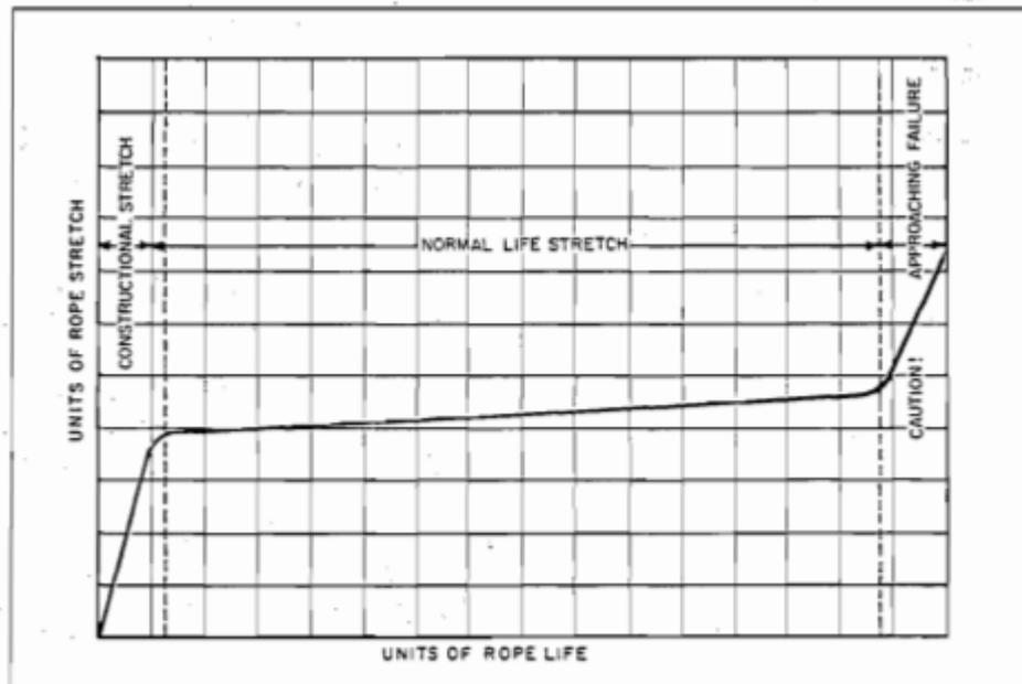
Fig.67: Stretch Curve of wire rope
