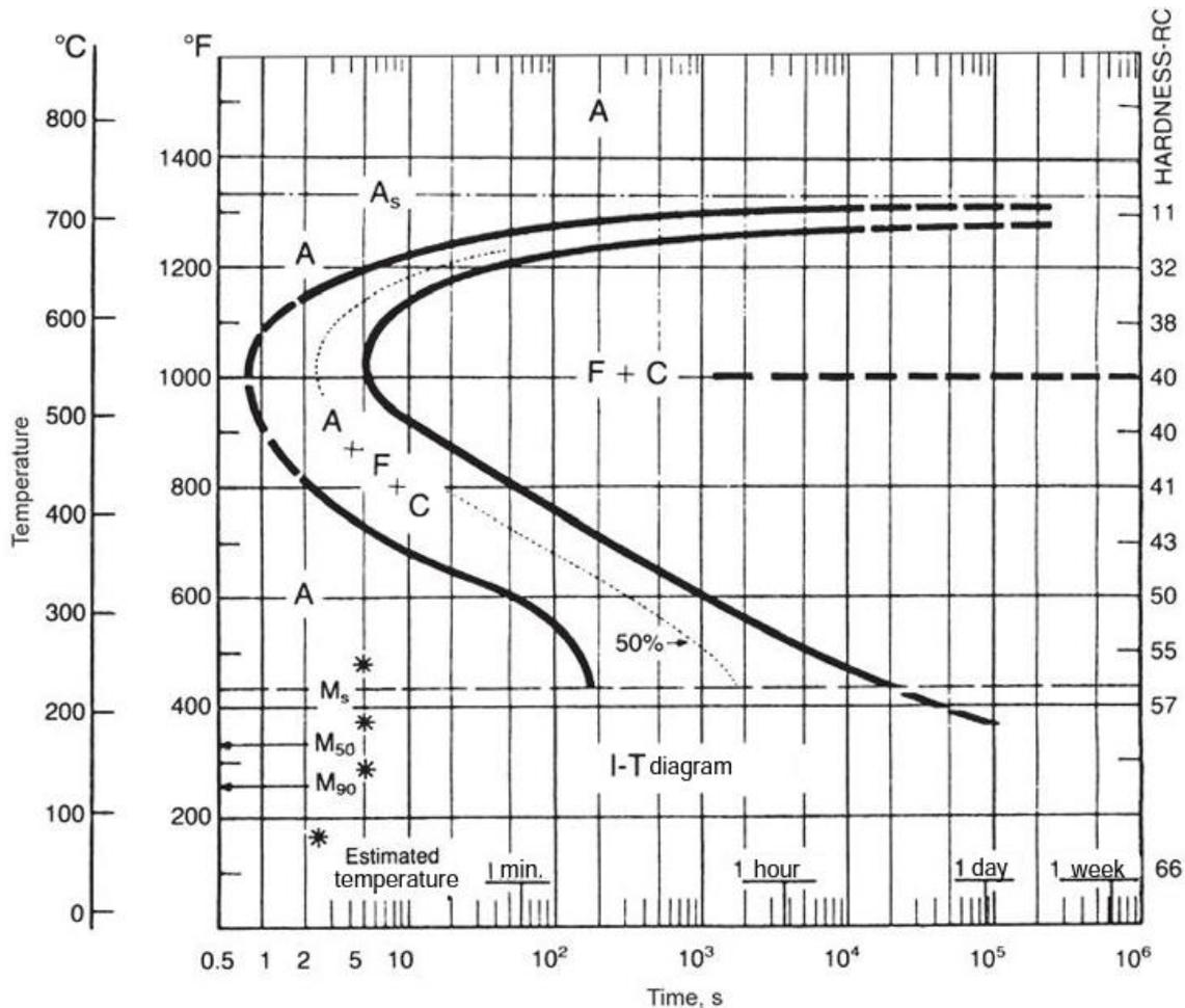
Fig.24: Isothermal Transformation of 1080 steel [10]
