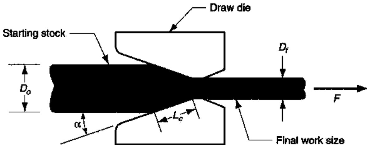
Fig.30: Drawing Process
