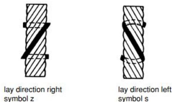
Fig.8: Lay direction of wires [4]
