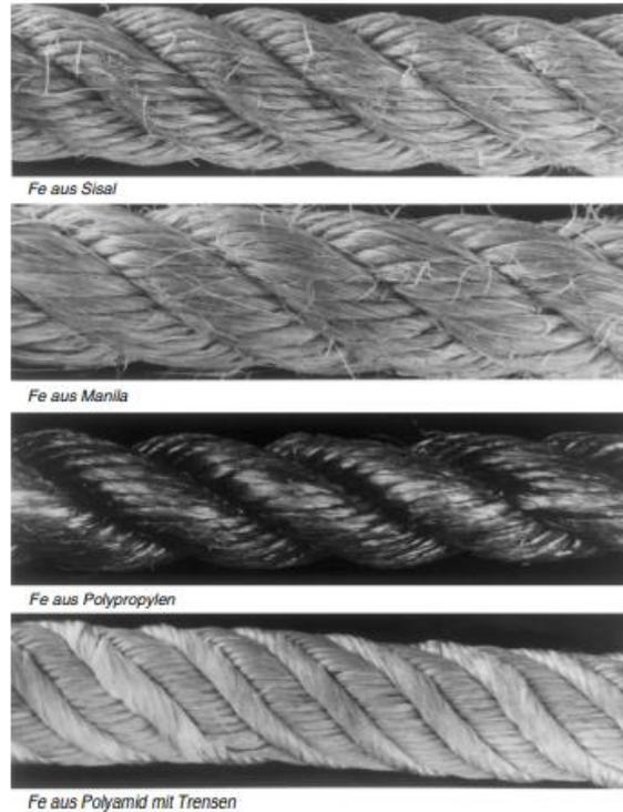
Fig.14: Fibre cores [5]
