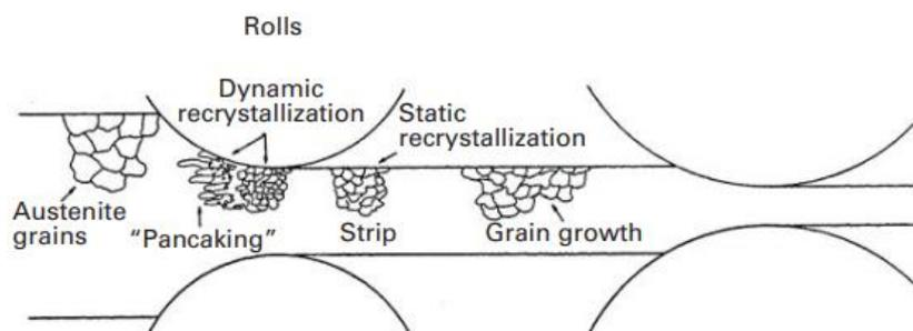
Fig.29: Changes in Microstructure during Hot Rolling [19]
