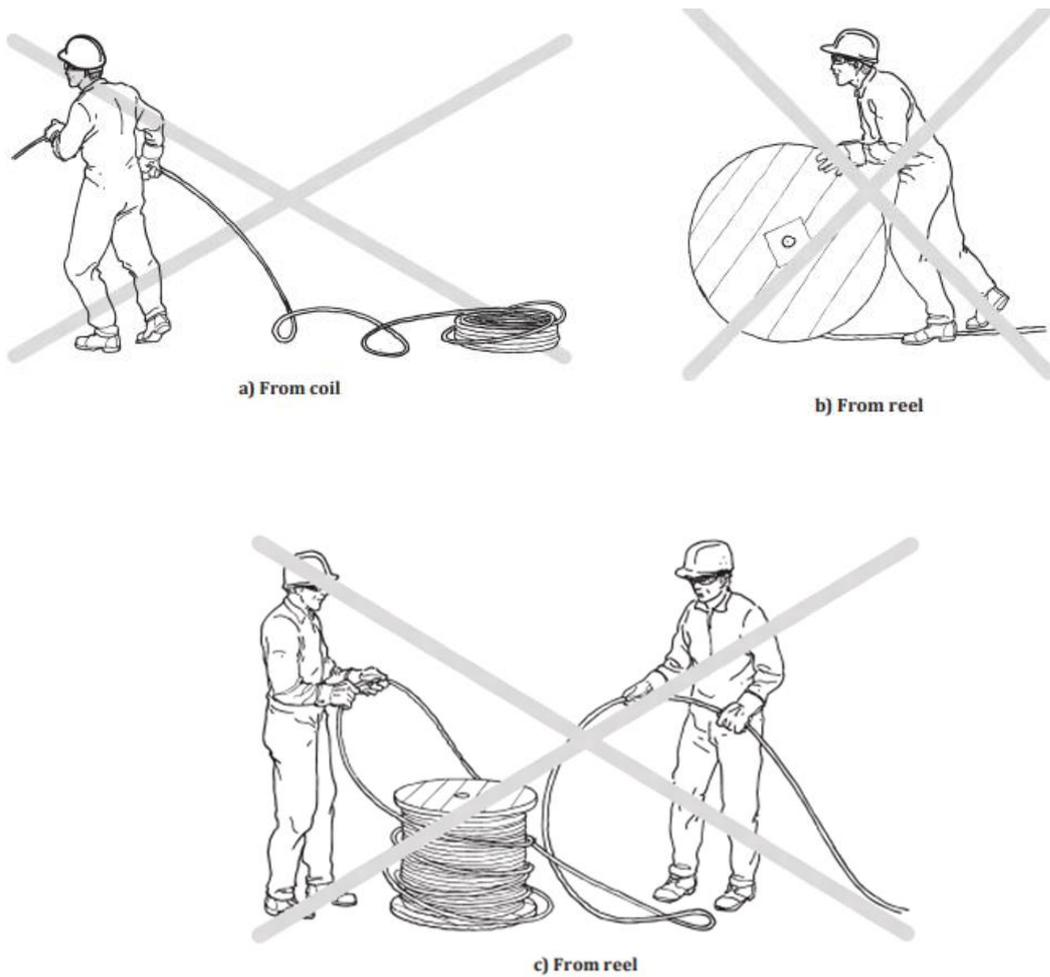
Fig.52: Incorrect Procedures of uncoiling a wire rope
