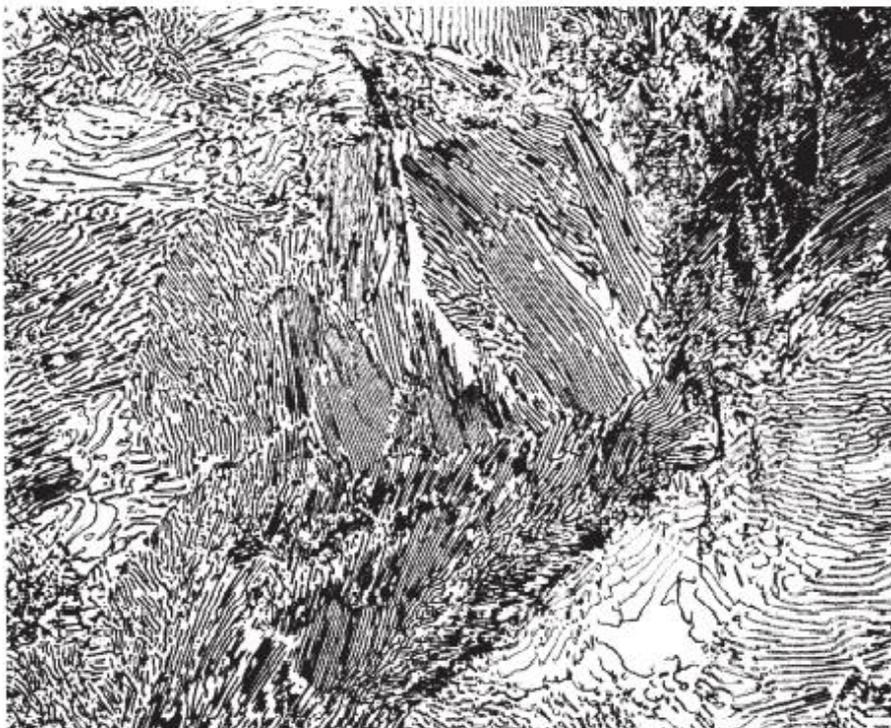
Fig.23: Pearlite in a furnace-cooled Fe-0.75C alloy [10]
