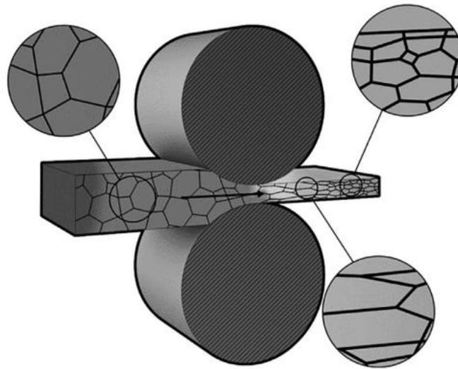
Fig.28: Hot Rolling Process Illustration [17]
