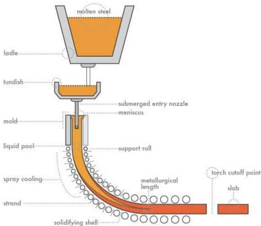
Fig.26: Continuous Casting [16]
