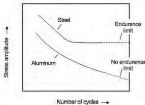
Fig.3: Schematic of materials with endurance limit and without endurance limit
