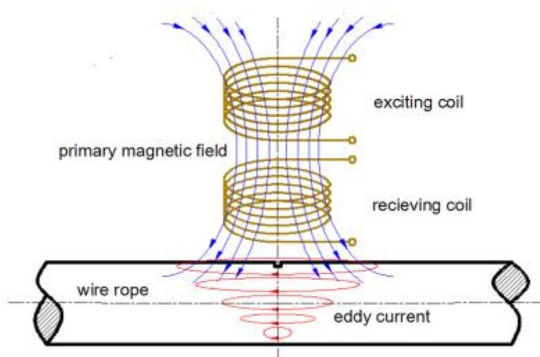
Fig.36: Principle of Eddy Current testing
