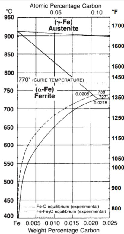
Fig.19: Ferrite phase field and decrease of carbon solubility with decreasing temperature [9]
