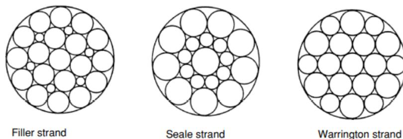
Fig.10: Parallel Lay Strands with two wires [4]
