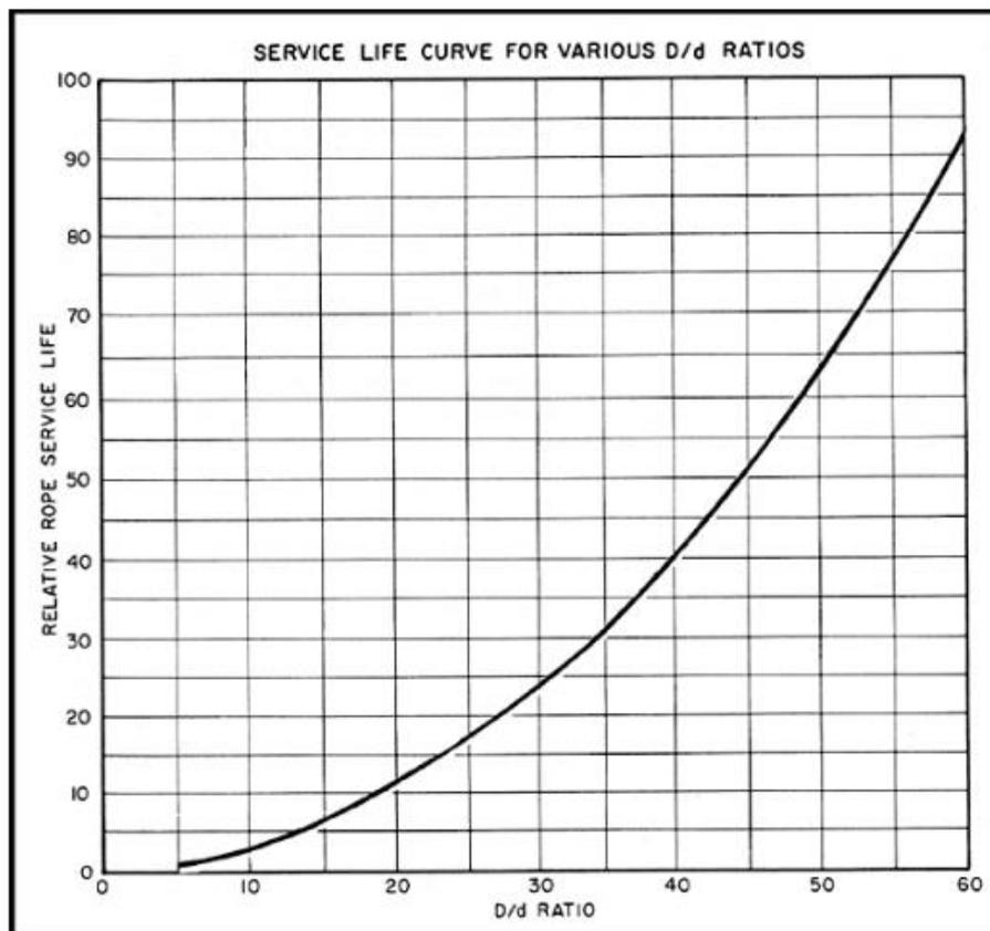
Fig.59: Service life curve of Wire Rope
