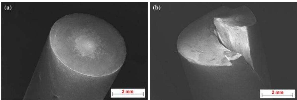
Fig.82: Torsion fracture of steel wire a) Flat fracture; b) Cleavage fracture [143]
