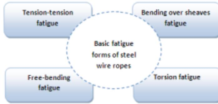
Fig.32: Fatigue forms of steel wires
