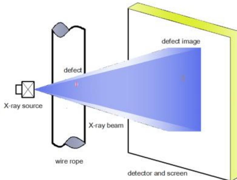
Fig.42: Schematic of X-Ray testing method of wire rope
