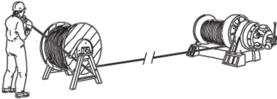
Fig.53: Transfer of rope from bottom of reel to bottom of drum
