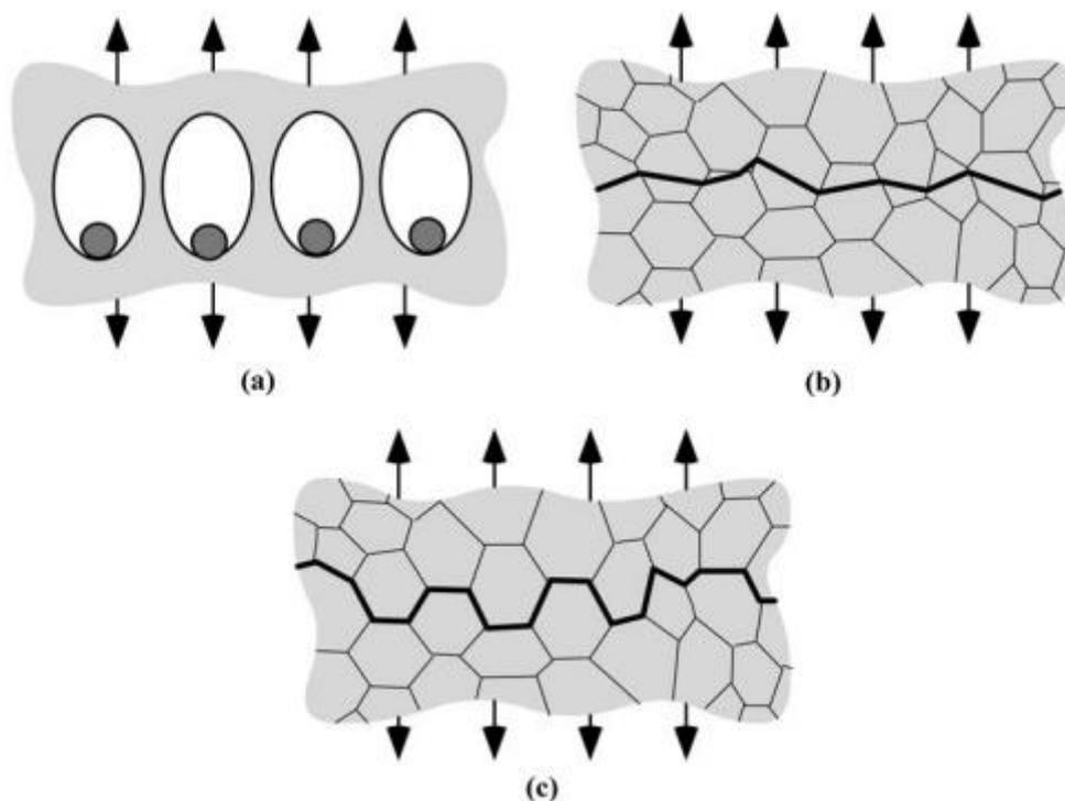
Fig.68: Mechanisms of Fracture a) Ductile, b) Cleavage, c) Intergranular [123]
