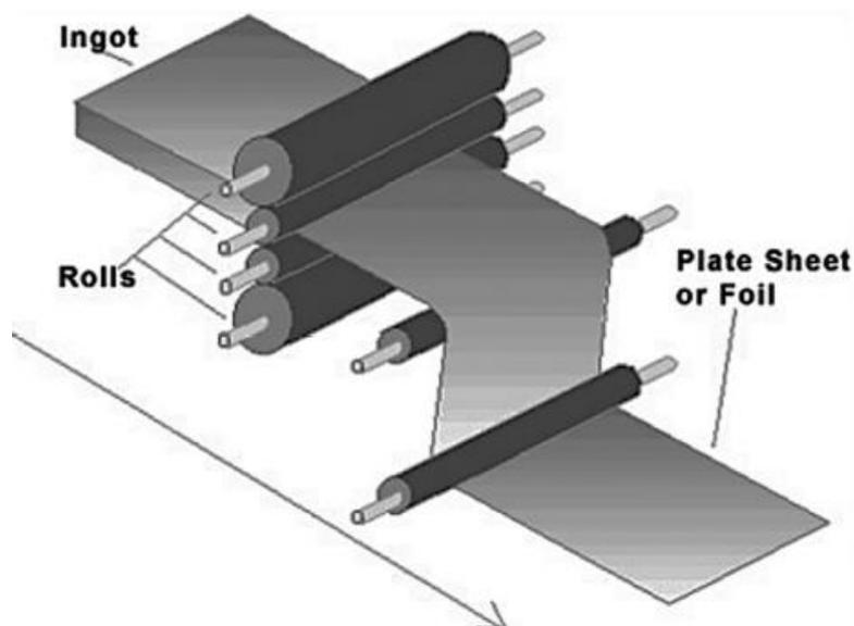
Fig.27: Rolling operation explained [17]
