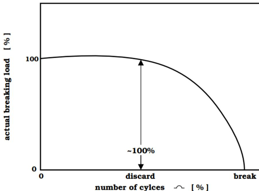
Fig.47: Relation between breaking load and number of cycles
