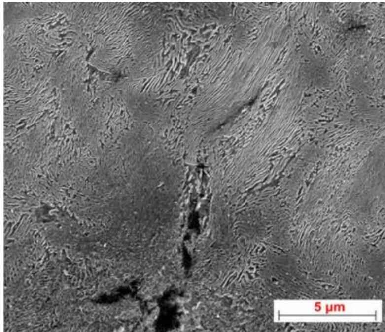
Fig.83: SEM microfractography showing torsion cracks in pearlite [143]
