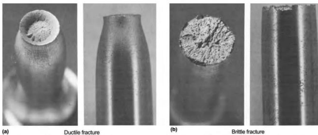
Fig.4: Ductile and Brittle Fracture
