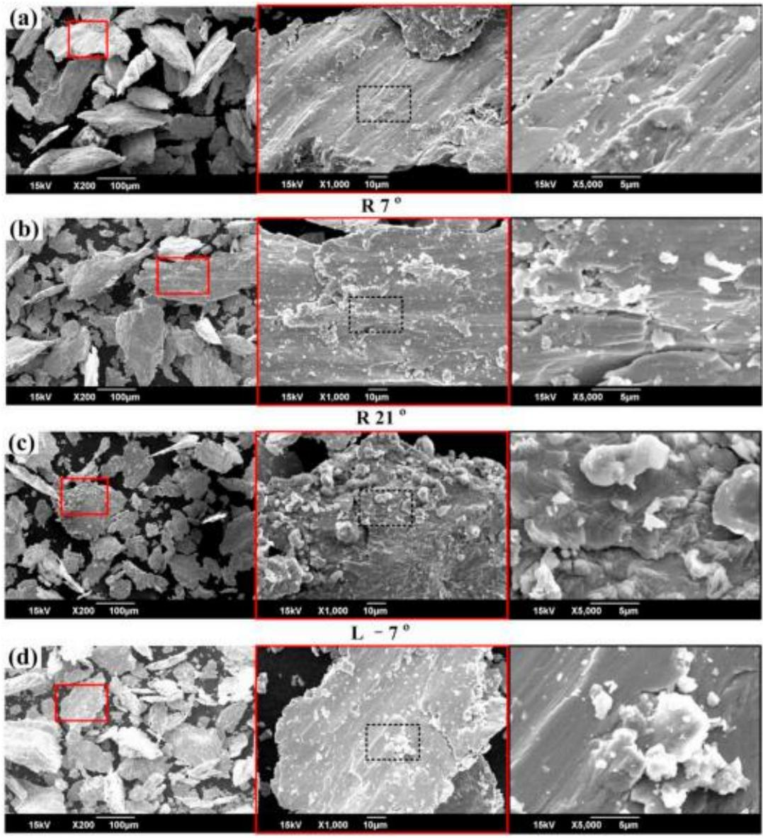
Fig.75: SEM micrograph of debris a)and b) right cross contact; c) and d) left cross contact [133]
