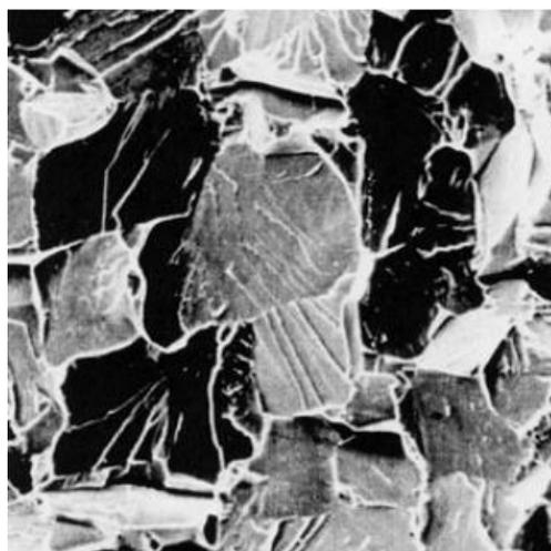
Fig.70: Cleavage fracture specimen of a carbon steel [124]
