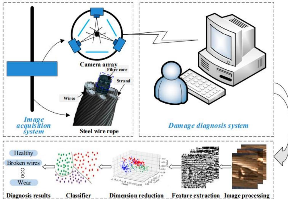
Fig.43: Principle of optical detection method
