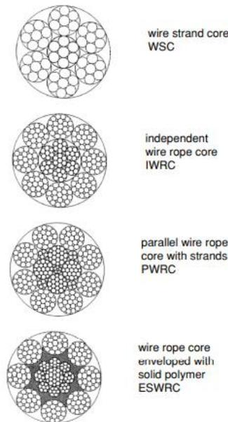
Fig.15: Steel Cores in wire ropes [4]
