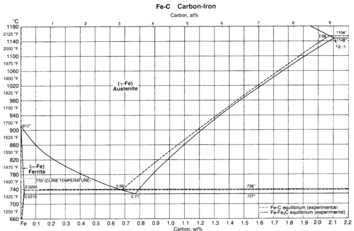
Fig.22: Portion of Fe-C diagram pertinent to transformation [9]
