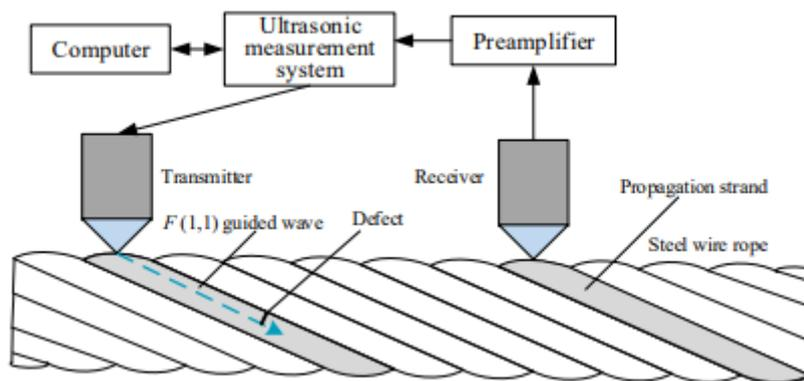
Fig.40: Schematic of Ultrasonic Guided Wave Testing Method
