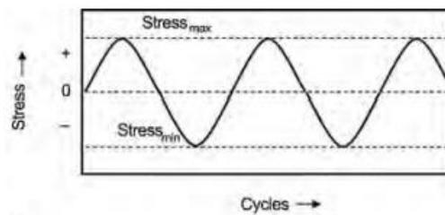
Fig.2: Fatigue (Cyclic Loading)
