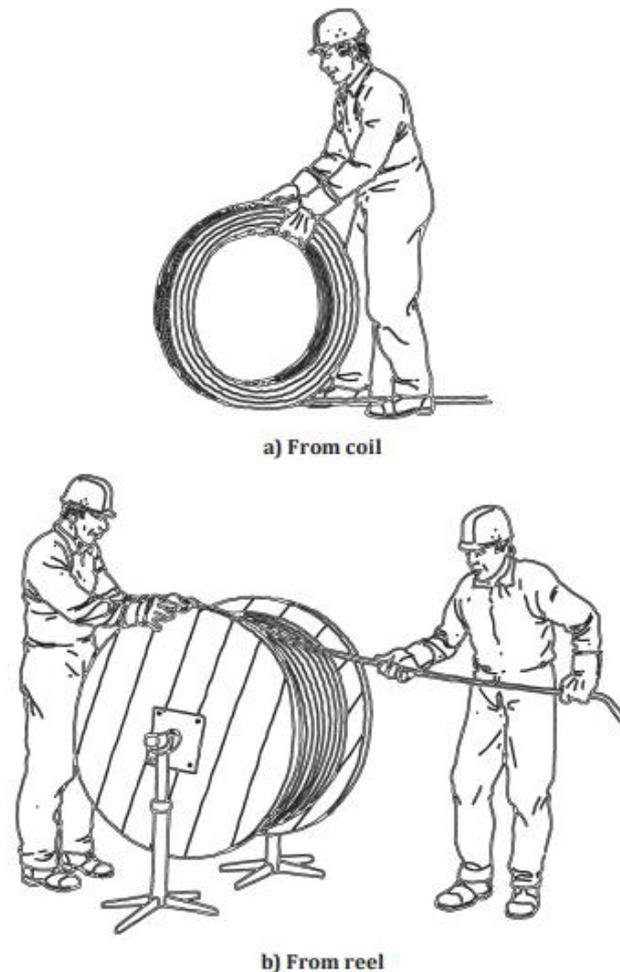
Fig.51: Correct procedures for uncoiling wire rope
