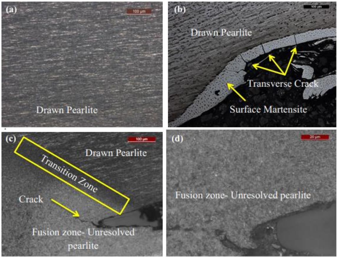
Fig.81: Optical microfractography of damaged ropes a) away from damaged zone; b) abraded region; c) and d) fusion zones at different magnifications [142]
