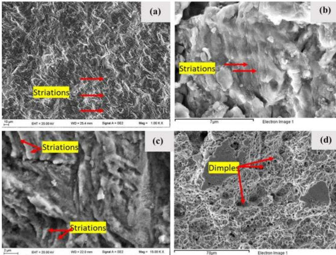
Fig.80: SEM microfractography a), b), c) showing fatigue striations; d) cup and cone fracture showing dimples
