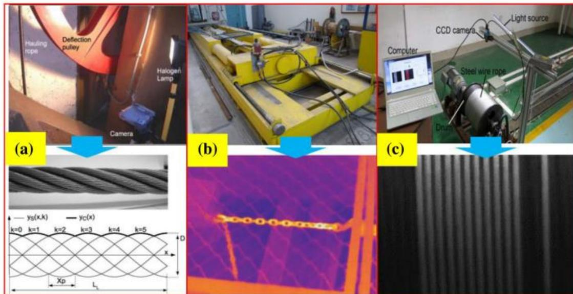
Fig.44: Other testing methods: a) Laser light method b) Thermal Imaging c) Machine vision
