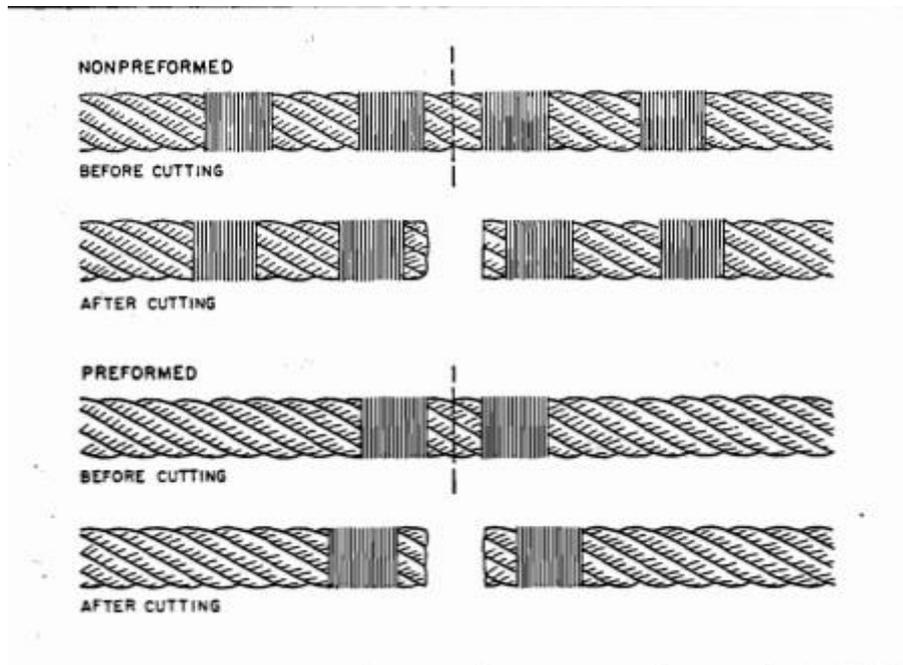
Fig.55: Seizings for non-preformed and preformed wires
