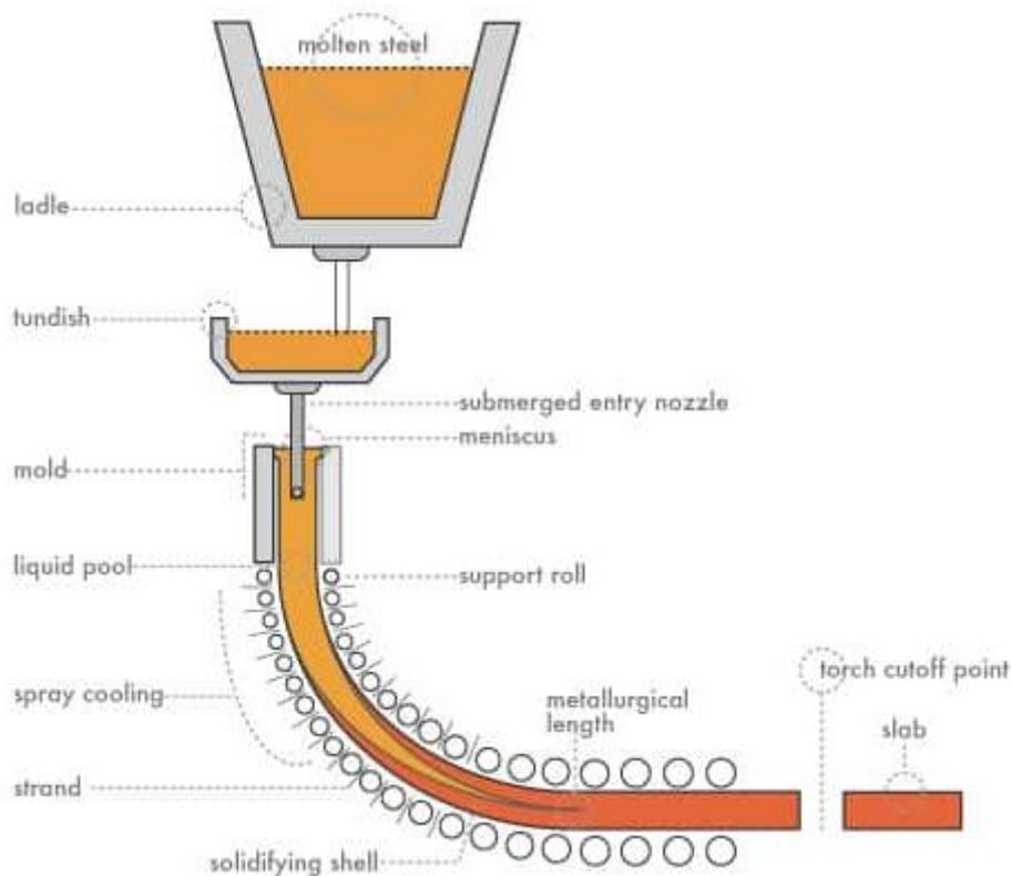
Fig.26: Continuous Casting [16]
