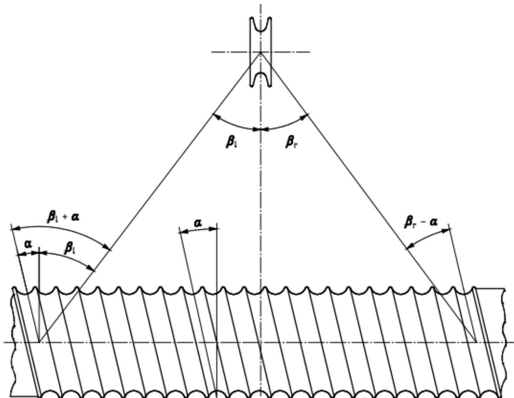
Fig.61: Fleet and Groove Angles
