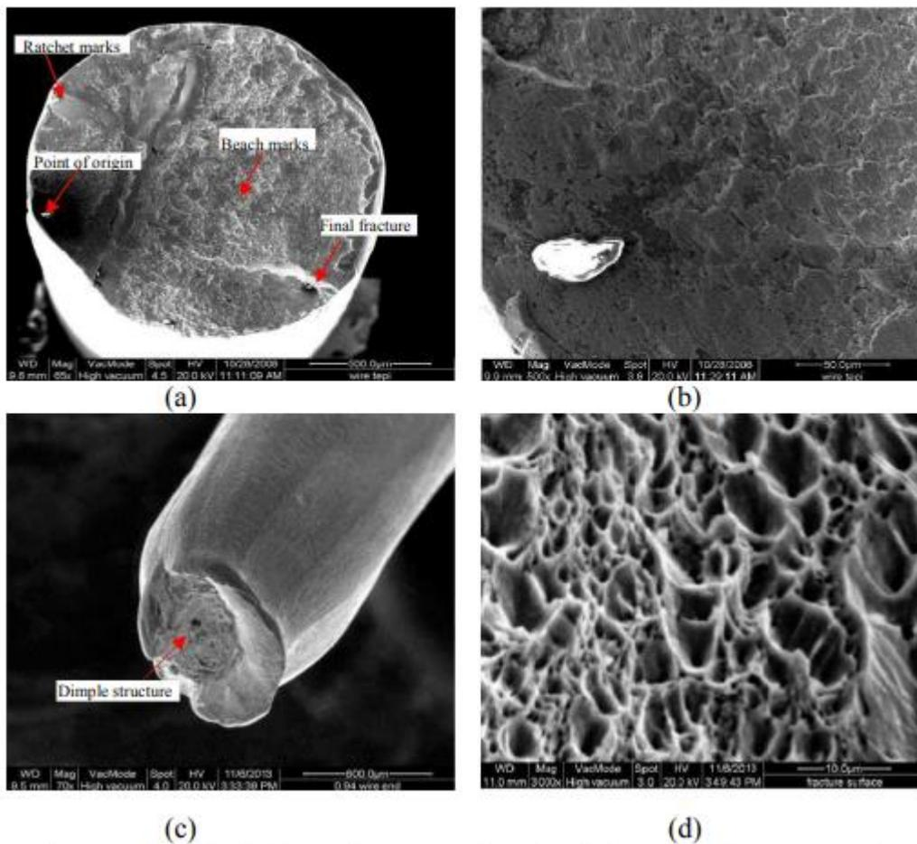
Fig.76: a) fatigue fracture surface; b) fatigue striations; c) cup of cup and cone fracture; d) zoomed in image showing dimple morphology [134]
