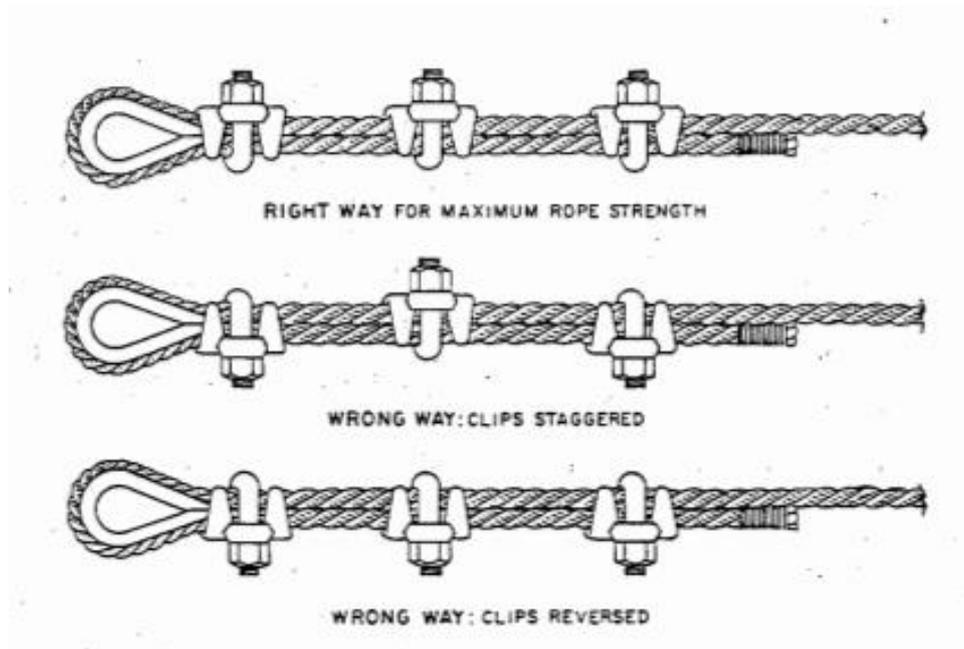
Fig.56: Right and wrong ways of attaching the U-bolt clips
