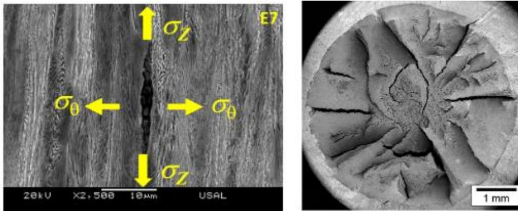
Fig.72: Anisotropic fracture behaviour in cold drawn pearlitic steel
