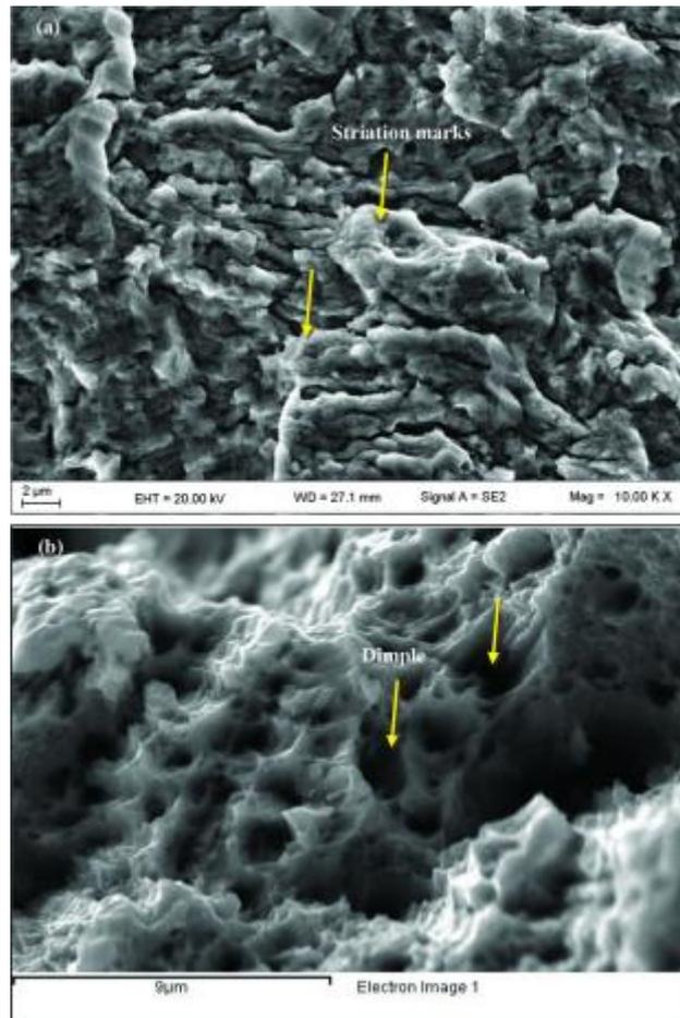
Fig.79: a) striation indicating fatigue; b) dimples indicating ductile fracture [141]
