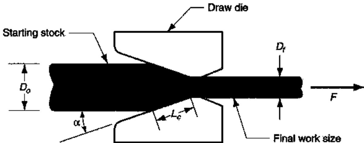
Fig.30: Drawing Process
