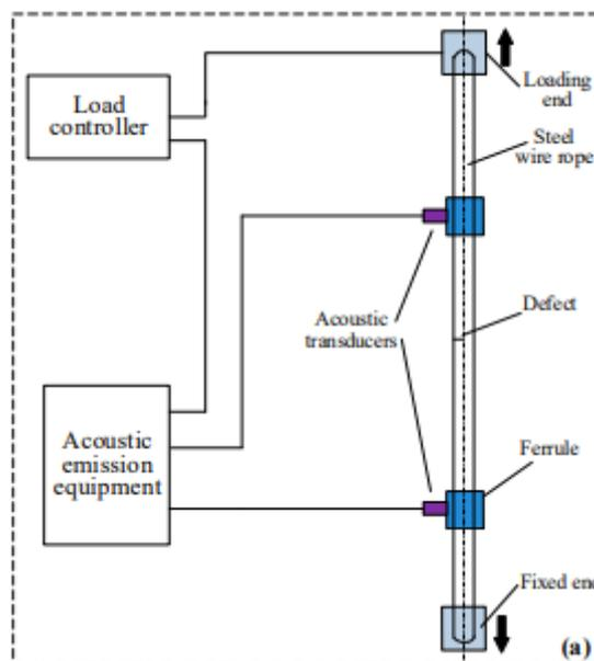
Fig.38: Schematic diagram of detection system
