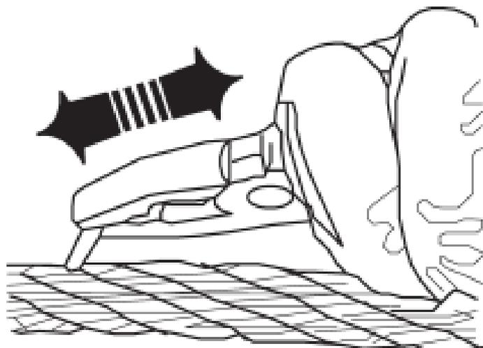
Fig.63: Removal of broken wire
