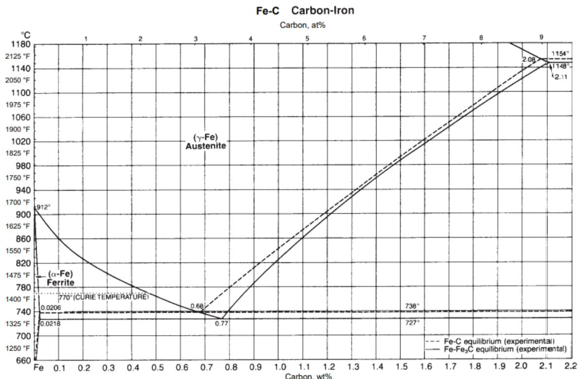
Fig.22: Portion of Fe-C diagram pertinent to transformation [9]
