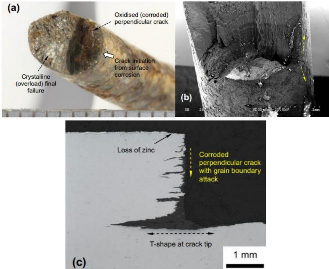
Fig.73: Broken wire removed from the cable a) corrode crack initiation b) change in crack propagation direction c) grain boundary attack [130]
