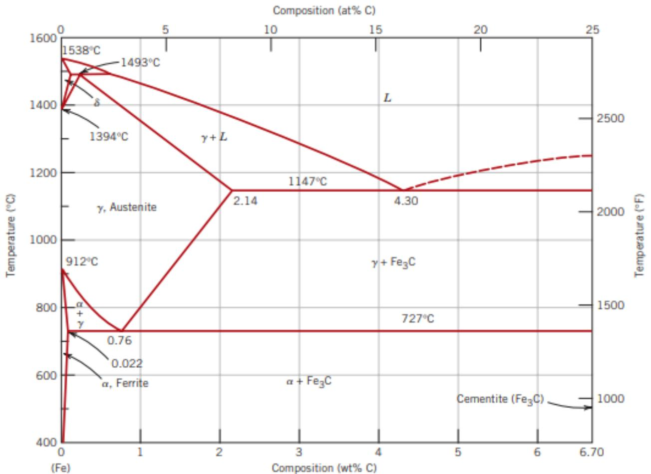
Fig.18: Iron-Iron Carbide phase diagram [9]
