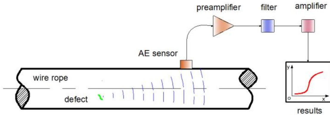
Fig.39: Principle of Acoustic Emission Testing Method
