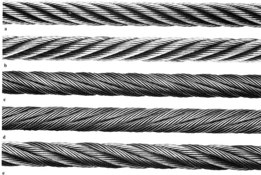
Fig.16: A comparison of typical wire rope lays: a) right regular lay, b) left regular lay, c) right lang lay, d) left lang lay, e) right alternate lay [2].
