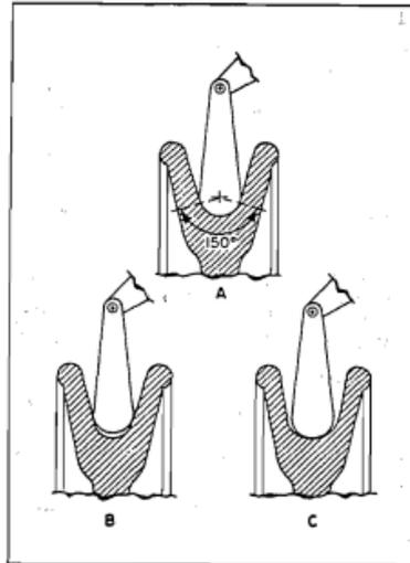
Fig.65: Schematic of gage groove contact, A is the optimum condition, B is small sheave diameter and C is large sheave diameter
