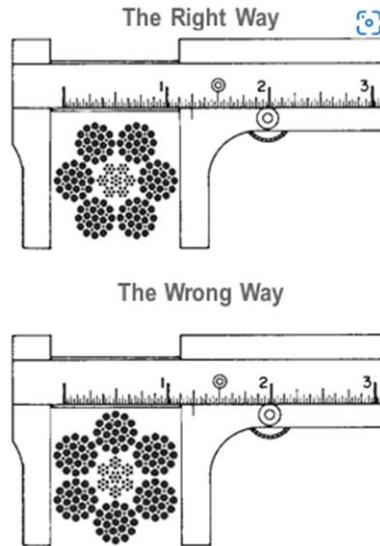
Fig.48: Measurement of wire rope diameter
