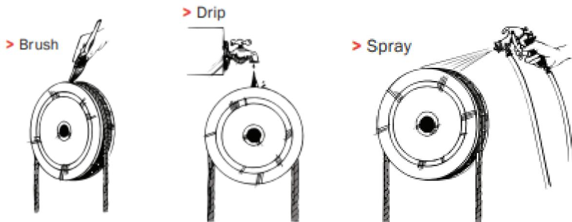
Fig.62: Different types of lubrication
