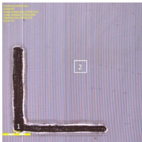
Figure 2.18: L-shaped mark in the reference surface (master).
