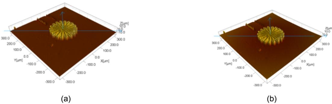
Figure 4.6: Global plane correction of ASG raw measurement: a) Levelling b) Bow removal.
