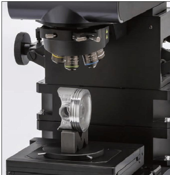
Figure 2.4: Olympus LEXT laser scanning confocal microscope (LSC).
